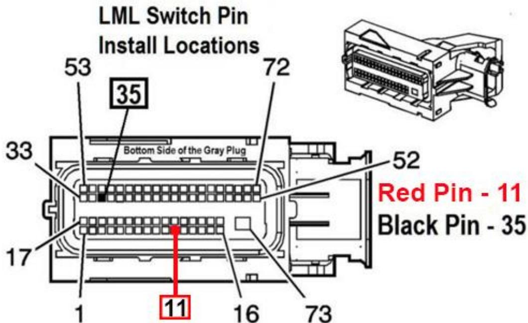
Note: Some Tuner could use different Pin locations, confirm to ensure proper pin locations and Installation
