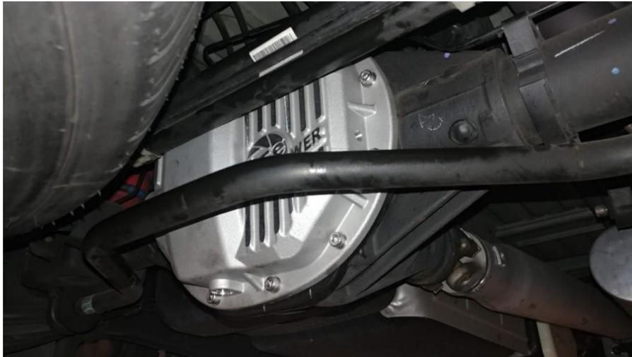
13. Hold the OEM gasket and the supplied aFe differential cover into position, aligning the screw holes. Install two (2) of the supplied M8x1.25x25 socket head screws and flat washers into separate sides of the cover to hold it in place.
