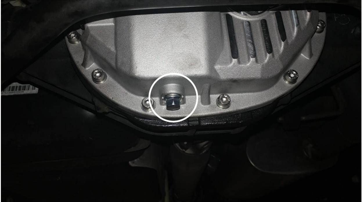
18. Install the supplied M12x1.25 drain plug and crush washer into the bottom of the cover.
