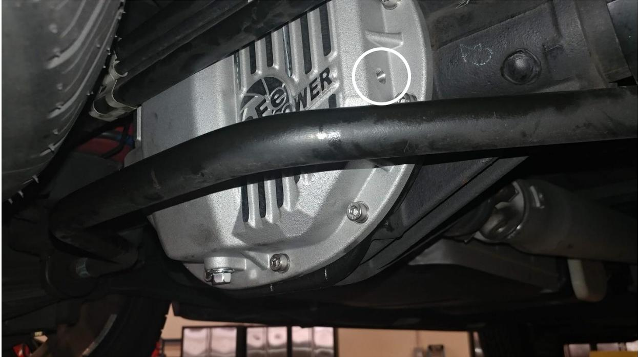
20. Fill the aFe differential cover using new gear oil. Fill until gear oil runs out of the 1/8" NPT port on the side of the cover (about 3 1/2 quarts).
