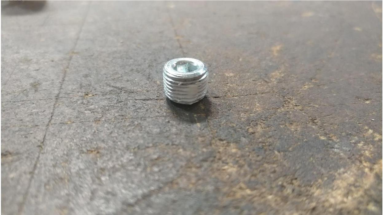
19. Apply Teflon pipe sealant to the threads of the supplied 1/8" NPT plug.
