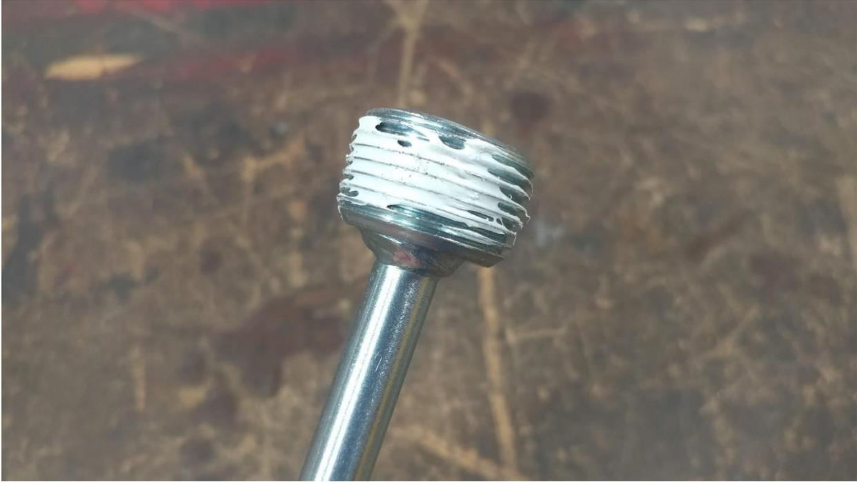
21. Apply Teflon pipe sealant to the threads of the supplied 1/2" NPT magnetic 3" deep reach plug.
