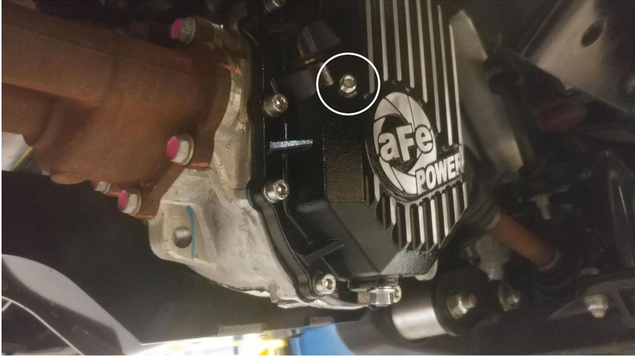
20. Install the 1/8" NPT plug into the side of the cover.
