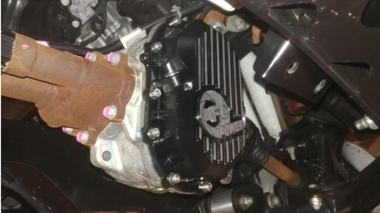
14. Hold the OEM gasket and aFe differential cover into position, aligning the screw holes. Install one (1) of the supplied M8x1.25x25 socket head screws and flat washers at the top of the cover to hold it in place.
