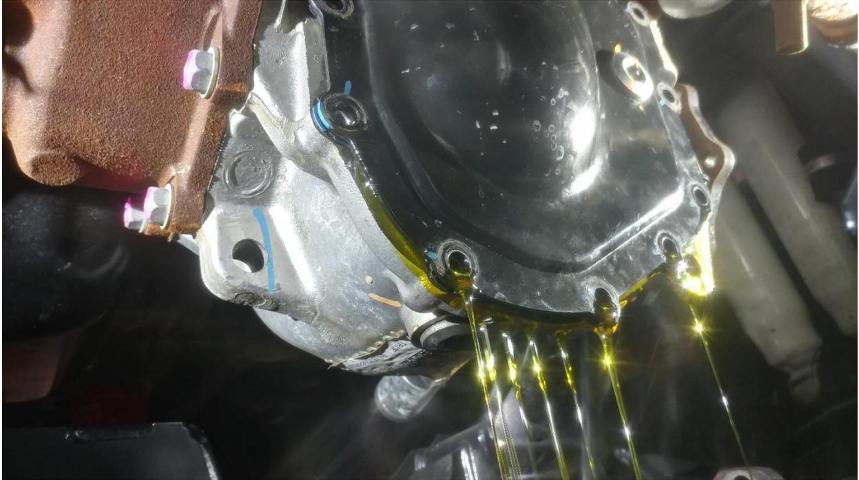
7. Allow all of the gear oil to drain from the differential.
