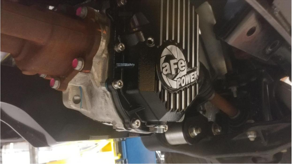
17. Install the supplied M12x1.25 drain plug and crush washer into the bottom of the cover.
