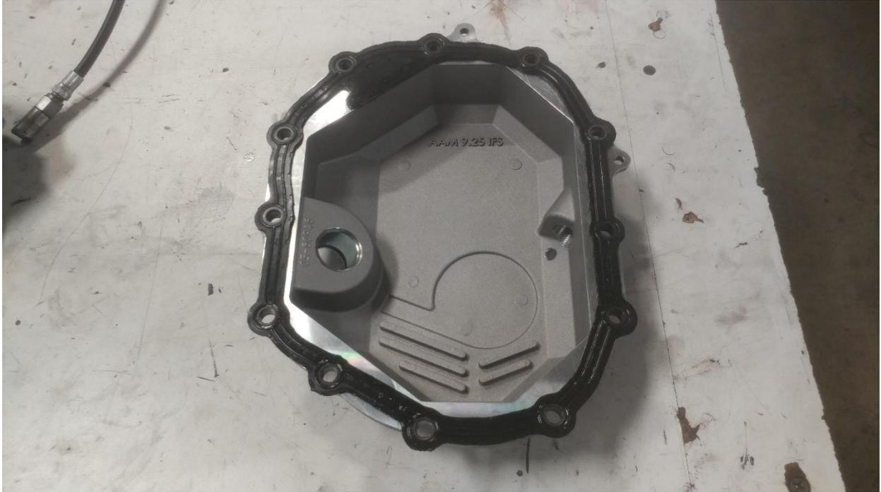
13. Align the OEM gasket and supplied aFe differential cover into position using the correct orientation shown above.
