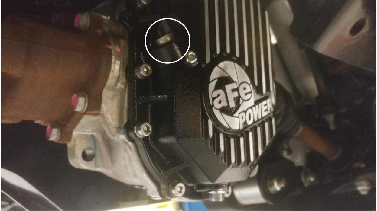
22. Install the 1/2" NPT magnetic 3" deep reach plug into the fill port.
