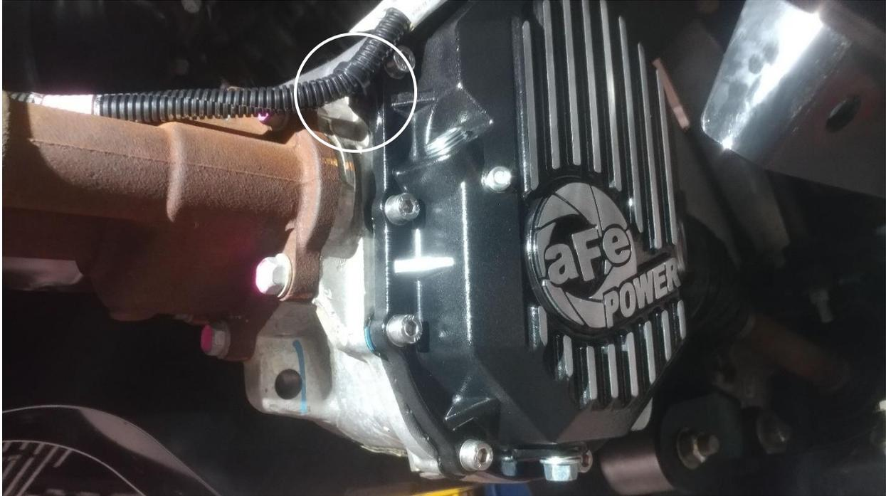
23.Reconnect the four wheel drive actuator wire to the left side and top of the aFe differential cover.
