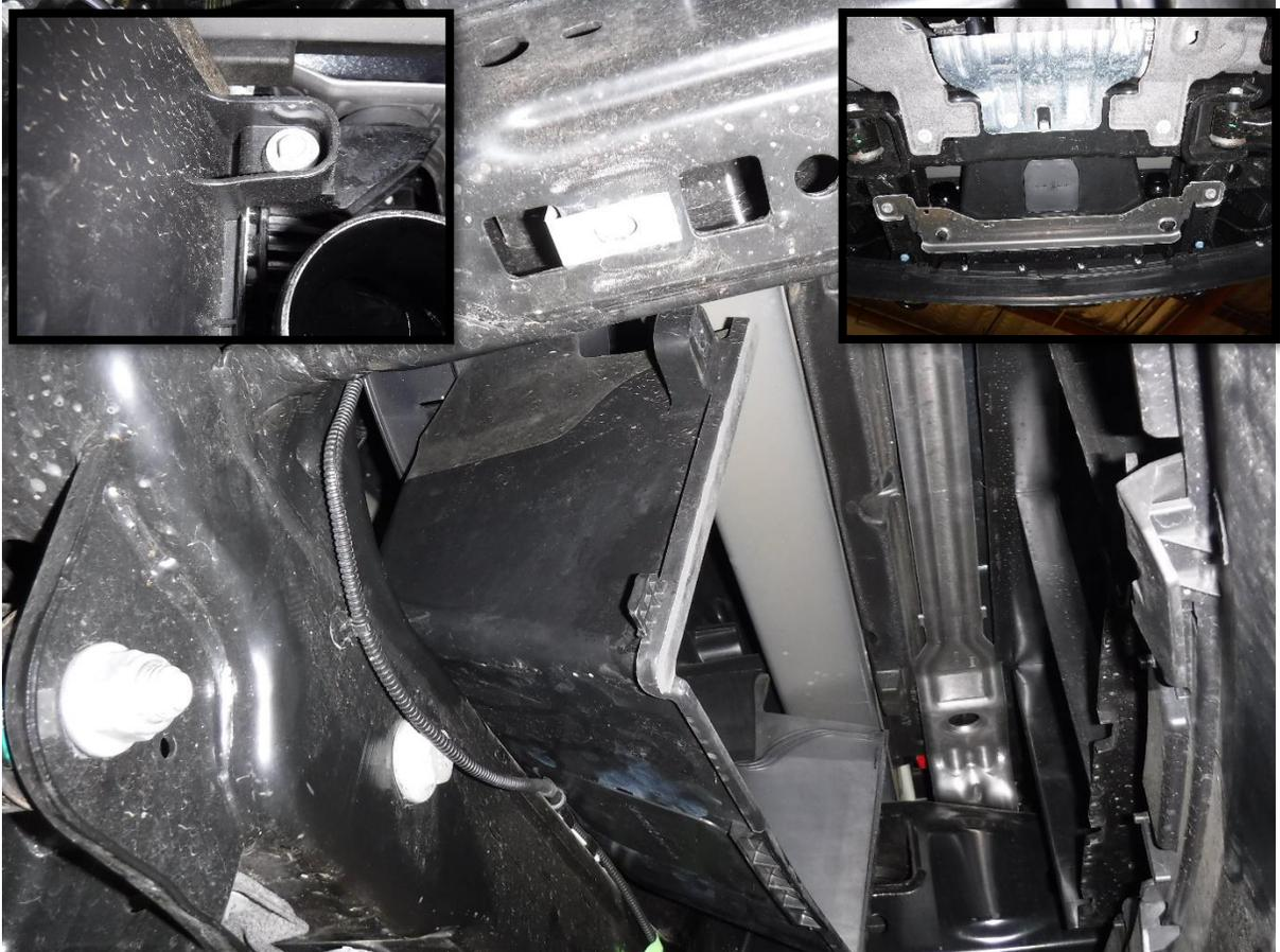
17. Remove the bolt securing the lower fan shroud to the intercooler located above the hot side intercooler tube connection.
