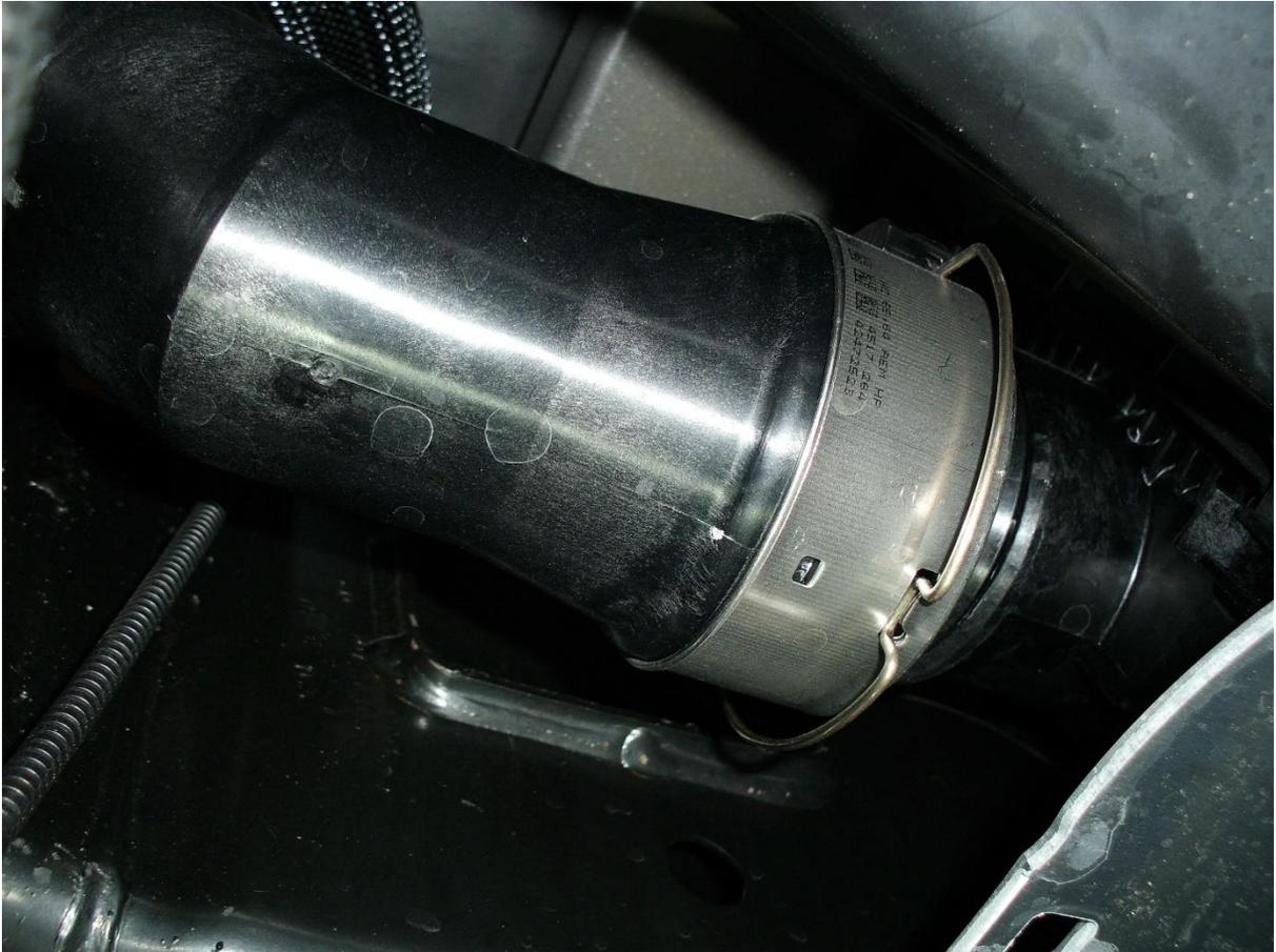
15. Underneath the vehicle on the driver side, disconnect the quick connect adapter connecting the cold side intercooler tube to the intercooler.
