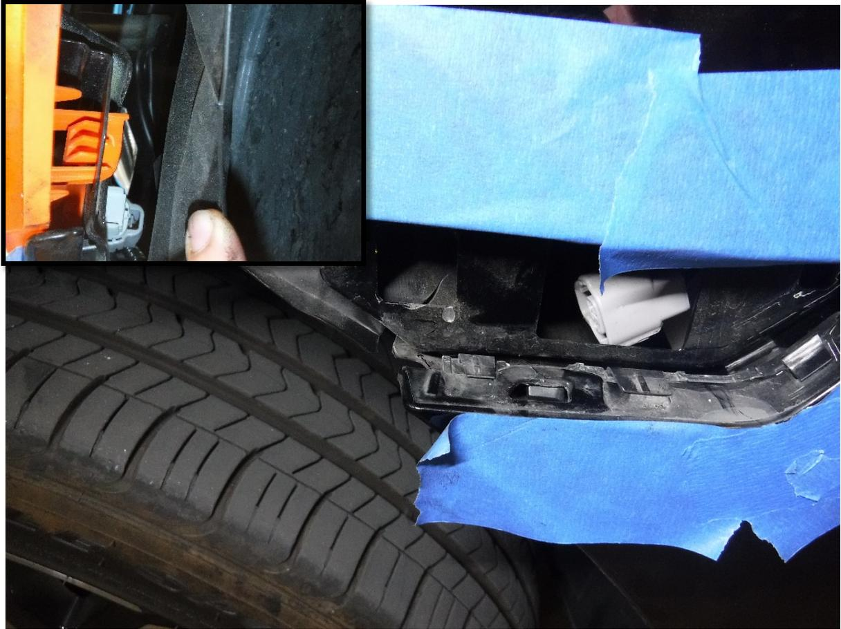
6. Depress the retaining clip behind the fender liner to remove the side marker lights on each side then disconnect the connectors.
