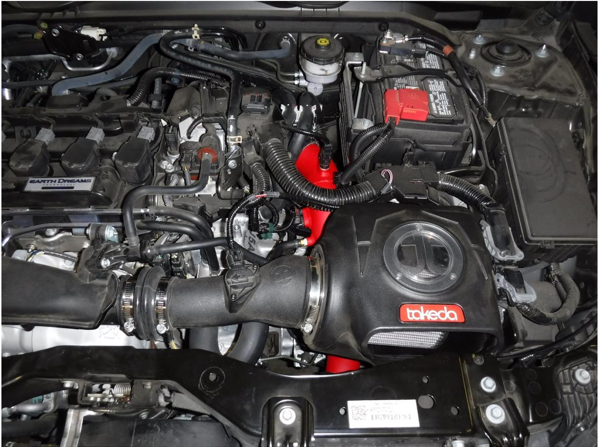
63. Reinstall the intake system back into the vehicle.
