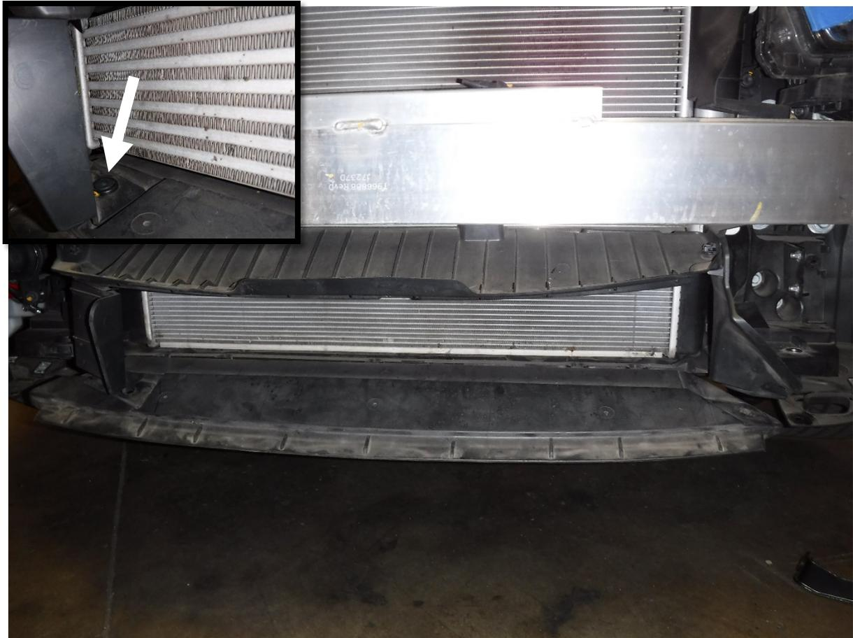
33. Remove the clip securing the air deflector on the passenger's side of the vehicle.
