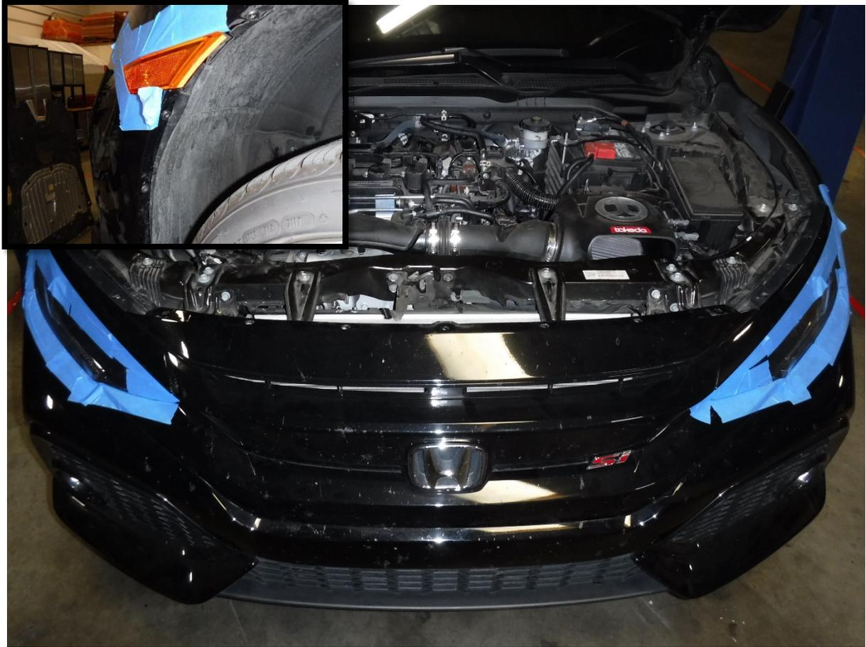
4. Remove plastic radiator cover, using a panel popper or flat blade screwdriver.
