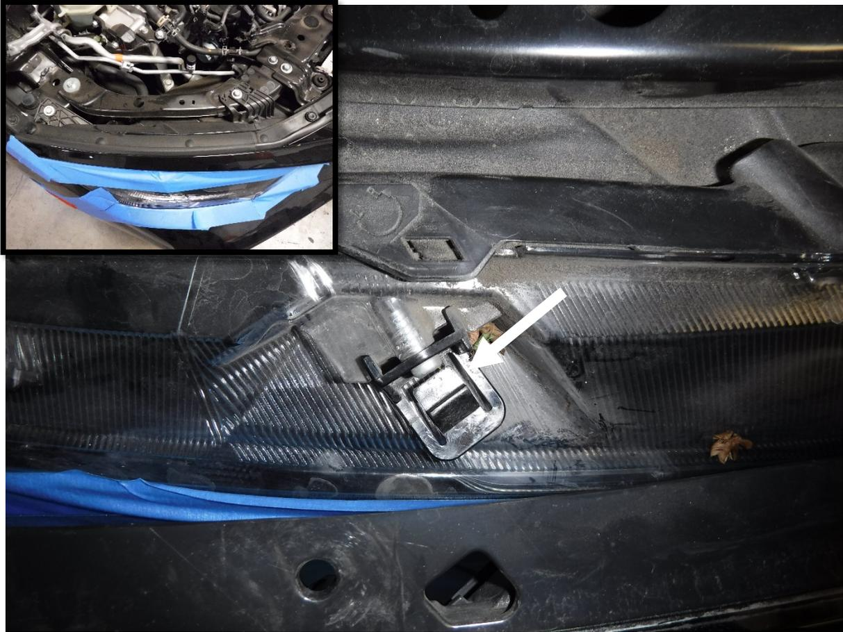
8. Remove the clips securing the trim seal across the top of the bumper.
