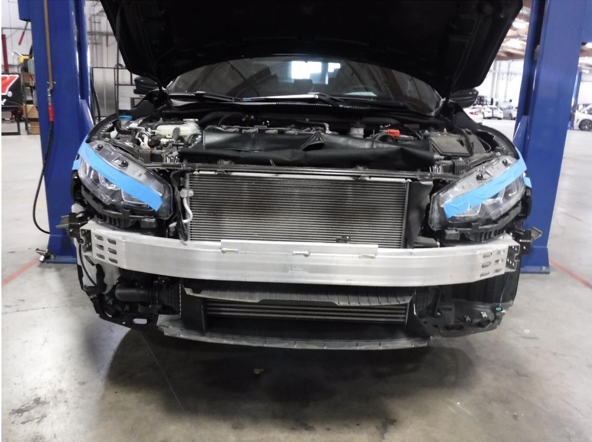
12. If the vehicle is equipped with fog lights, disconnect the connector for each of the fog lights once sides of bumper are unclipped from the vehicle.
