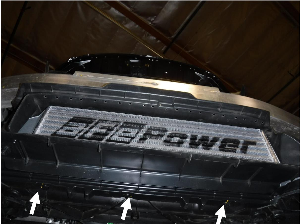
36. Install the aFe intercooler into the vehicle.
