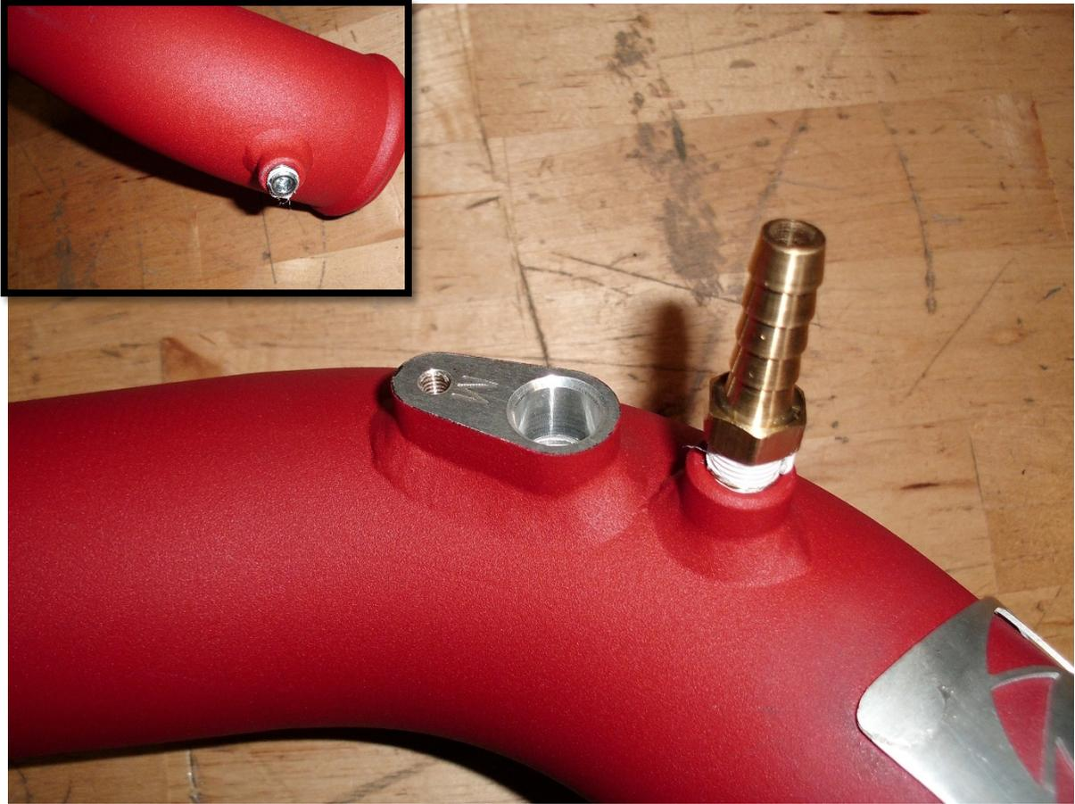
**Note: Be sure to use thread sealant on the plugs, sensors, or fittings to prevent any leaking**
