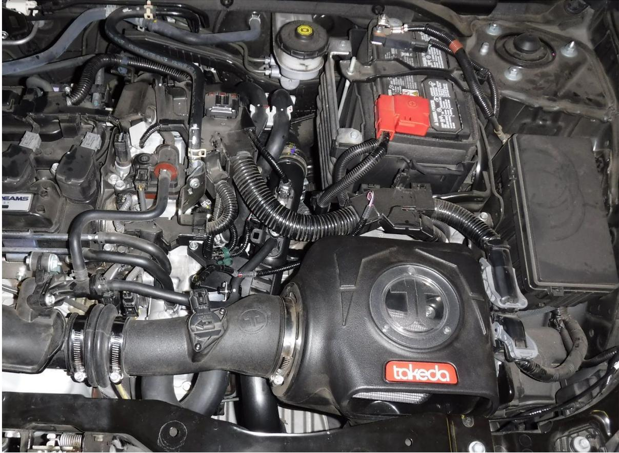
14. Disconnect the MAF sensor on the intake tube.
