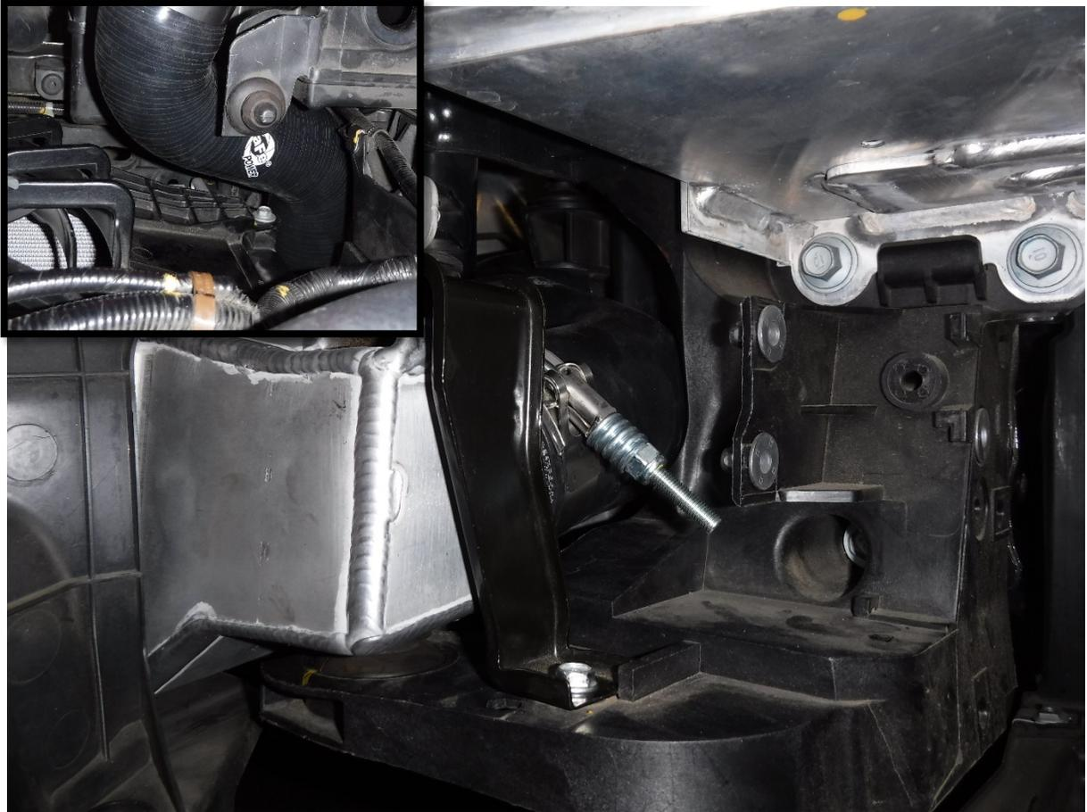
52. Install the supplied silicone hose along with one (1) of the supplied 2-3/8" clamps onto the intercooler from the top (do not tighten the clamp yet).
