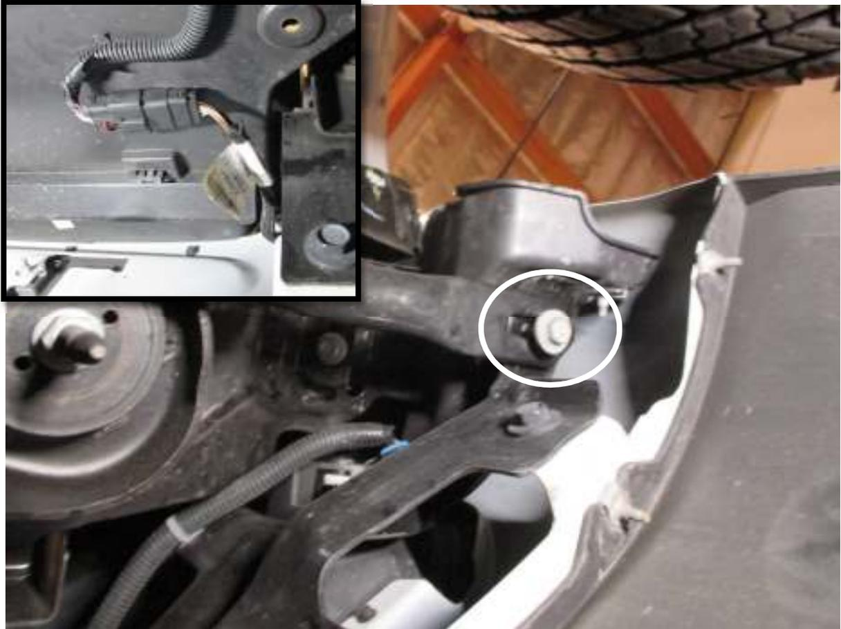
10. Disconnect the wire harness for the bumper from underneath the vehicle directly behind the license plate.
