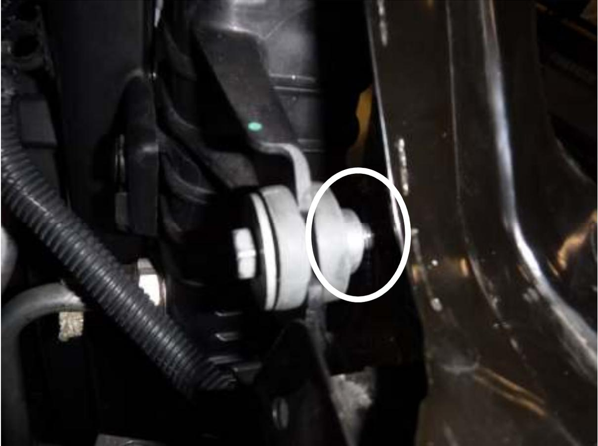
55. Place the radiator on the mounts on the back side of the aFe intercooler.
