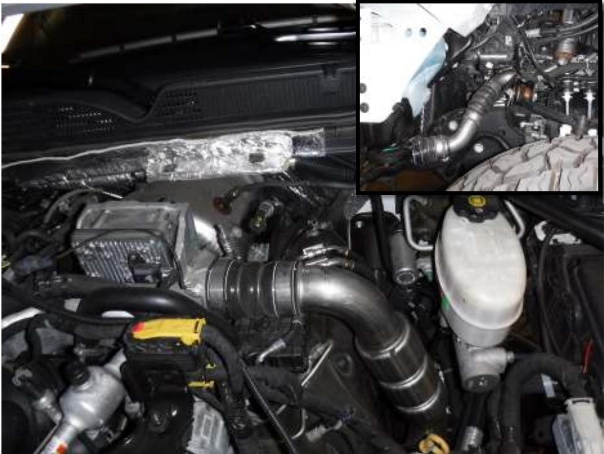
20. Loosen the clamps for the hot side intercooler tube at the turbo outlet and intercooler inlet on the driver side of the vehicle using a 11mm socket.
