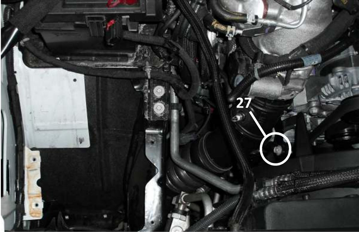
25. Remove the lower air box mounting bracket from the vehicle using a 10mm socket and a flat head screwdriver to release the transmission lines from their mount.
