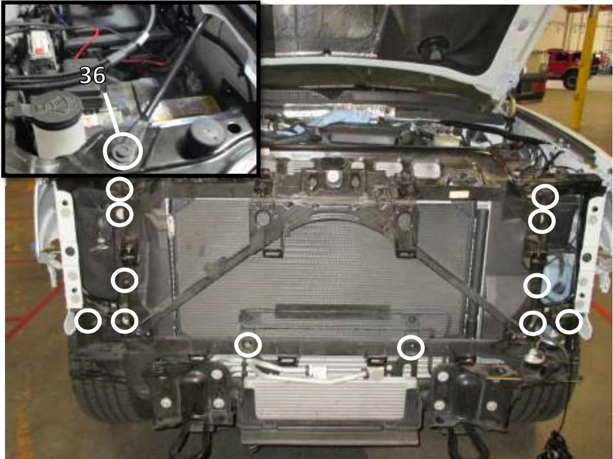
36. Remove the bolt securing the brace (on the drivers side) to the upper core support using a 10mm socket and push the brace out of the way.
