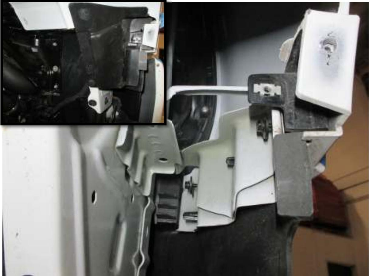
14. Remove the plastic cover in the wheel well to expose the bolts securing the air deflectors onto the vehicle, using a panel popper or flat head screwdriver.
