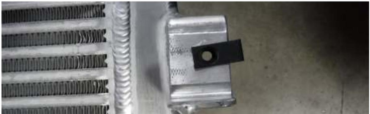
49. Once the factory intercooler is out of the vehicle, transfer the two (2) rubber grommets on the bottom pins over from the factory intercooler to the supplied aFe intercooler.
