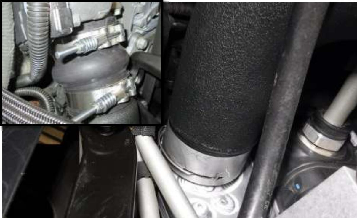
74. Place the 3.38" clamp onto the coupling and connect the coupling to the engine.
