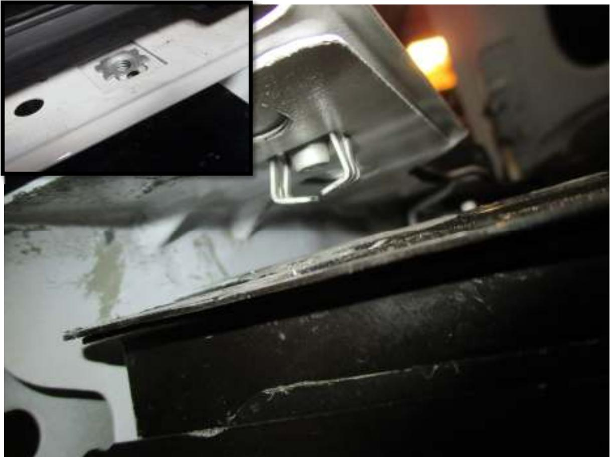
40. Remove both headlight mounting clips from the fenders, by squeezing the ends underneath the fender together and pulling it out of the top.
