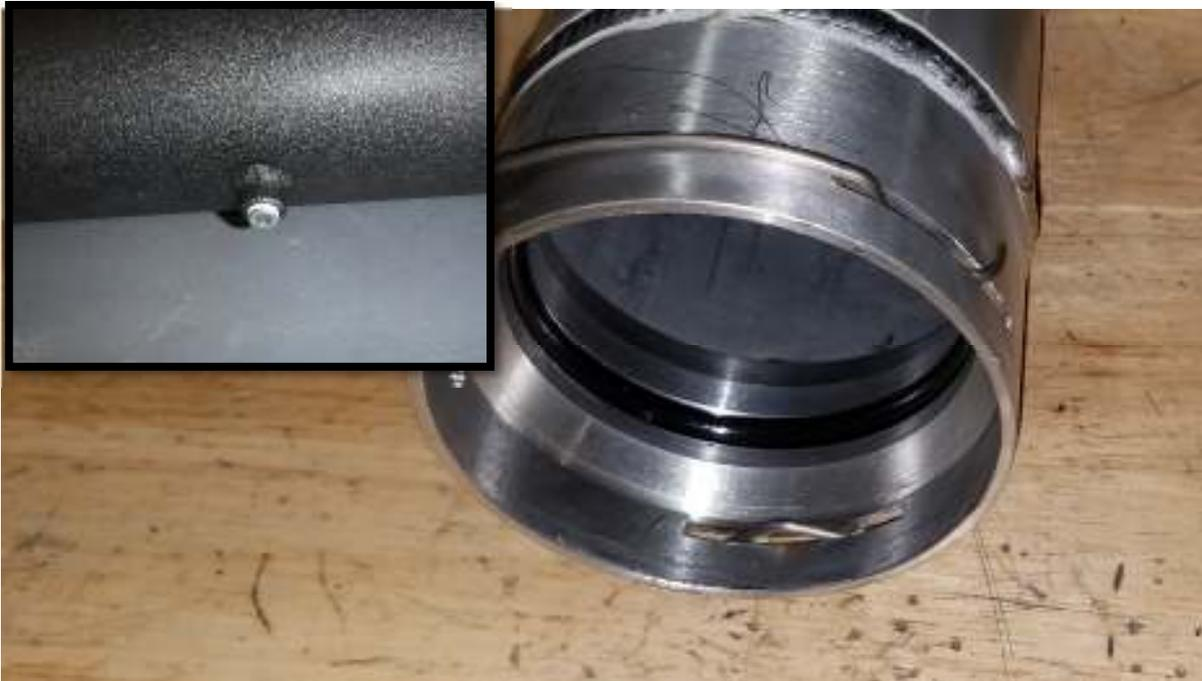
**Note: Be sure to use thread sealant on the plugs or sensors to prevent any leaking**
