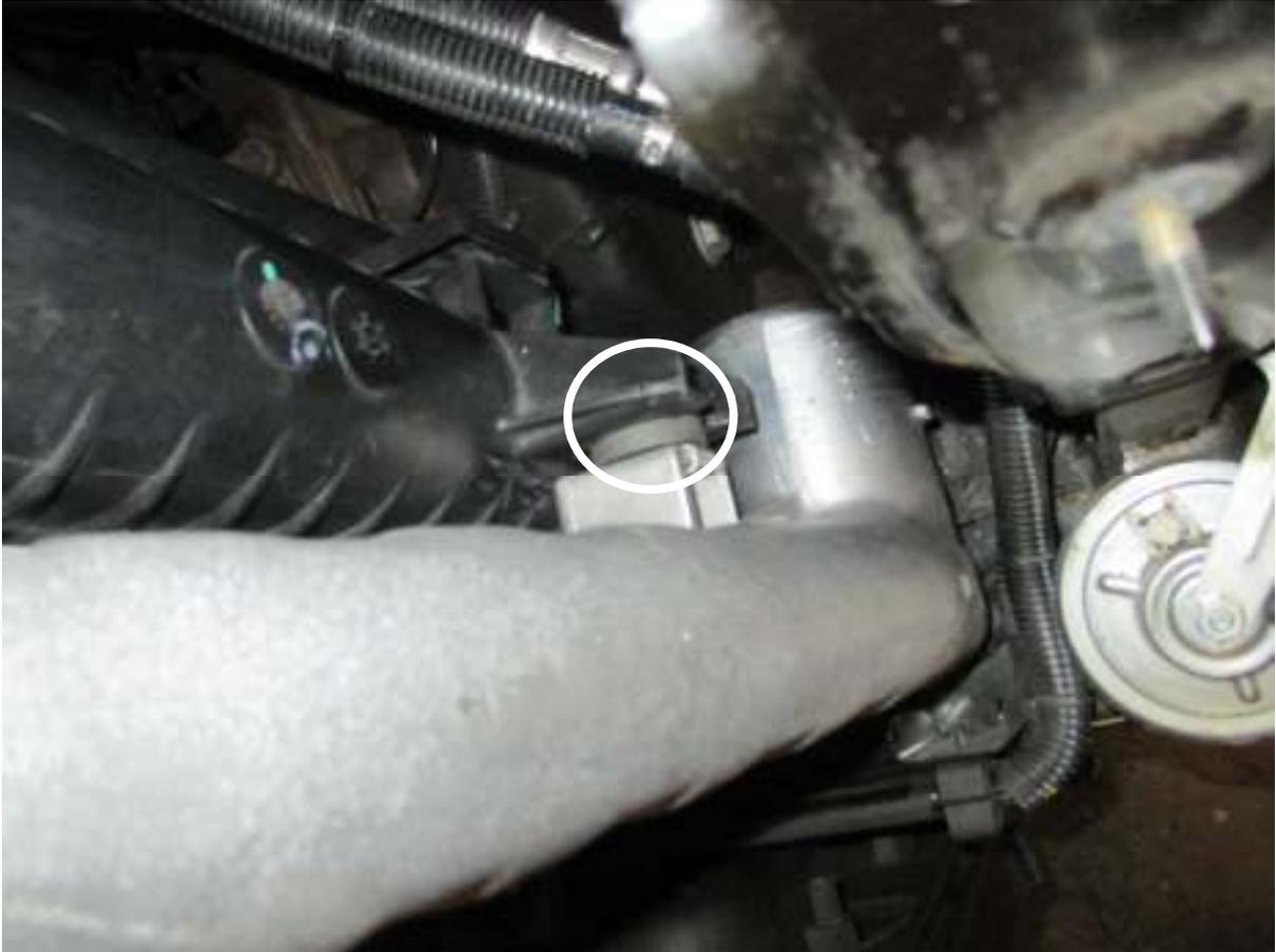
43. Remove the four (4) bolts securing the radiator to the intercooler using a 13mm socket.
