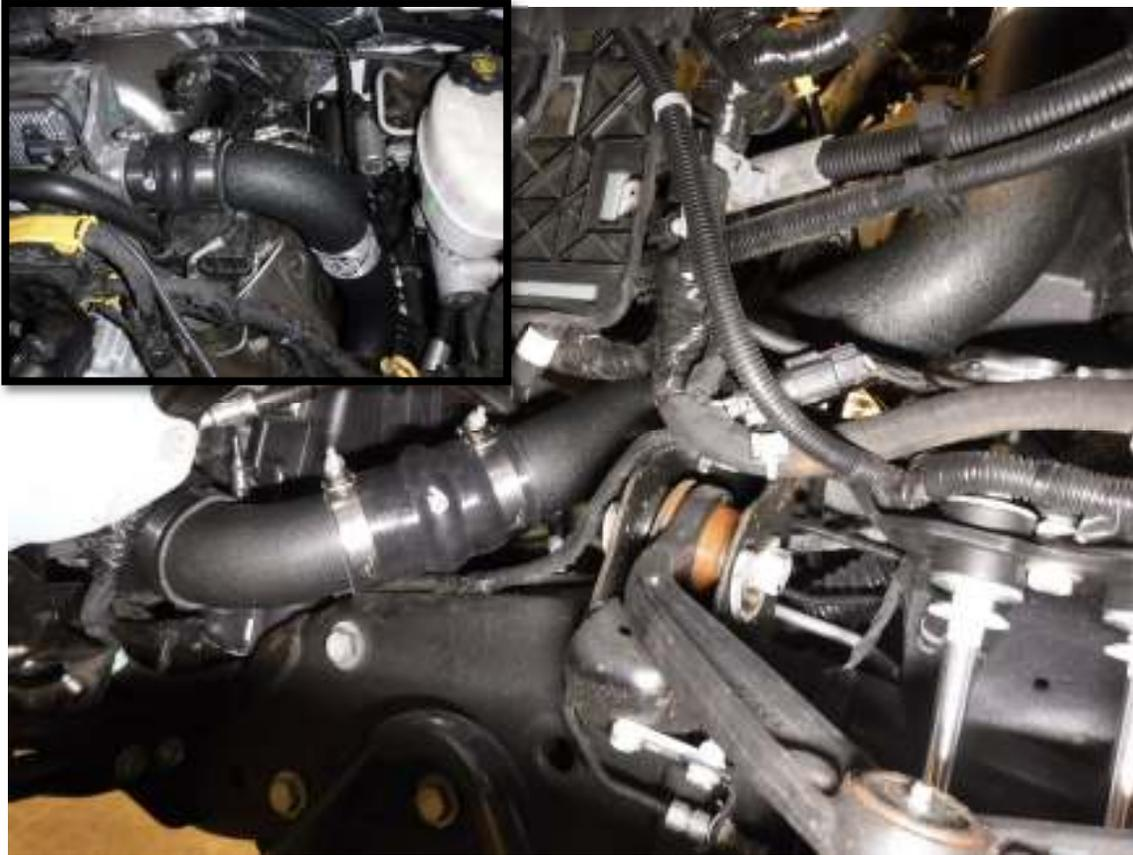
79. Install one of the 3" clamps and the small hump coupling onto the turbo.
