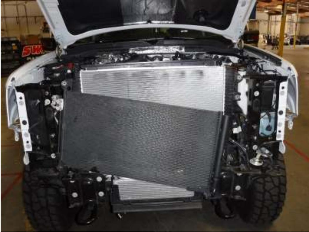
45. Remove the two (2) bolts securing the power steering cooler to the vehicle using a 10mm socket.
