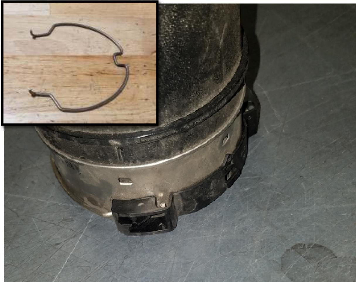
67. Stand the factory intercooler tube up on the end with the metal adapter.
