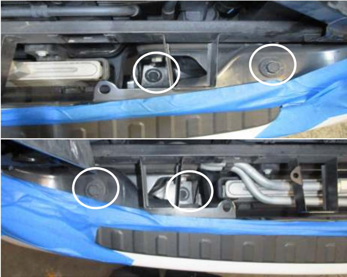
12. Remove the four (4) bolts across the front of the bumper located near the tow hooks, using a 18mm socket.
