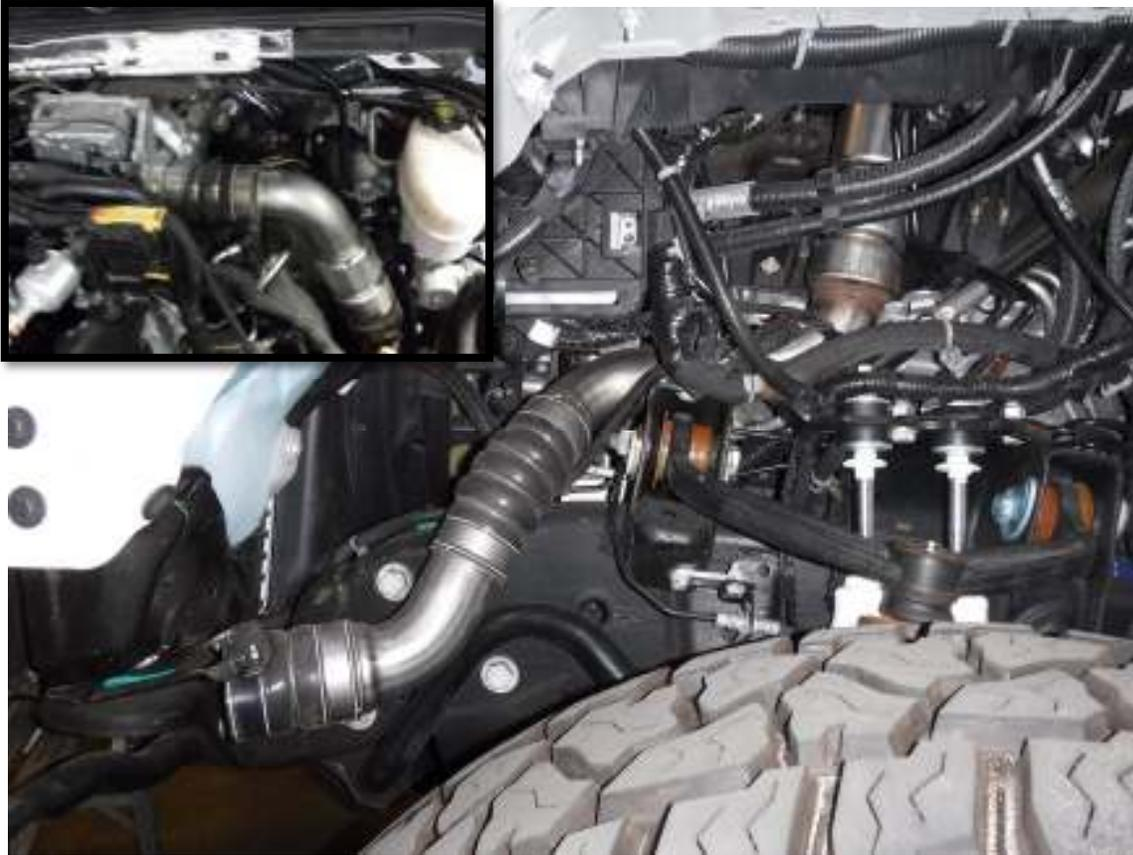
72. Reinstall the factory hot side intercooler tube into the vehicle from the bottom.
