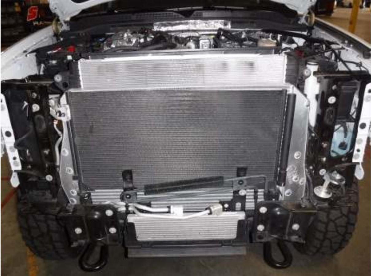
52. With some help, install the aFe intercooler into the vehicle very carefully. You will need to maneuver the intercooler around the radiator and some A/C lines.
