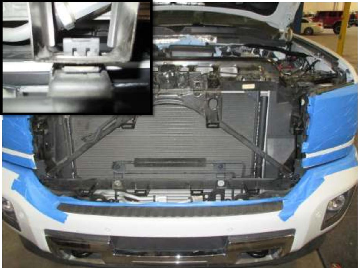
5. Remove the four (4) mounting screws on the top of the grille, using a 10mm socket.
