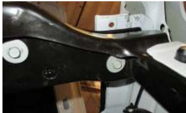
41. Remove the two (2) bolts securing the radiator to the core support from the back, using a 13mm socket.
