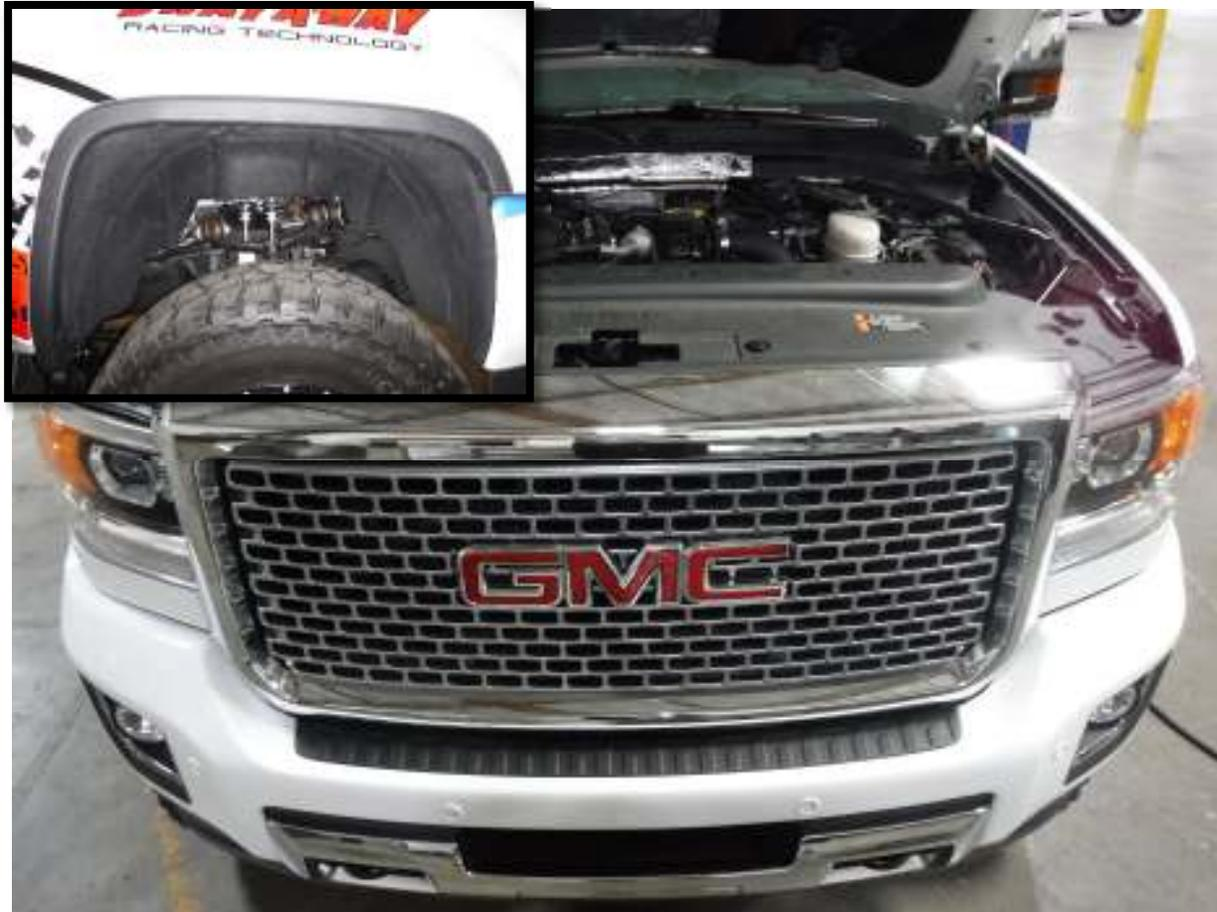
82. Reinstall the wheel wells and fender flares onto vehicle and tighten all bolts.
