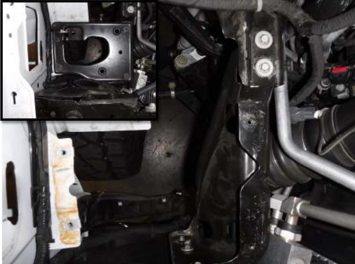
70. Reinstall the lower air box mount into the vehicle and tighten all the bolts using a 10mm socket.
