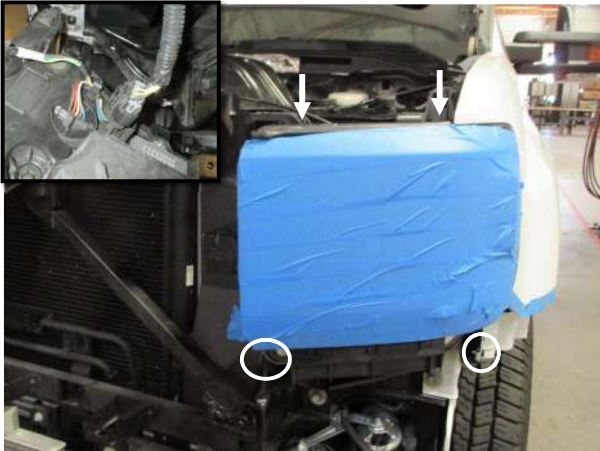
17. Remove the hood seal along the passenger side of the fender by pulling straight up to release the tape securing it to the fender.
