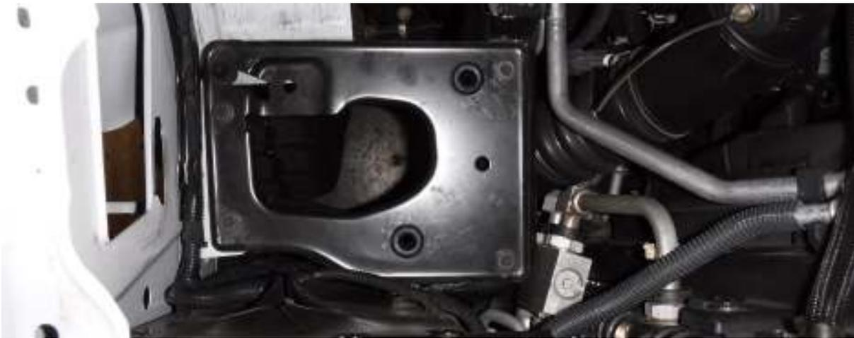
22. Disconnect the Mass Air Flow sensor from the intake tube.
