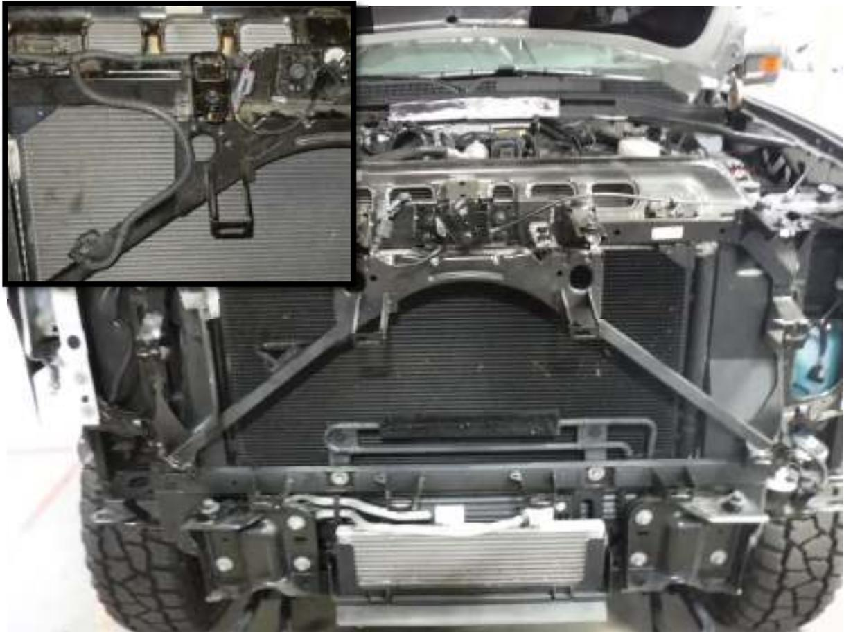
61. Reinstall the bolt securing the passenger side brace to the upper core support and tighten using a 10mm socket.
