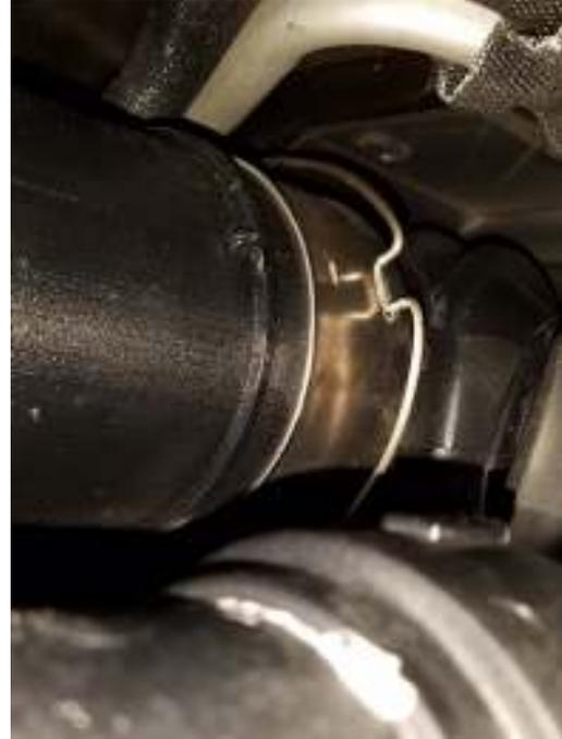
28. To disconnect the intercooler tube from the engine you will need to rotate the grey ring at the top of the tube to the left slightly and pull it downwards to release it from the engine.
