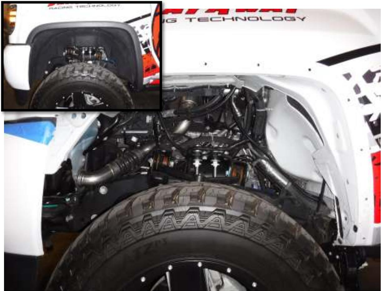
8. Remove both front fender flares from the vehicle using a T15 Torx and a 13mm socket.
