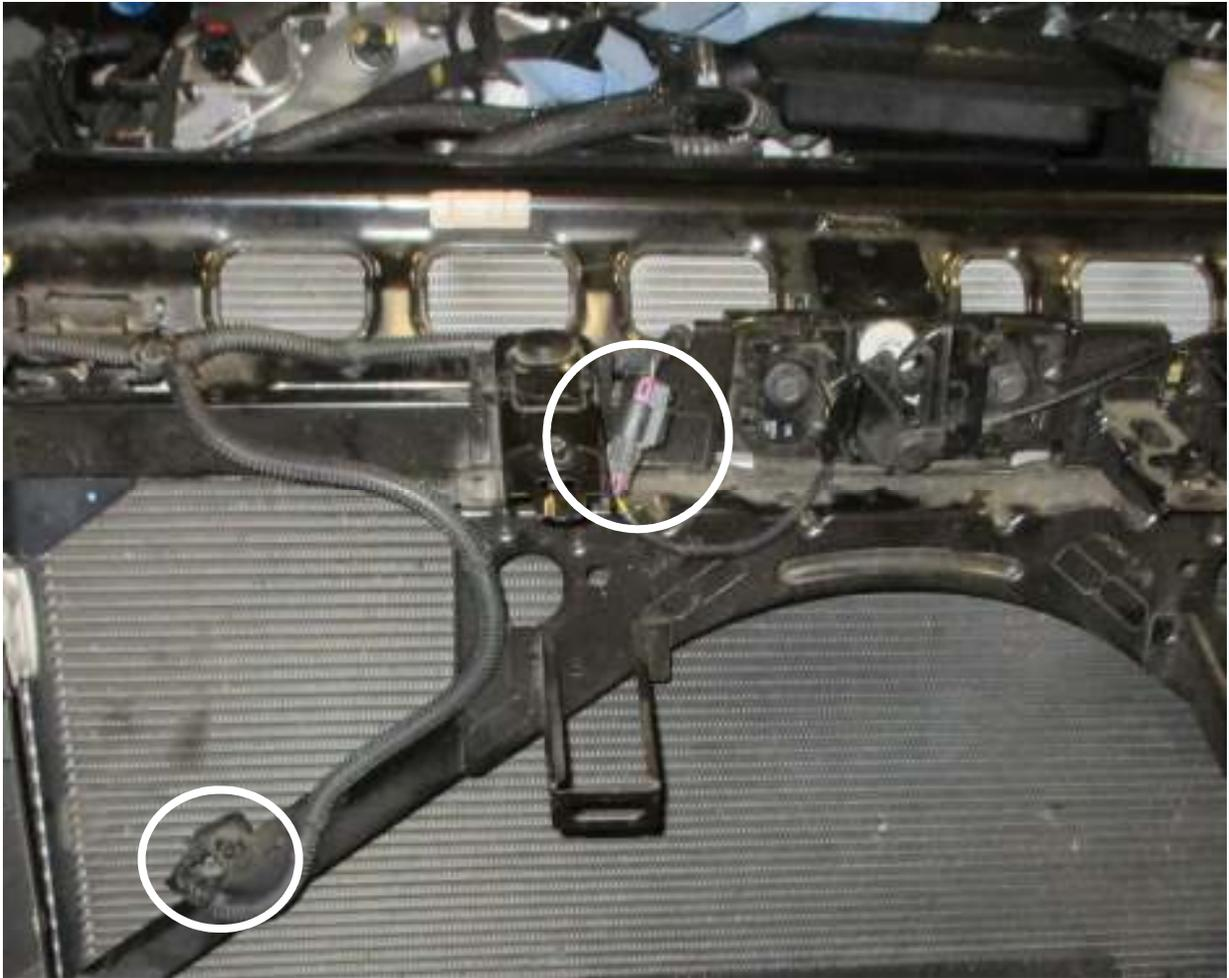
34. Disconnect the temperature sensor and hood latch from the wiring harness.
