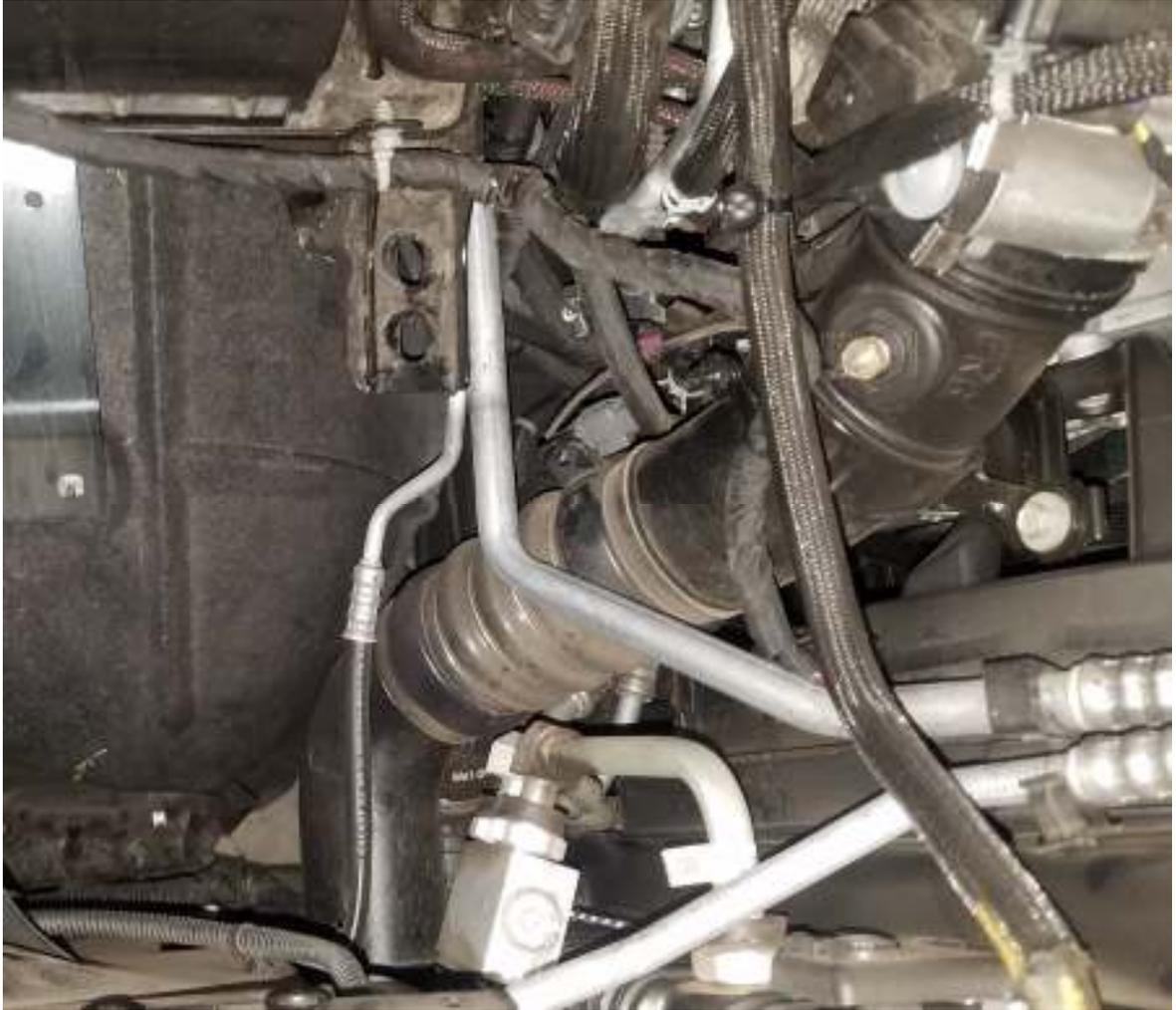
67. Reinstall the factory cold side intercooler tube into the vehicle by first connecting the intercooler tube to the engine inlet, then connecting the intercooler tube to the intercooler connection.
