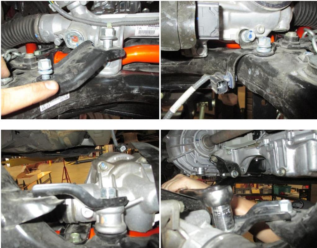
5. Reconnect steering rack wiring harness. This will complete the rack install.
