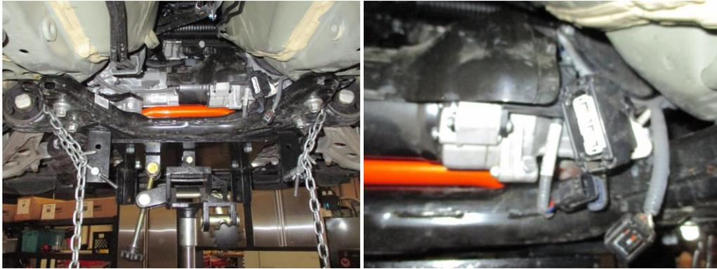
7. Secure the rear subframe, by re-attaching the left and right brackets. Shift subframe as required to keep everything aligned. Go back and torque the previously snugged subframe fasteners.
