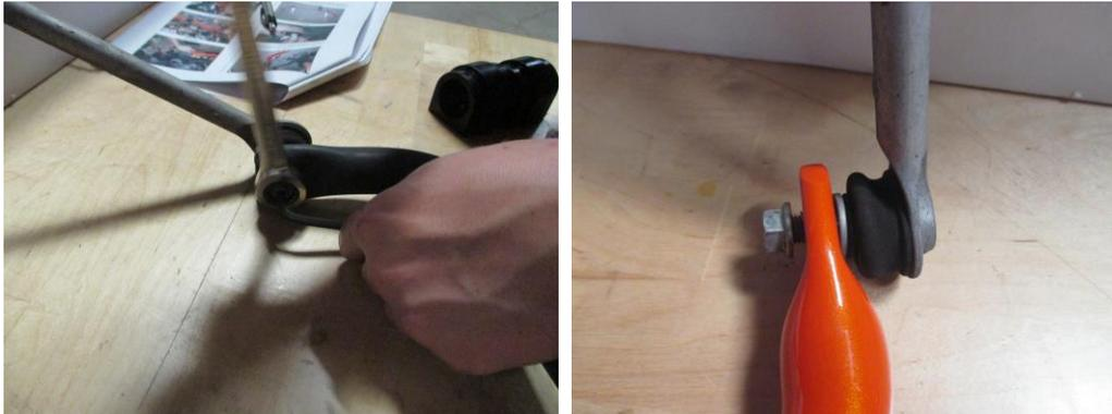
2. Reinstall the new sway bar by raising into the sub frame, in the pictured orientation.
