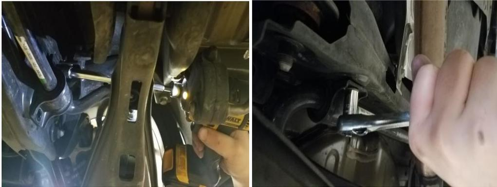
5. Remove the OEM bushing brackets on both sides of vehicle.
