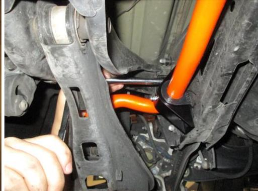
4. Double check all your work and re-install sway bar and tighten down sway bar brackets.
