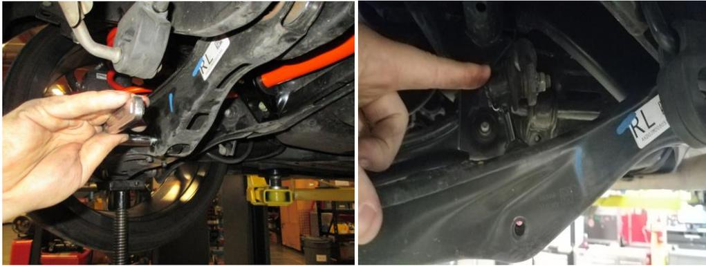
4. Remove the driver and passenger side sway bar mounts
