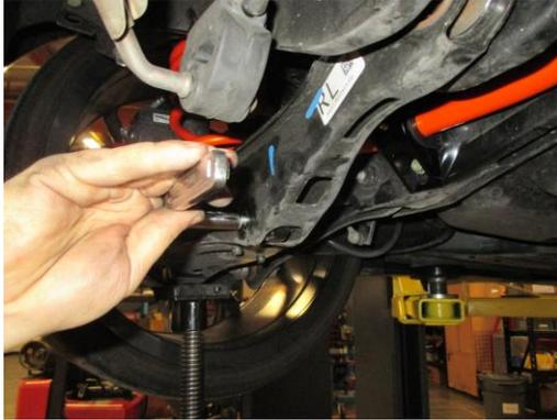
6. Double check all bolts and hardware, reinstall the tires and torque to oem specifications.
