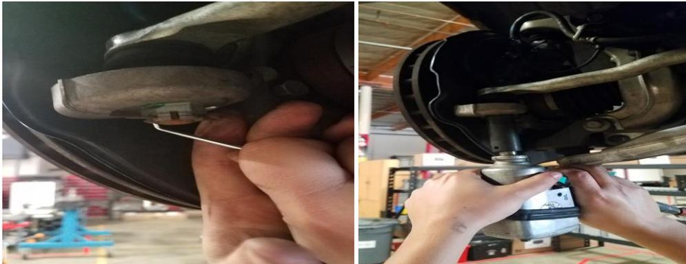
12. Using a screw jack, support the subframe, then remove the left and right side forward sub frame bolts. We chose to place the screw jack forward on the subframe near the lower control arms, this is helpful in the next step.
