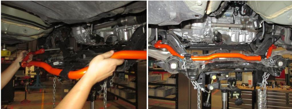
3. Reinstall the OEM brackets, carefully noting the correct orientation. Reattach the mounting hardware, and tighten bolts.
