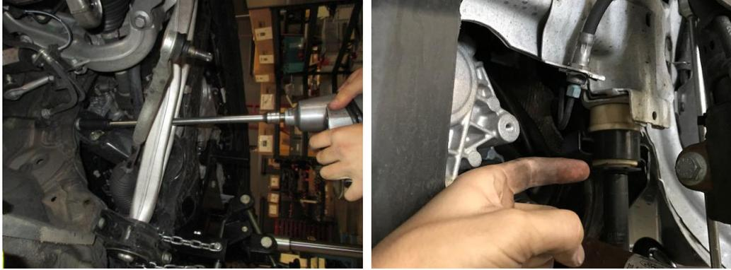
13. Slowly lower the subframe, be careful to ensure that you are not binding on anything and that all electrical connections and lines are free and not under tension. We were able to achieve this step by rotating the subframe back, and not completely dropping it from the vehicle. In this step be careful and make sure the steering spline does not get caught on anything.
