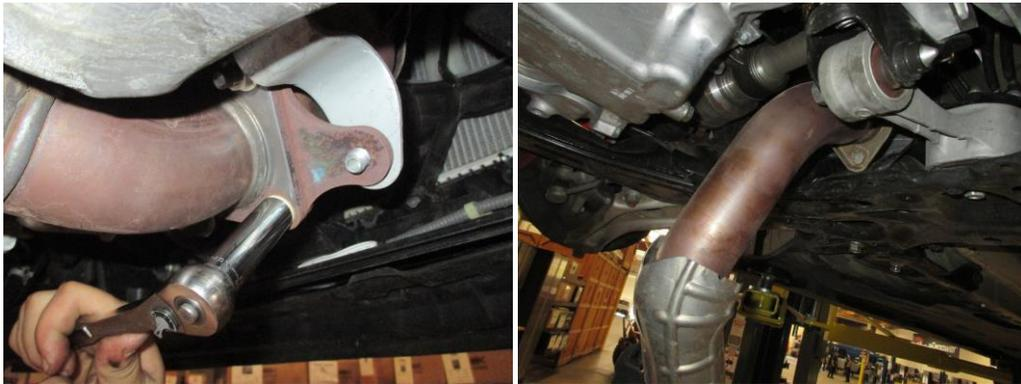
10. Loosen and remove the 19mm bolt that hold the engine mount. Remove sub frame braces using a 17mm socket.
