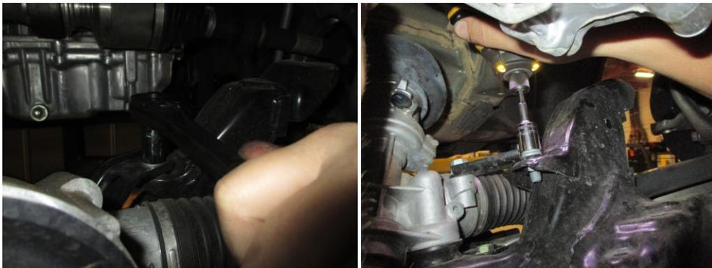
15. With the rack bolts removed you disconnect rack wiring harness. Now you can remove the whole rack from the sub frame.
