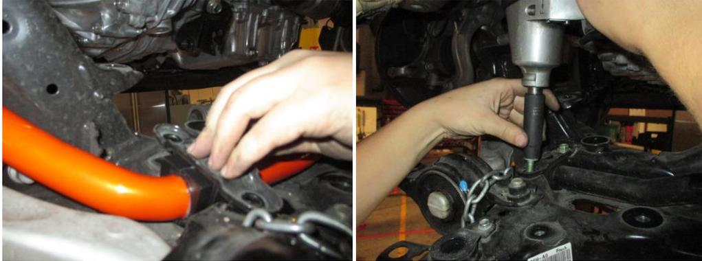
4. You can now reinstall the steering rack into the sub frame. Tighten down all bolts that hold the rack into the sub frame.
