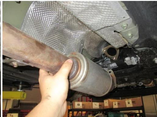
7. Loosen and remove the 14mm bolts that secure the heat shield to the vehicle.
