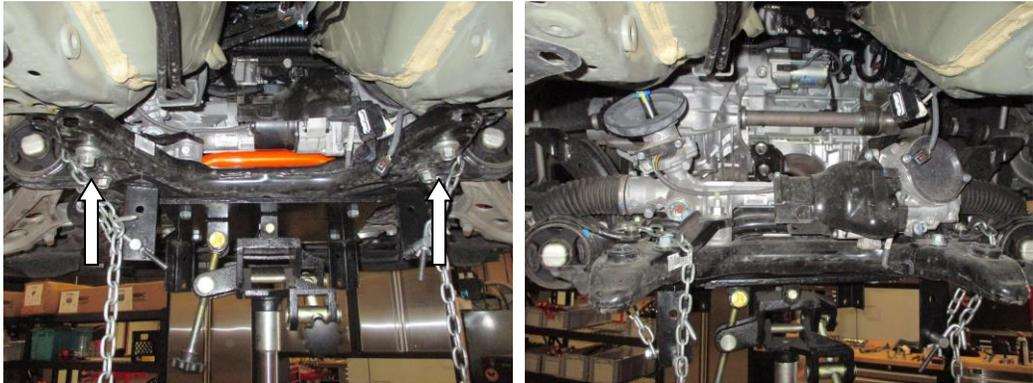
14. You can now access the steering rack bolts that hold the rack to the sub frame. Remove the 9 bolts that hold the rack to the sub frame.
