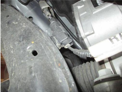
11. Re-secure the bracket that holds the transaxle bracket to the subframe.
