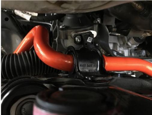
4. You can now raise the subframe back up into position. Be careful to make sure nothing is binding or pinching. You can use a pry bar to help align the subframe bolts. **Do not fully tighten bolts yet, just snug to hold position.**
