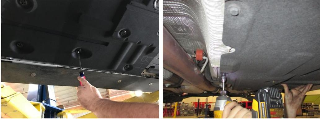
6. Remove the rear main subframe brace by removing the four nuts and bolts that secure it to the vehicle.
