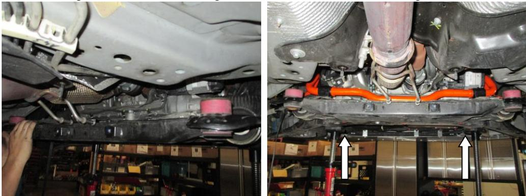
14. Alternate method to step 13. Remove the 3 bolts that secure the steering rack to the subframe. Using a ratchet strap secure the tie rods to the strut assemblies. This will keep them in place during the next step as the sub frame is lowered. Failure to do this could cause damage to the steering.
