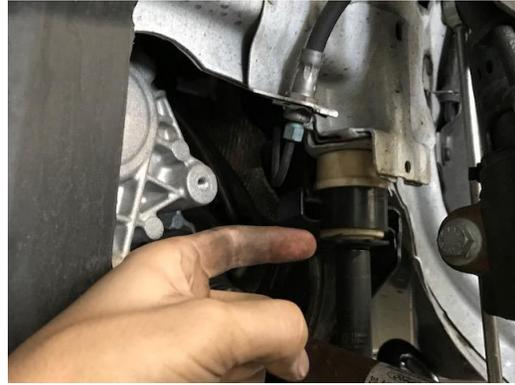
6. If removed in step 14 of disassembly, secure the steering rack by reattaching the 3 OEM bolts as removed.
