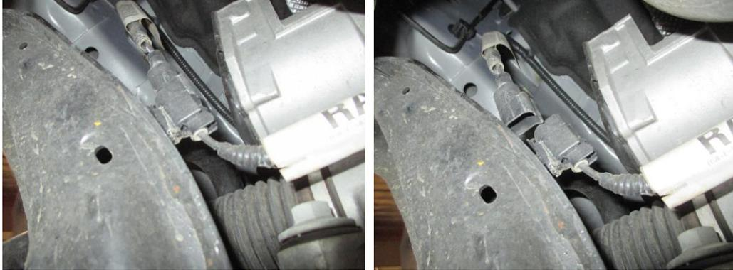
12. Using a screw jack, support the subframe, then remove the left and right side forward sub frame bolts. We chose to place the screw jack forward on the subframe near the lower control arms, this is helpful in the next step.
