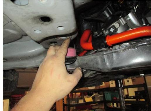
5. You can now reinstall the forward subframe bolts. Since some final adjustment will be done when you reinstall the braces, these **bolts only need to be snug at this time, do not completely tighten.**
