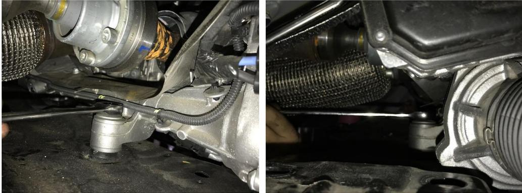
15. With the subframe lowered, you can now access the bolts that secure the sway bar bushing brackets to the subframe. Remove the bolts.
