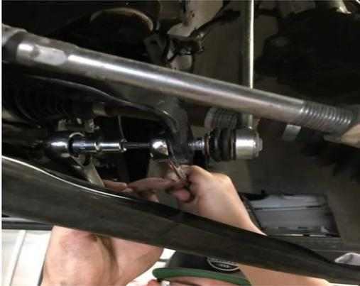
5. To gain access to the rear subframe brace attachment points, remove the plastic rivets that secure the side underbody covers. You will only need to access the forward portion by pulling down on the cover.
