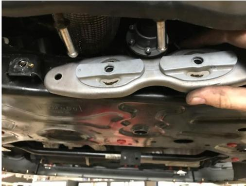
9. Loosen and remove the left and right side subframe brackets by loosening and removing the bolts that secure them in place.
