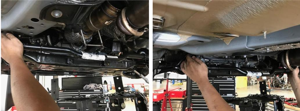
17. Before removing the brackets, take time to note the orientation of the OEM brackets, the holes are offset and this orientation will need to be followed upon reinstallation.
