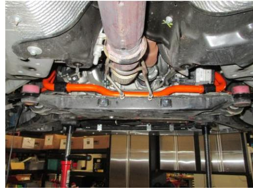
3. Reinstall the OEM brackets, carefully noting the correct orientation, as the holes are offset. Reattach the mounting hardware, and tighten bolts. Reinstall the OEM end links to the new bar, in the same orientation as removed from the OEM bar. Proper placement would put the end link on the outside of the bar, and the nut on the inside.
