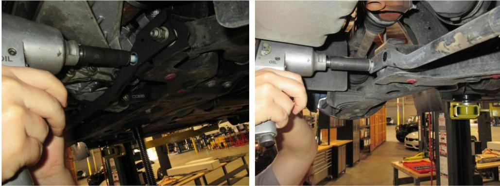
8. Loosen and remove the two bolts that secure the exhaust hanger to the subframe.
