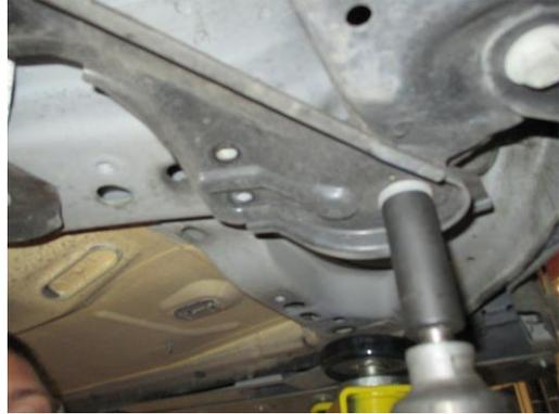
8. Reinstall the rear main subframe brace.
