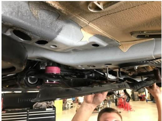
9. Re-attach the rear exhaust hanger bracket to the subframe.
