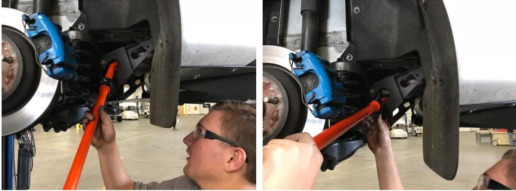
2. Reattach the OEM sway bar bushing brackets and heat shield.
