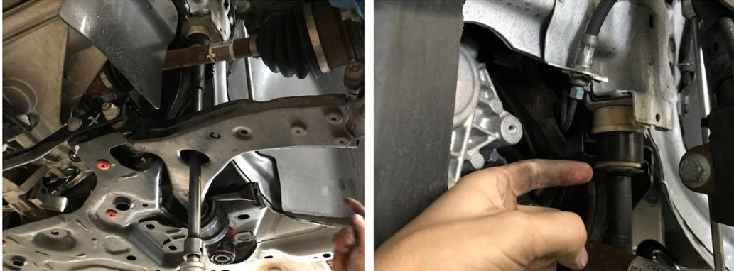
13. Slowly lower the subframe, be careful to ensure that you are not binding on anything and that all electrical connections and lines are free and not under tension. We were able to achieve this step by rotating the subframe back, and not completely dropping it from the vehicle. In this step be careful not to pull too far, as the steering rack is still connected to the steering shaft.
