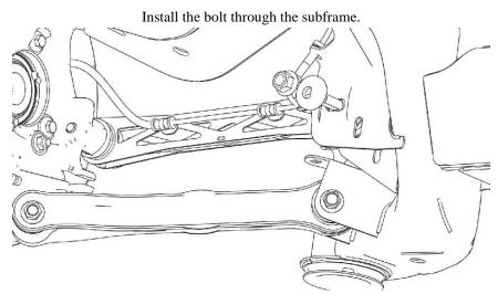
Install the washer and nut and tighten using the 21mm box end wrench and 21mm socket and ratchet.
