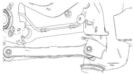
Using a 21mm socket, ratchet and 21mm box end wrench remove the nut and washer from the subframe bolt.
