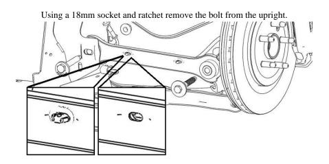
Remove the two clips retaining the ABS sensor by squeezing the tabs on the front and pushing the tab through the hole.
