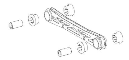
Clean the mating surfaces of the bushings and the tie rod with mild cleaner. Press the bushings into the control arm bores from each side.
