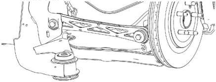
Install the bolt into the upright and tighten using the 18mm socket and ratchet.
