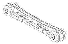
Press the sleeves into the bushings. Use the excess grease to lubricate the faces of the four bushings. The end faces of the sleeves do not require grease.
