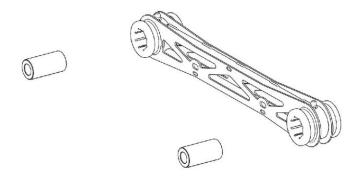
Using the provided grease, grease the inside of each bushing and the outside of each aluminum sleeve. Try and fill the grooves in the bushing with the grease.
