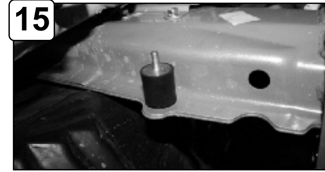
15 Install isolation mount to frame.
