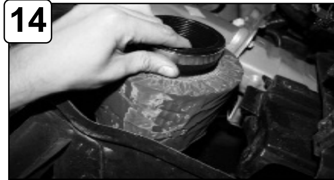
14 Attach pre-filter to filter and place filter inside front of driver side wheel.
