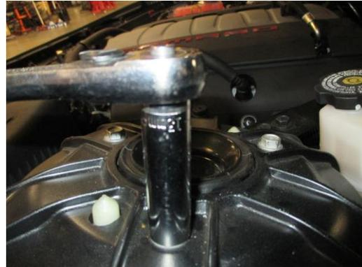
3. Slide the spindle upright back onto strut and attach the bolts and nuts. Using a 21 mm socket and 15/16" wrench, torque the 2 bolts that holds the OEM strut into the upright to 52 lb-ft.
