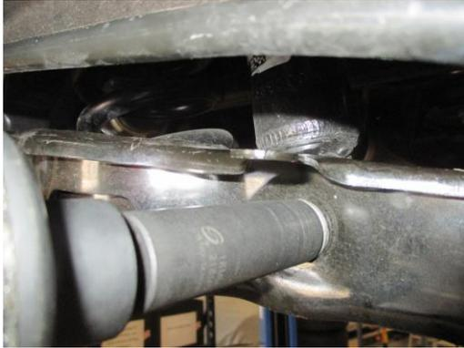
6. Re-attach the end links to the upright and torque to 25 lb-ft.
