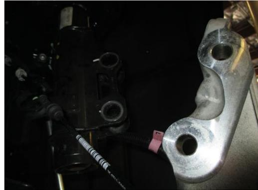
7. If the vehicle is equipped with Selective ride you will need to disconnect the connector before removing the OEM strut from the vehicle.
