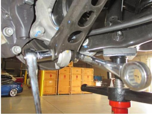
6. Using a 18 mm wrench and 15 mm socket remove the bolt holding the lower control arm to the upright. Slowly lower the control arm to release tension on the OEM springs, and remove spring from vehicle.
