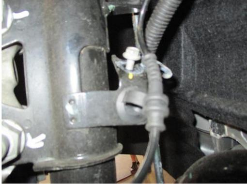
6. Using a 21 mm socket and 15/16 wrench, remove the 2 bolts that holds the OEM strut into the upright. Slowly lower the jack and slide strut free from upright.
