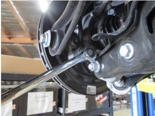
4. Using a 18 mm wrench, disconnect the OEM shock from the lower control arm.
