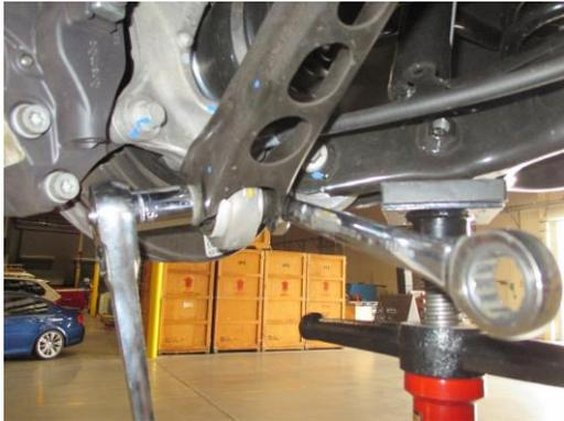
5. Install the lower shock bolt and Torque the 18 mm nut to factory specs.
