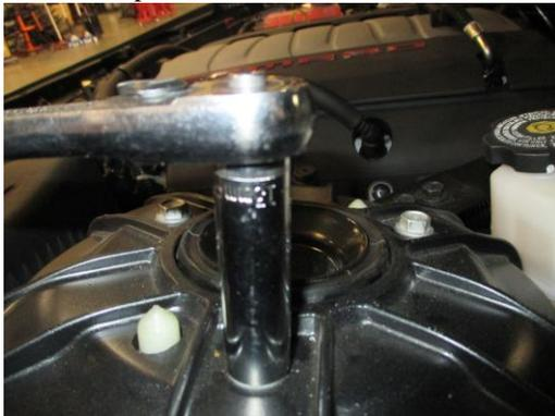
9. Using a strut compressor, remove the factory springs from the strut, by removing the top nut, using a 18mm socket. Remove the upper strut mount, spring seat, and spring isolator. It is not necessary to remove the rubber boot, or the bump stop.
