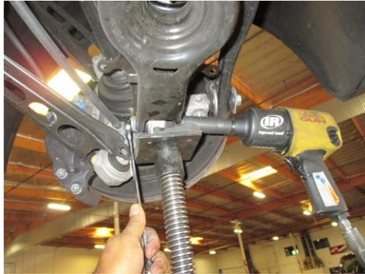
4. Using a 18 mm wrench and 15mm socket, reattach the trailing arm and torque to factory specs.
