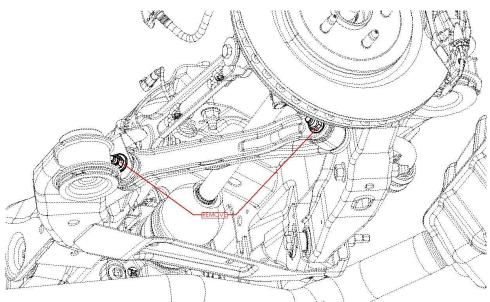
Using the 18mm socket and 18mm box end wrench remove the two bolts and nuts holding each trailing arm in the car.
