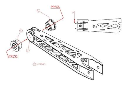
Clean the surfaces of the trailing arm and bushing as shown. Press the polyurethane bushings into the trailing arm. The flange faces should be touching the sides of the trailing arm.
