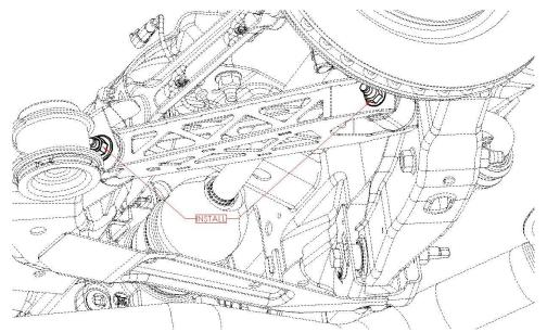
Using the 18mm socket and 18mm box end wrench reinstall the two bolts and nuts attaching the trailing arm to the chassis and torque.
