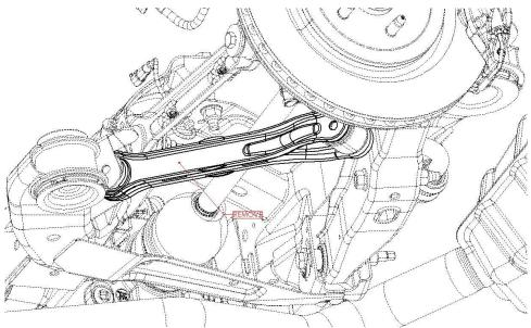
Remove the trailing arm and press bushing from upright.
