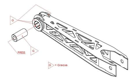
Coat the outside of the aluminum sleeve. Coat the flange and inside of each bushing, filling the grooves, with the provided grease.
