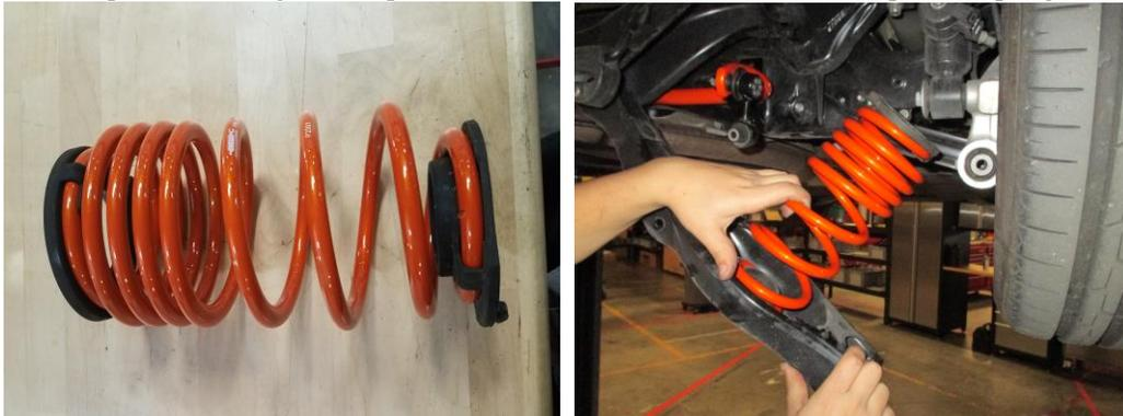
2. Using a screw, or floor jack, raise the lower control arm into position, and align control arm to the upright.
