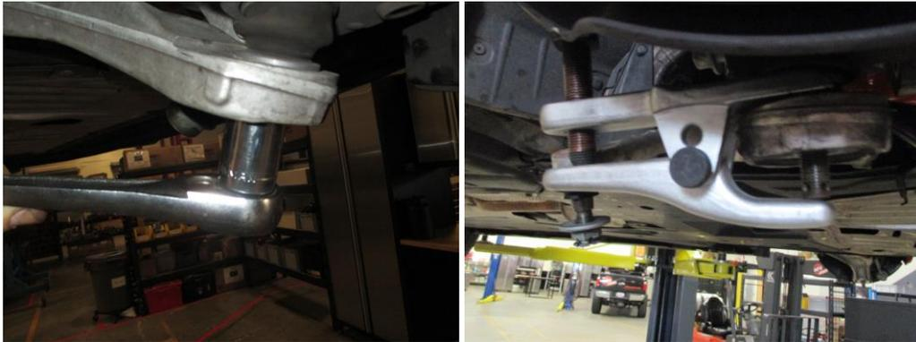
11. Once the lower arm is free. Remove the 2 lower bolts using a 17mm socket that run through the spindle.
