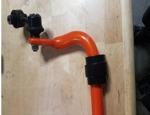
3. Install grease fitting onto supplied brackets, and install onto bar, using factory hardware.
