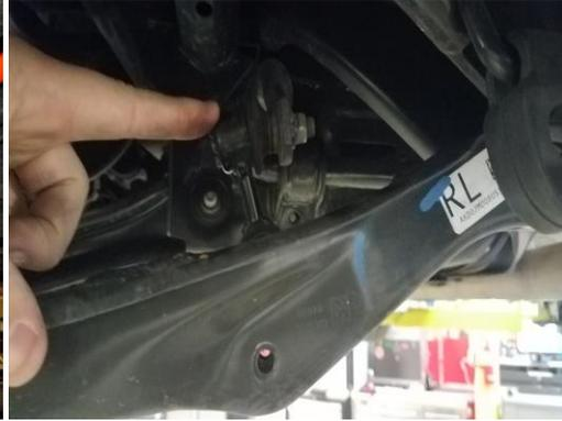
4. Remove the driver and passenger side sway bar mounts
