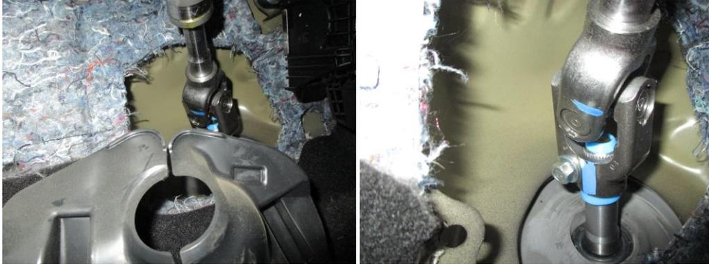
4. Use a 10mm socket to remove steering column bolt. **Before pulling the knuckle apart use a paint pen to mark the orientation of the two parts for proper column alignment later.**
