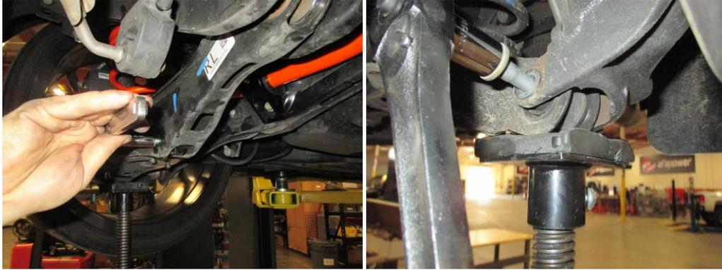
5. Slowly lower the control arm to release tension on the OEM springs, and remove spring from vehicle.
