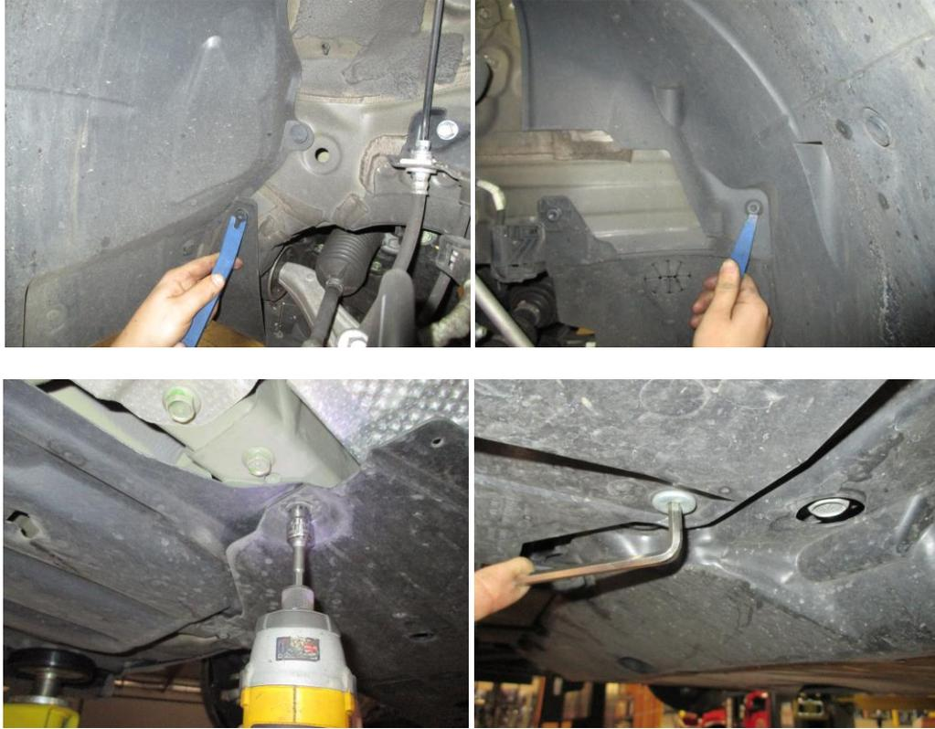
6. Remove the lower crash bar with a 17mm socket. To gain access to the exhaust. Using a 14mm socket remove the 3 nuts to exhaust.
