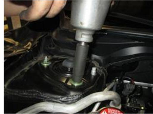
6. Reinstall the strut into the spindle. “WD-40 will help with reinstalling the strut”
