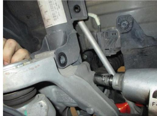
8. Using a 10mm socket remove the plastic shield. This will give you more room to remove the link in the picture. Using a 19mm wrench and a 5mm Allen to remove link.
