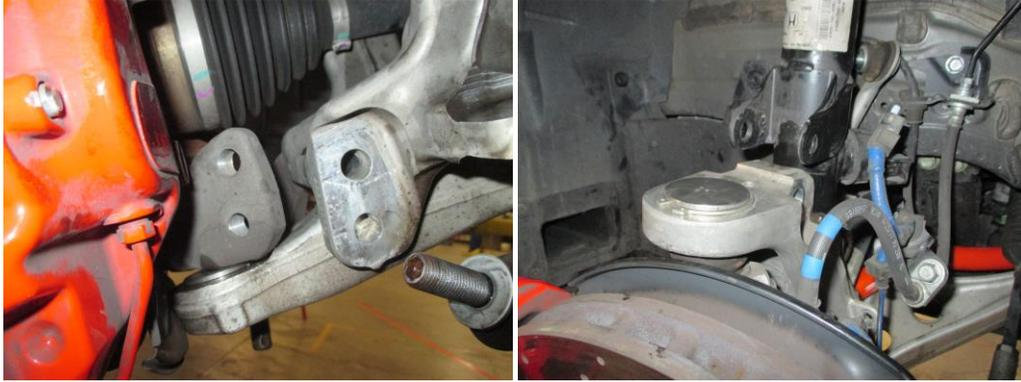
14. Last make sure you remove the top 3 bolts you broke lose earlier so you can remove the strut from the vehicle
