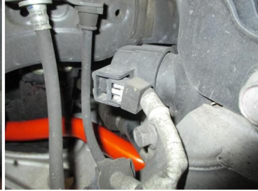
5. Use a 14mm socket to break loose the OEM strut top bolts that hold the strut up.
