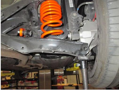
3. Using a 12mm socket, reattach the trailing arm and torque to factory specs.
