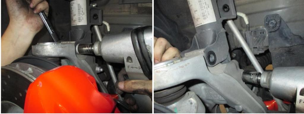
9. Reinstall the sway bar end link, ride height sensor, and reinstall the linkage back on the spindle housing.
