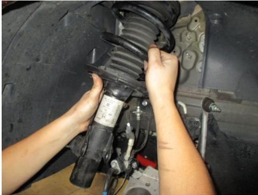
Front aFe Control Coil Spring Installation
