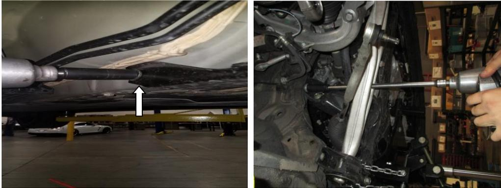
8. Reinstall the rear main subframe brace.
