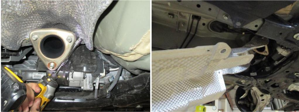
8. Once heat shield is removed from vehicle, disconnect the steering sensor connection. Disconnect steering rack connection on the side of the frame also.
