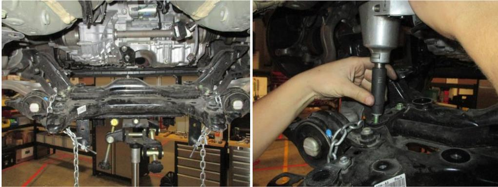
17. Before removing the brackets, take time to note the orientation of the OEM brackets.
