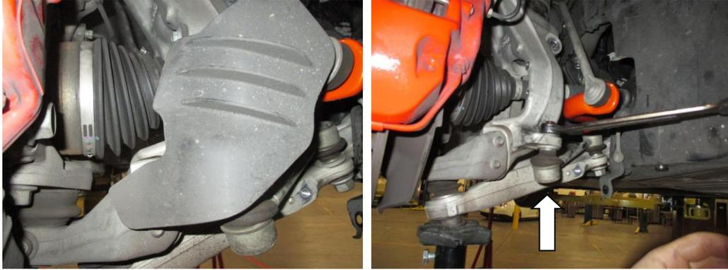
9. Using a 17mm socket remove the lower arm ball joint nut.
