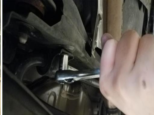
5. Remove the OEM bushing brackets on both sides of vehicle.
