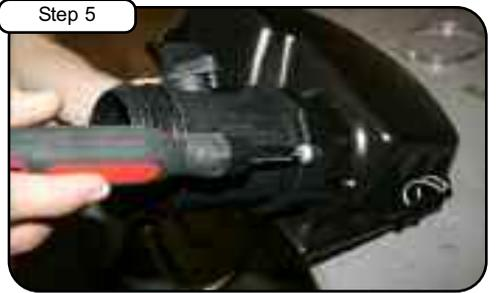
Remove MAF sensor using T30 torx bit.
