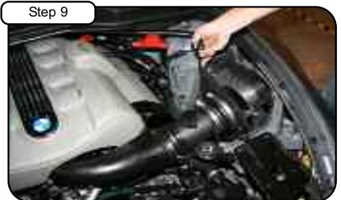
Place MAF sensor into intake tube. (Make sure MAF sensor arrow is in direction towards throttle body.) Now install housing into vehicle. Place other end of MAF sensor into coupler. Do not tighten clamps.
