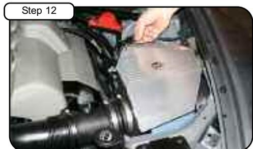
Install cover on housing using button head screws provided and tighten using 5mm allen key.
