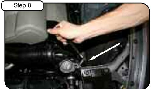
With 10mm socket loosen the bolt holding in windshield washer reservoir. Save bolt for later install.
