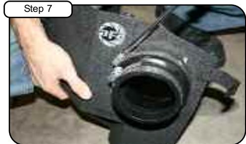
Install coupler reducer to filter adaptor with clamps provided.
