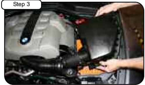
Unclip upper half of air box and lift carefully. Pull back MAF sensor from OE tube.
