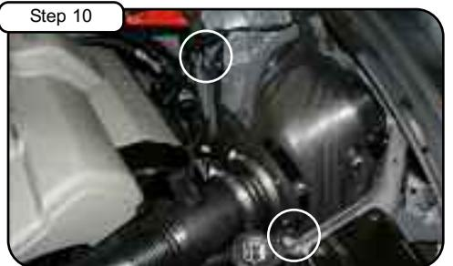
Tighten housing using bolts from step 4 and 8. Tighten all clamps using 5/16" nut driver.
