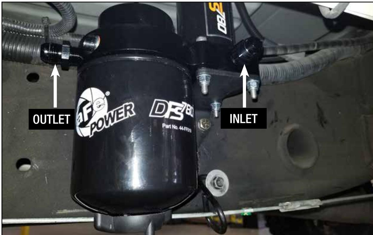
**Step 1:** Mount the supplied fuel manifold assembly to the supplied carbon steel frame bracket using the supplied hardware and tighten:
