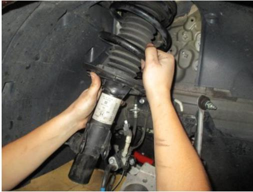
Front aFe Control Coil Spring Installation
