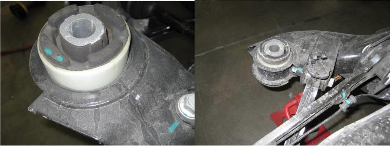
1) With a long, coarse sawzall blade, cut the rubber and plastic in two places on each bushing all the way to the edge (right up against the subframe). That will release compression on the bushing and allow them to be driven out with a dead blow hammer. They come out easily if they are relieved properly.
