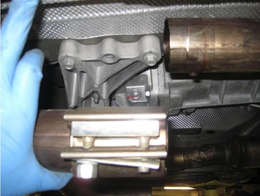
Remove the exhaust system that is fully disconnected now.
