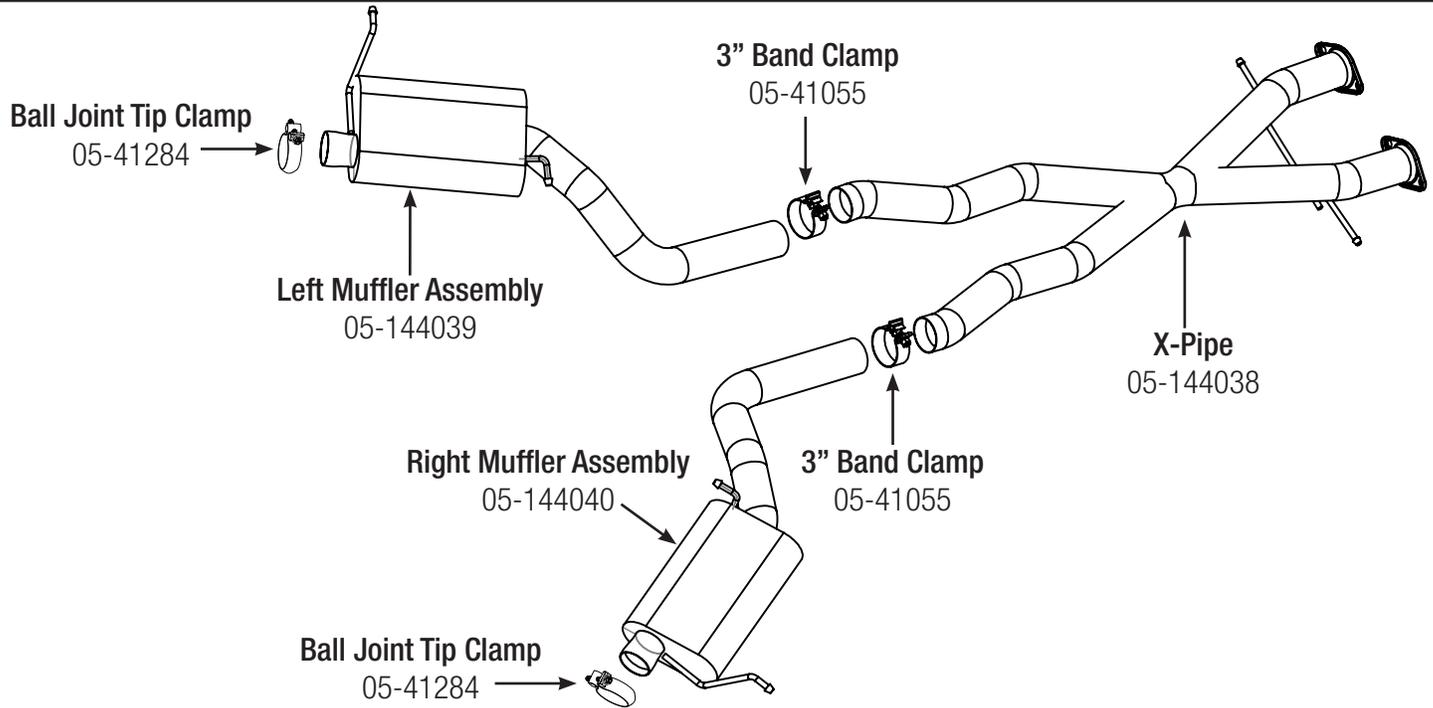
Professional installation is highly recommended. (Read instructions prior to installation) **Make sure to always have at least (2) stands or jacks on hand to support the removal of OE system. As, well as for the installation of aFe system. Any Removal of rubber isolation mounts may require using a spray lubricant such as WD40 and a pry bar.**
