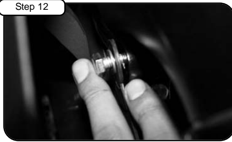
Step 12 Attach screw through fan shroud hole and tighten to manifold. See Notes 2 & 5
