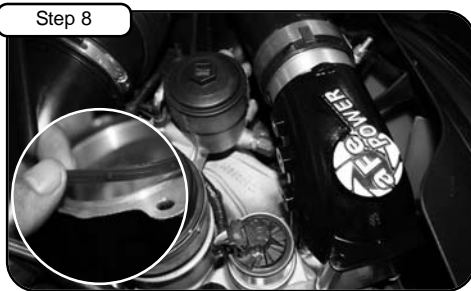
Step 8 Install 1/8" NPT plugs to back of manifold. Tighten using 3/16" allen key. Attach new seal ring to bottom of manifold. Install new aFe BladeRunner manifold to vehicle. See Notes 2 & 3.
