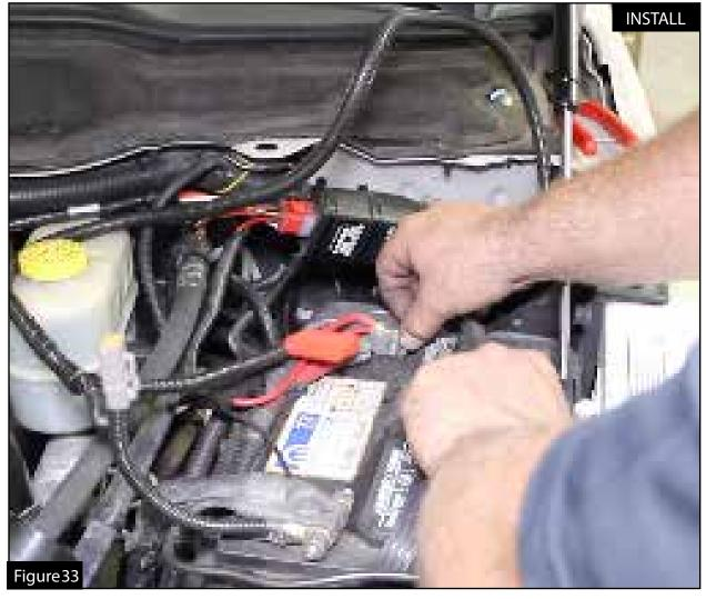
Step 43: Connect the red wire ring terminal to the positive side of the battery.
