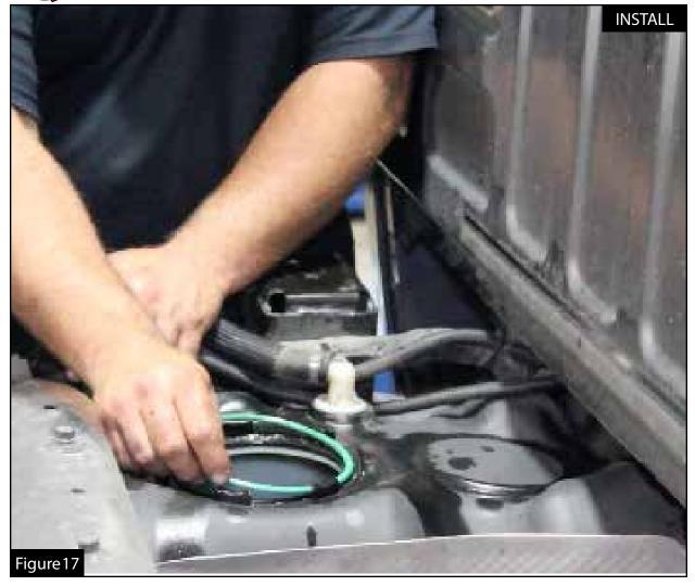
Step 23: Wipe around the fuel tank thoroughly and install the stock o-ring back in place.
