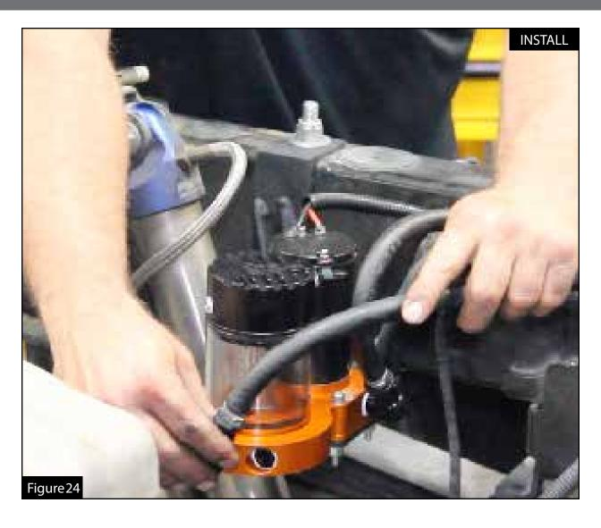
Step 30: Install the supplied outlet fuel line (black "AN" fitting) onto the fuel outlet port of the DFS780.
