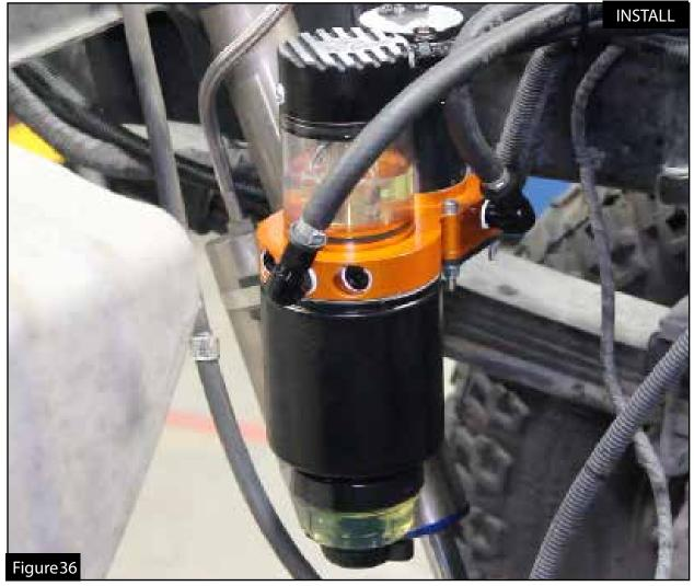
Step 45: Turn the key to the "Run" position and watch to see if the DFS780 fills with fuel. If the DFS780 does not fill with fuel, use the supplied tank valve (on the top of the DFS780) to release trapped air which will allow DFS780 to fill. If DFS780 still does not fill, try starting the engine.
