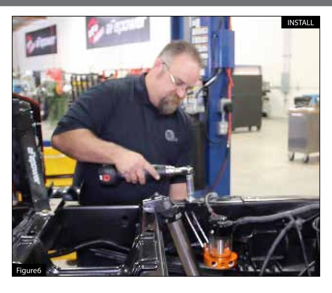
Step 6: Install the other supplied 5/8" washer and 5/8" nut onto the bolt and tighten using a 15/16" wrench and socket.
