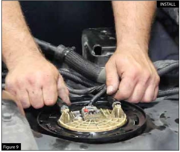
Step 13: Clean area around stock fuel fuel pump sender assembly to prevent dirt from falling into the tank.
