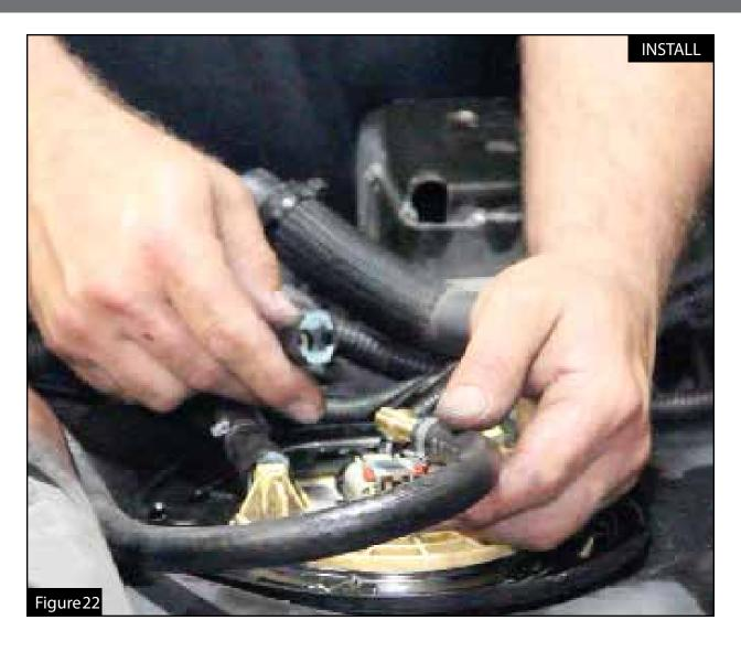
Step 28: Install the 3/8" quick disconnect on the supplied outlet fuel line (with black "AN" fitting) into the quick disconnect fitting on the stock fuel feed line.
