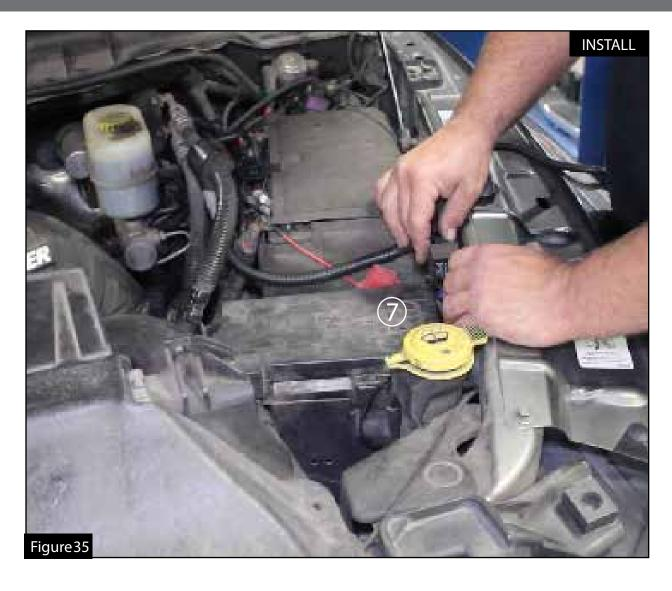
Step 48: Plug the supplied relay harness into the Deutsch connector on the power harness.
