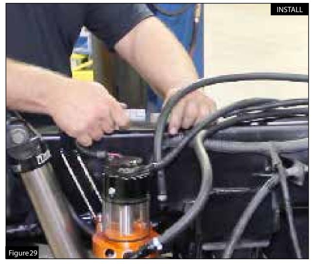
Step 38: Route the supplied wiring harness along the frame.
