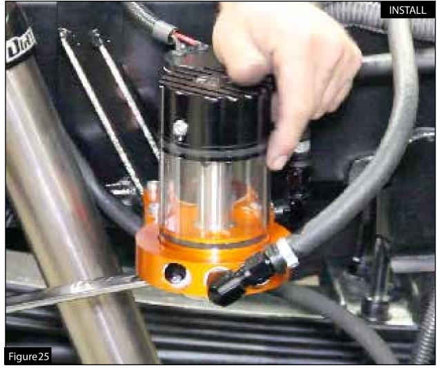
Step 31: Turn sight glass to the desired angle and using a 1-1/4" wrench, tighten the center nut under the DFS780 manifold.
