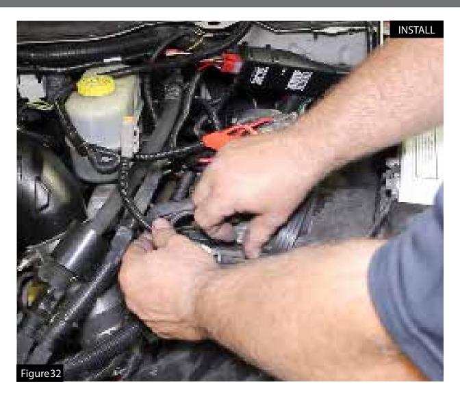
Step 42: Connect the black wire ring terminal to the negative side on the battery.
