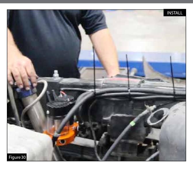
Step 40: Organize the wire harness and fuel lines and secure with the supplied zip ties.
