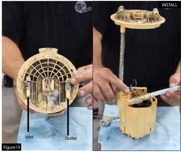
Step 21: Install the 10-1/2" clear tube with the strainer to the outlet of the stock fuel pump sender assembly. Be sure that the supplied clamp is pushed all the way to the top of the tube to prevent leakage.
