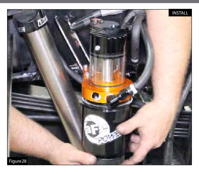
Step 37: Screw the fuel filter assembly onto the manifold and tighten.
