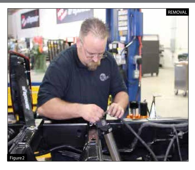
Step 2: Remove the rear differential vent hose from the shock tower.
