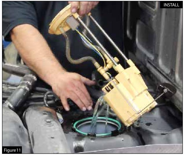
Step 16: Remove the stock fuel pump sender assembly. Be sure to pour out any remaining fuel.
