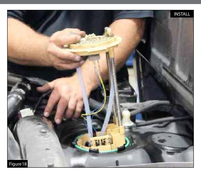
Step 24: Install the fuel pump sender assembly back into the tank.
