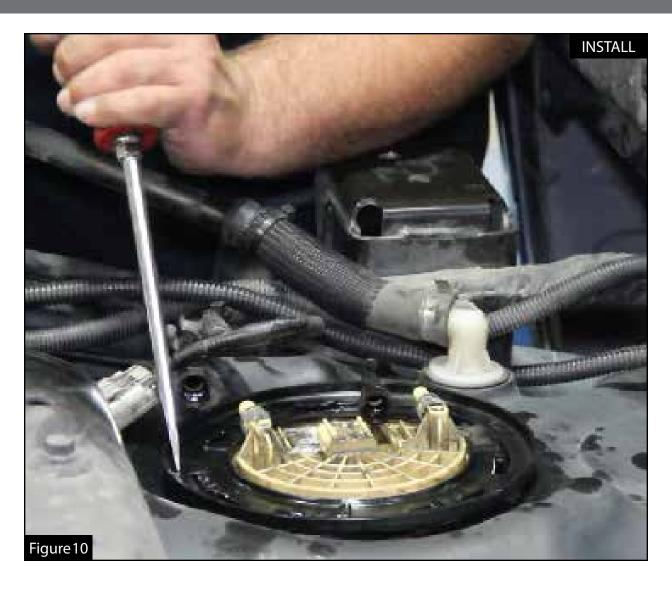
Step 15: Remove the lock ring for the stock fuel pump sender assembly.
