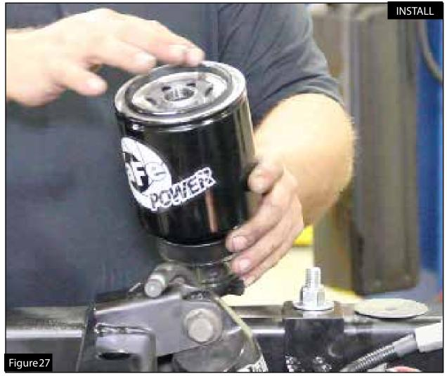
Step 36: Attach supplied water separator bowl onto the supplied fuel filter. Using a light oil, lube the gasket on the fuel filter before installation.
