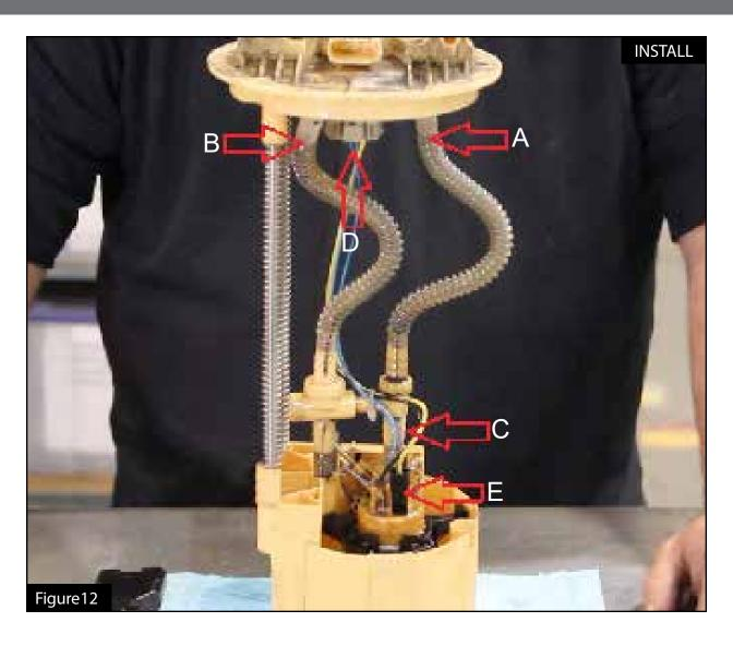
Step 17: Carefully cut the tubing at point A, B, and C. Remove supply tubes from assembly. Step 18: Carefully unplug the harness from points D and E.
