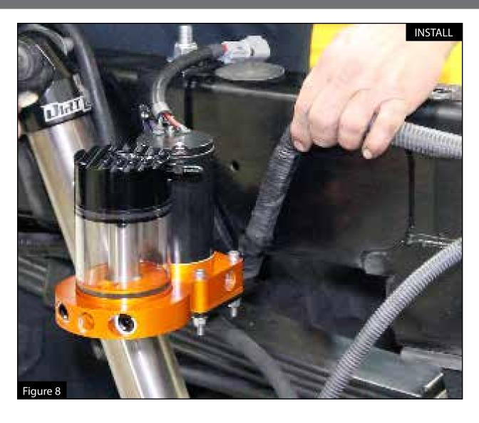
Step 8: Reattach the differential vent tube back onto the shock tower. Reinsert the stock wire harness back into the stock mounting location.
