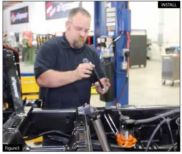
Step 5: Install the supplied 5/8"-11 x 8" bolt, and 5/8" washer through the bottom of the bracket into the factory hole in the frame.
