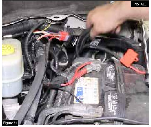
Step 41: Run the remaining wire harness along the frame to the engine compartment. Secure using supplied zip ties.
