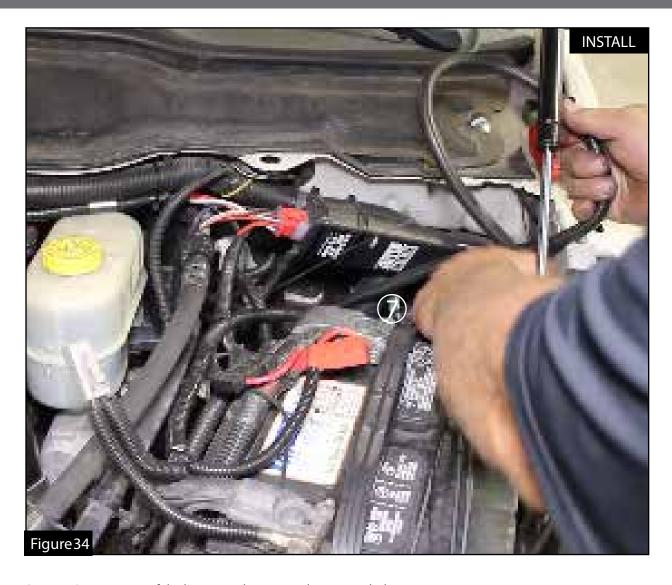
Step 44: Organize any of the loose wire harness and secure with the remaining zip ties.
