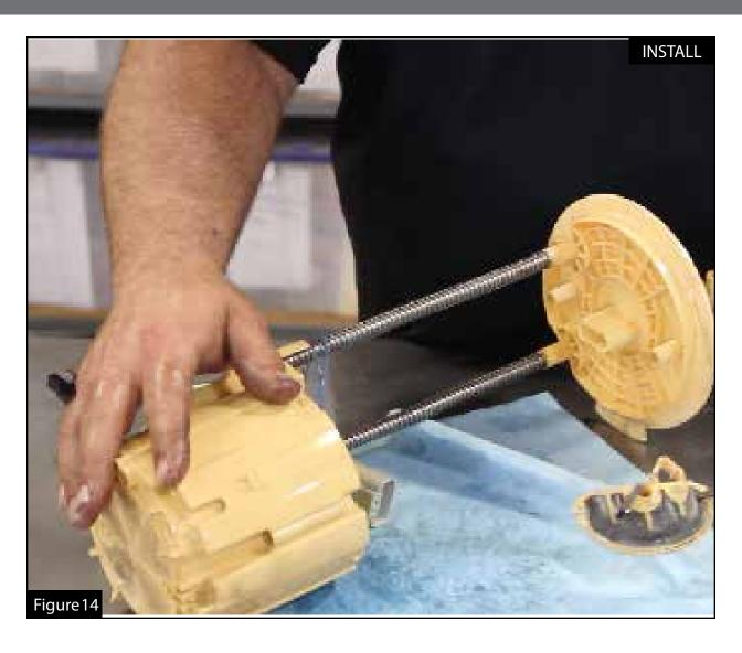
Step 20: Remove both the stock fuel strainer and diverter that are in the bowl.
