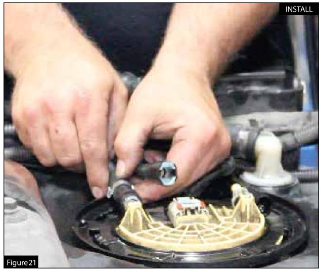
Step 27: Install the supplied fuel line (with silver "AN" fitting) onto the larger (outlet) side of the fuel pump sender assembly.
