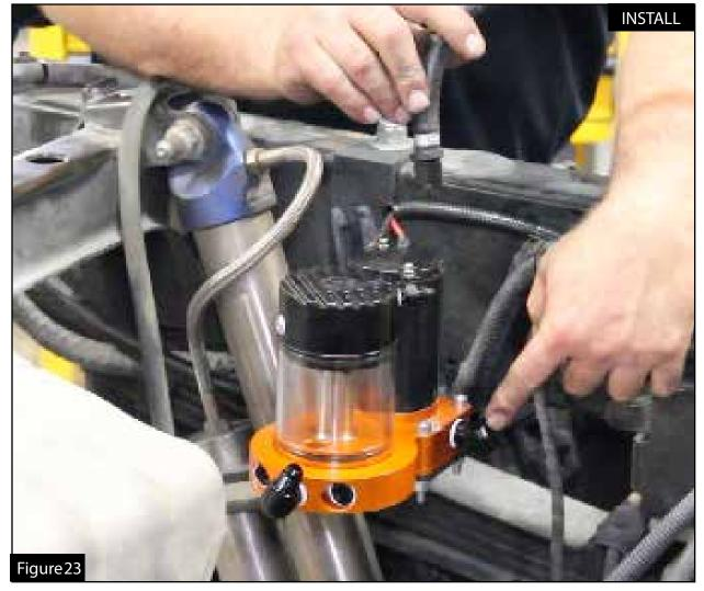
Step 29: Install the supplied inlet fuel line (silver "AN" fitting) onto the fuel inlet port of the DFS780.
