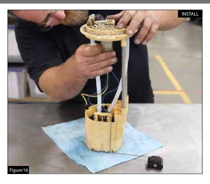
Step 22: Install the 12" clear tube to the inlet side of the pump sender assembly and plug the harness back into the top of the assembly.
