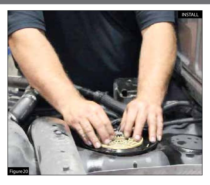
Step 26: Reinstall the stock harness back into the fuel pump sender assebmly.
