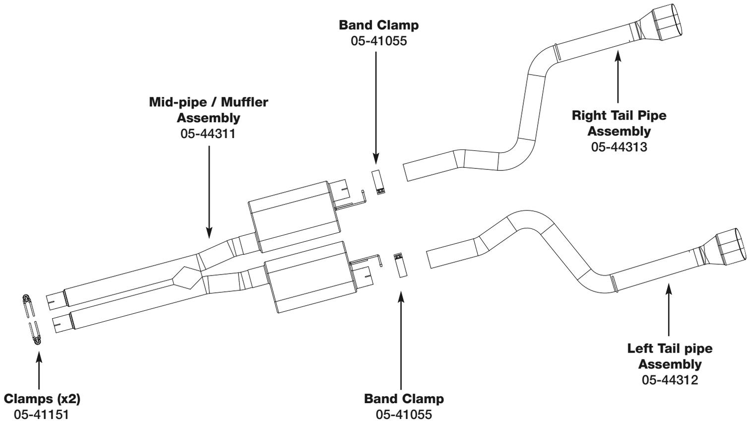
**Step 1: (Read Instructions prior to installation)** Remove your stock exhaust from the rear of your truck working your way forward. Disconnect the ground strap from chassis to muffler and save for re-use later. Also take caution not to damage the factory isolation mounts as they will be reused. **It is recommended to not fully tighten the clamps until the entire system has been installed.**
