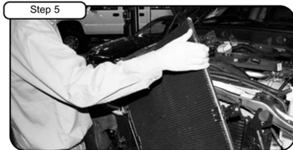
Step 5 Rotate the A/C condensor up and out away from vehicle. Take care to prevent damage to A/C lines.
