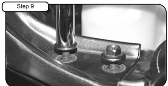
Step 9 Loosen and remove the 4 bolts holding in upper radiator support using 13mm socket or wrench.
