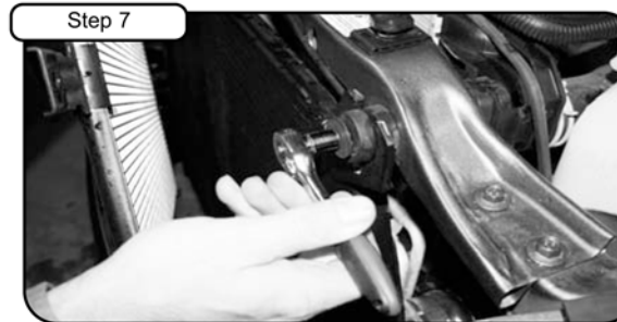
Step 7 With 10mm socket or wrench remove the 2 top intercooler attachment bolts connected to upper radiator support.
