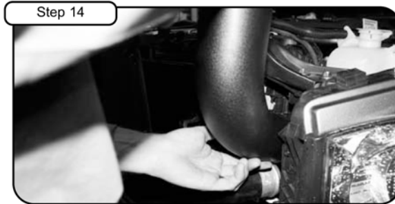
Loosely install new inlet tube to turbo coupler hose. Loosely install new outlet tube to manifold coupler hose.
