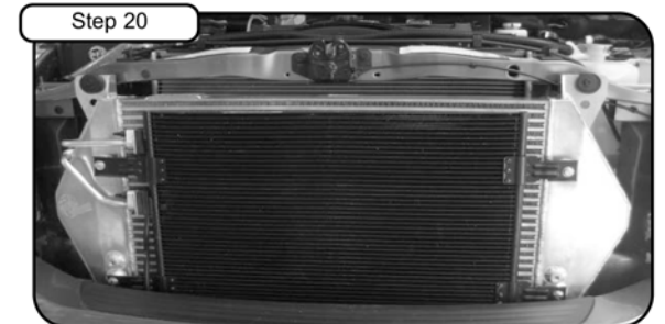
Re-attach A/C line protector (Not shown for photo purposes). Re-install intake/stock air box & re-connect battery. Your installation is now complete. Please check all screws and clamps periodically. Re-tighten if necessary. Thank you for choosing aFePower!
