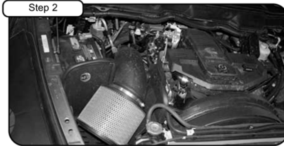
Step 2 Disconnect battery before install. Remove stock air box or intake system from vehicle for easier installation.
