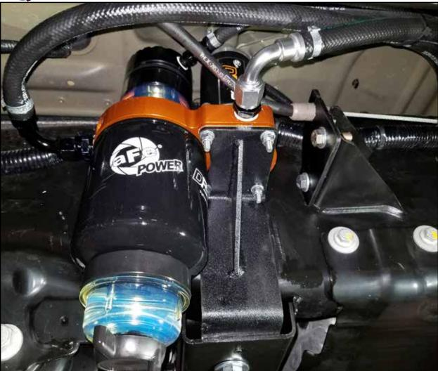
Step 33: Plug the pressure switch harness into the Deutsch connector on the power harness.
