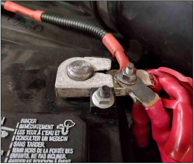
Step 26: Connect the red wire ring terminal on the power harness to the positive side of the battery.
