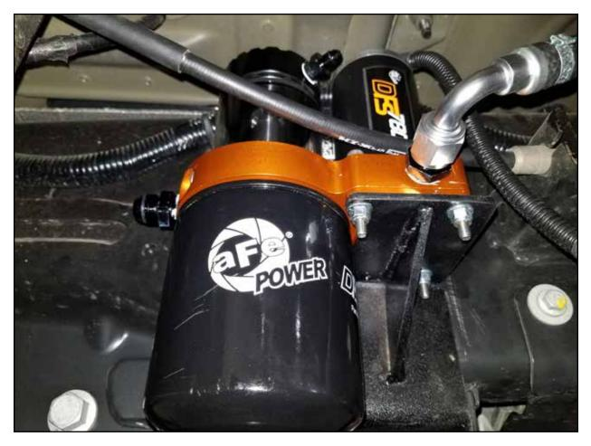
**Step 17:** Install the fuel inlet hose (90° silver -8 AN fitting) onto the male -8 AN fitting on the fuel inlet port of the fuel manifold assembly.
