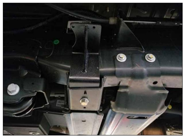
**Step 2:** Mount the supplied bracket to the frame using the supplied 1/2"-13 x 1.50" bolt, and 1/2" washer and tighten.
