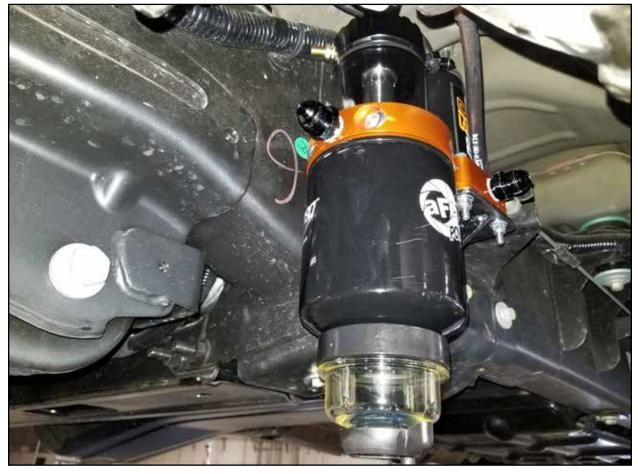
**Step 9:** Using a light oil, lube the gasket on the supplied fuel filter and install on the fuel manifold assembly. Thread the supplied water separator bowl onto the fuel filter.
