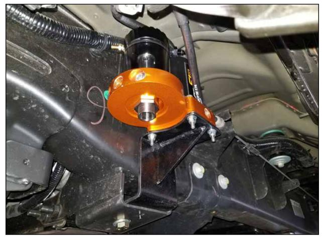
**Step 5:** Mount the supplied fuel manifold assembly to the carbon steel frame bracket using the supplied hardware and tighten.
