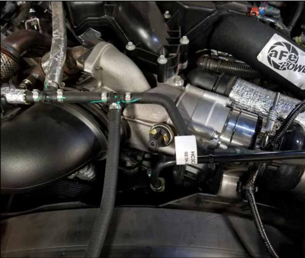
Step 28: Install the supplied pressure switch into the intake manifold (1/8" NPT).
