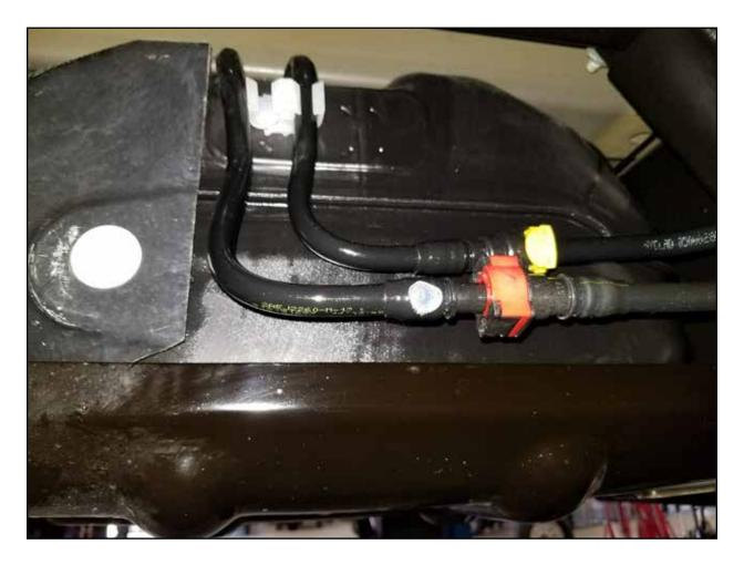
**Step 10:** Clean the area around the stock fuel lines (located on the driver's side, in front of the tank) to prevent dirt and debris from going into the lines.
