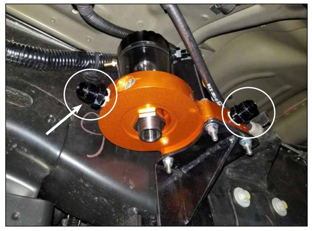
**Step 7:** Install the 2 x 3/8" NPT to -8 AN fitting into the DFS 780 (as shown above).
