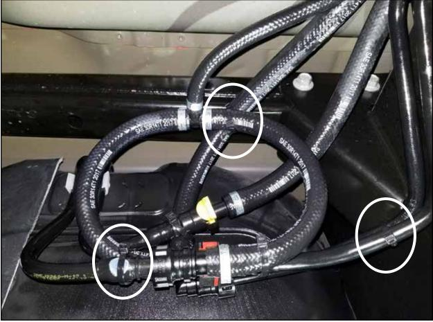
Step 20: Using the supplied nylon cable ties, secure the new hoses (as shown above).
