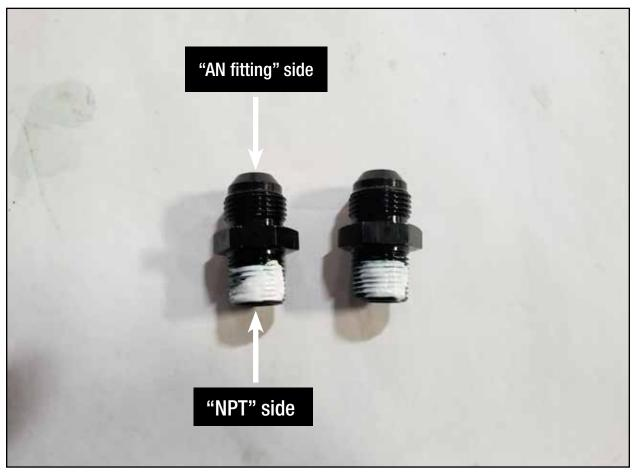
**Step 6:** Apply Teflon tape with PTFE or Teflon paste with PTFE to the 2 x 3/8" NPT to -8 AN fittings.
