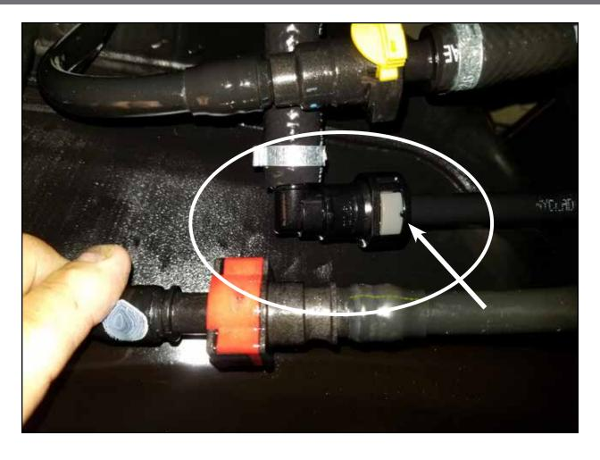
Step 13: Install the 90° female quick disconnect fitting on the supplied fuel outlet hose (black 90° -8 AN fitting - shown below) onto the male side of the stock fuel feed line.
