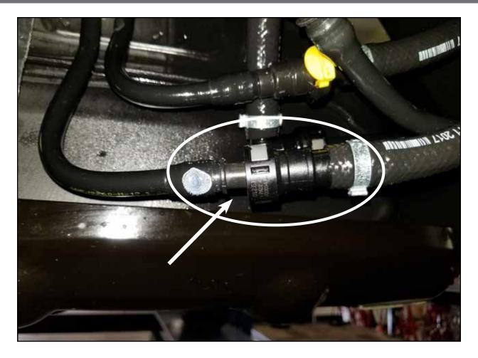
**Step 15:** Install the straight female quick disconnect fitting on the supplied fuel return line (as shown below) onto the male side of the stock return fuel line.
