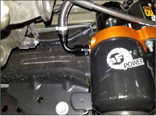
**Step 18:** Install the fuel outlet hose (90° black AN fitting) onto the male -8 AN fitting on the fuel outlet port of the fuel manifold assembly.
