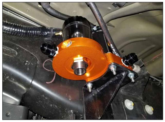
**Step 8:** Turn the sight glass to the desired angle and using a 1-1/4" wrench, tighten the center nut under the fuel manifold assembly.
