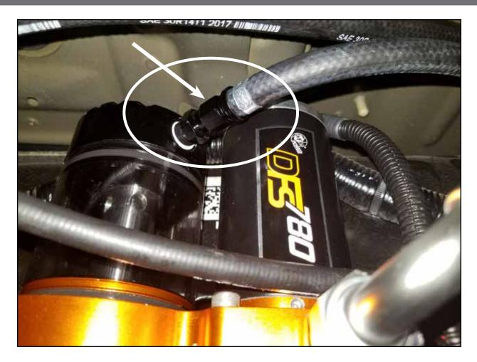
Step 19: Install the supplied fuel return line (-4 AN fitting) onto the top of the sight glass cover.
