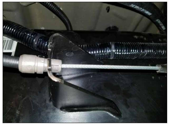
**Step 3:** Remove the parking brake cable from its mount on the frame.
