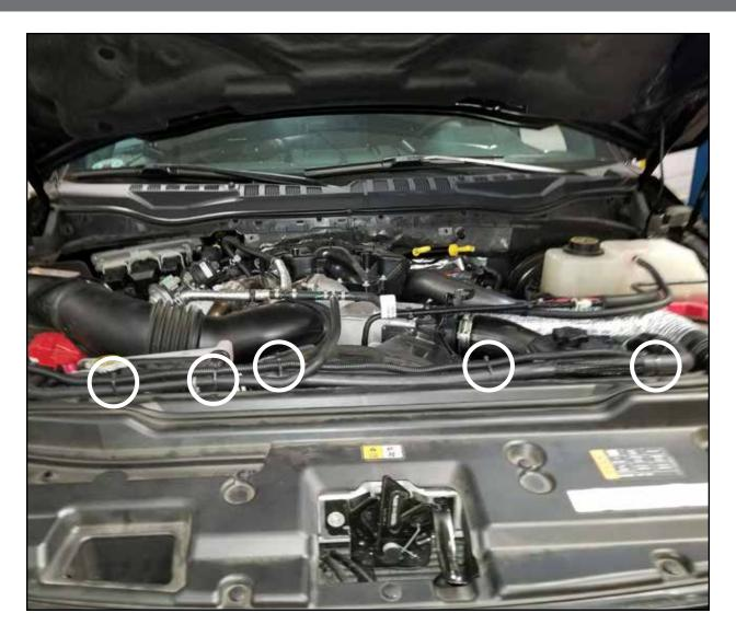
**Step 25:** Run the power harness across the front of the engine compartment using the supplied nylon cable ties to secure the harness.
