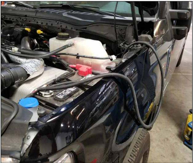
**Step 24:** Run the other end of the power harness along the inside of the frame into the engine compartment.
