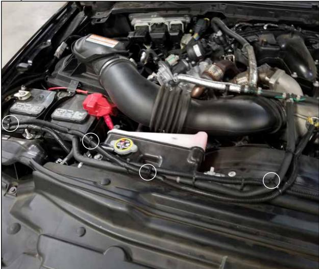
Step 30: Organize any of the loose wire harnesses and secure with the remaining nylon cable ties.
