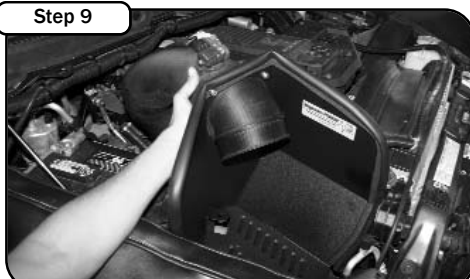
Install new housing with intake tube into vehicle. Position tube and housing to factory position.
