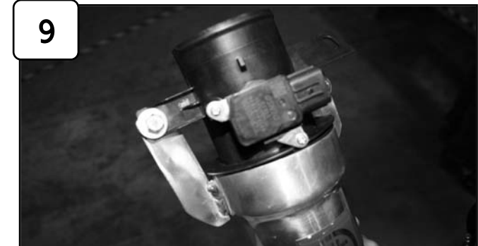
Attach MAF sensor to lower intake tube. Make sure gaskets on sensor are completely inside of tube. With provided M6 screw, nut, wavy and flat washers, secure tabs on sensor to intake tube. Tighten using 10mm socket or wrench.
