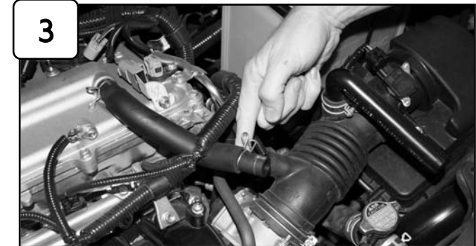
Disconnect MAF sensor harness. Loosen clamps using 10mm socket or wrench. Pull crank case line away from tube.
