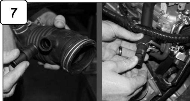
Remove factory crank case fitting from stock tube and re-install.
