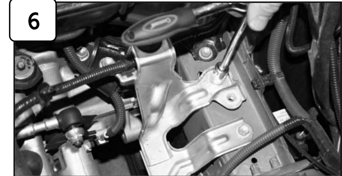
With 12mm socket or wrench, loosen air box bracket and remove.
