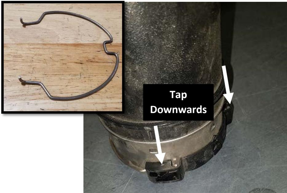
17. Stand the factory intercooler tube up on the end with the metal adapter.
