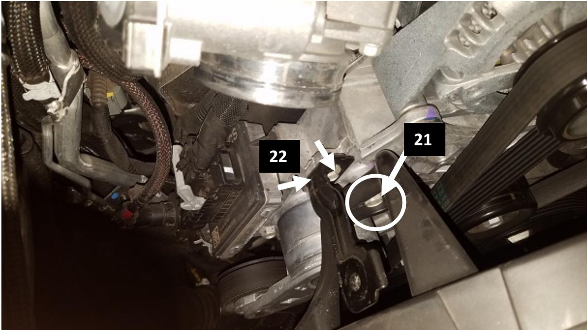
21. Remove the bolt securing the fan shroud to the engine directly behind the intercooler tube mounting bracket, using a 13mm socket.
