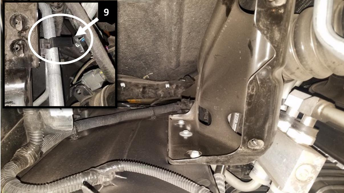
7. Remove the four bolts securing the air box mount to the support bracket, using a 10mm socket.
