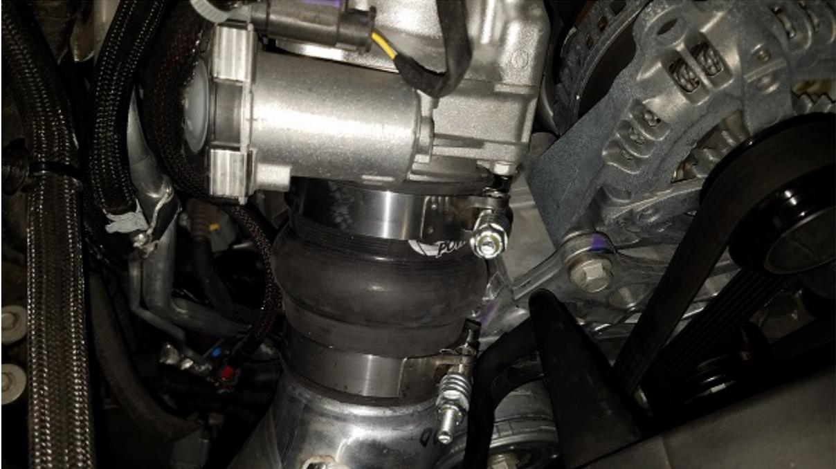
29. Place the 3.38" clamp onto the coupling and connect the coupling to the engine.
