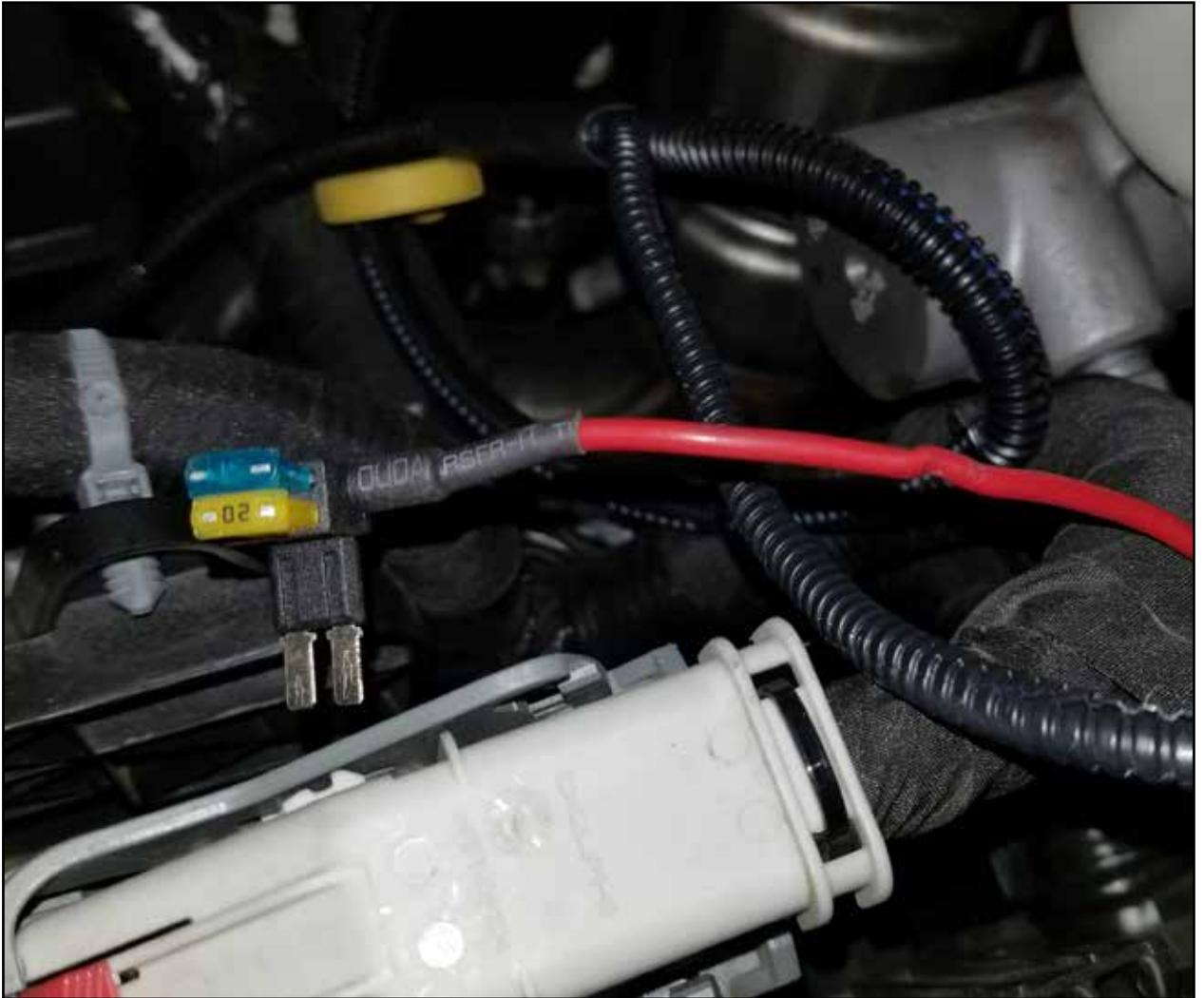
**Step 39:** Install the fuse removed in Step 38 into the open location on the add a harness fuse adapter (not in line with the wire).
