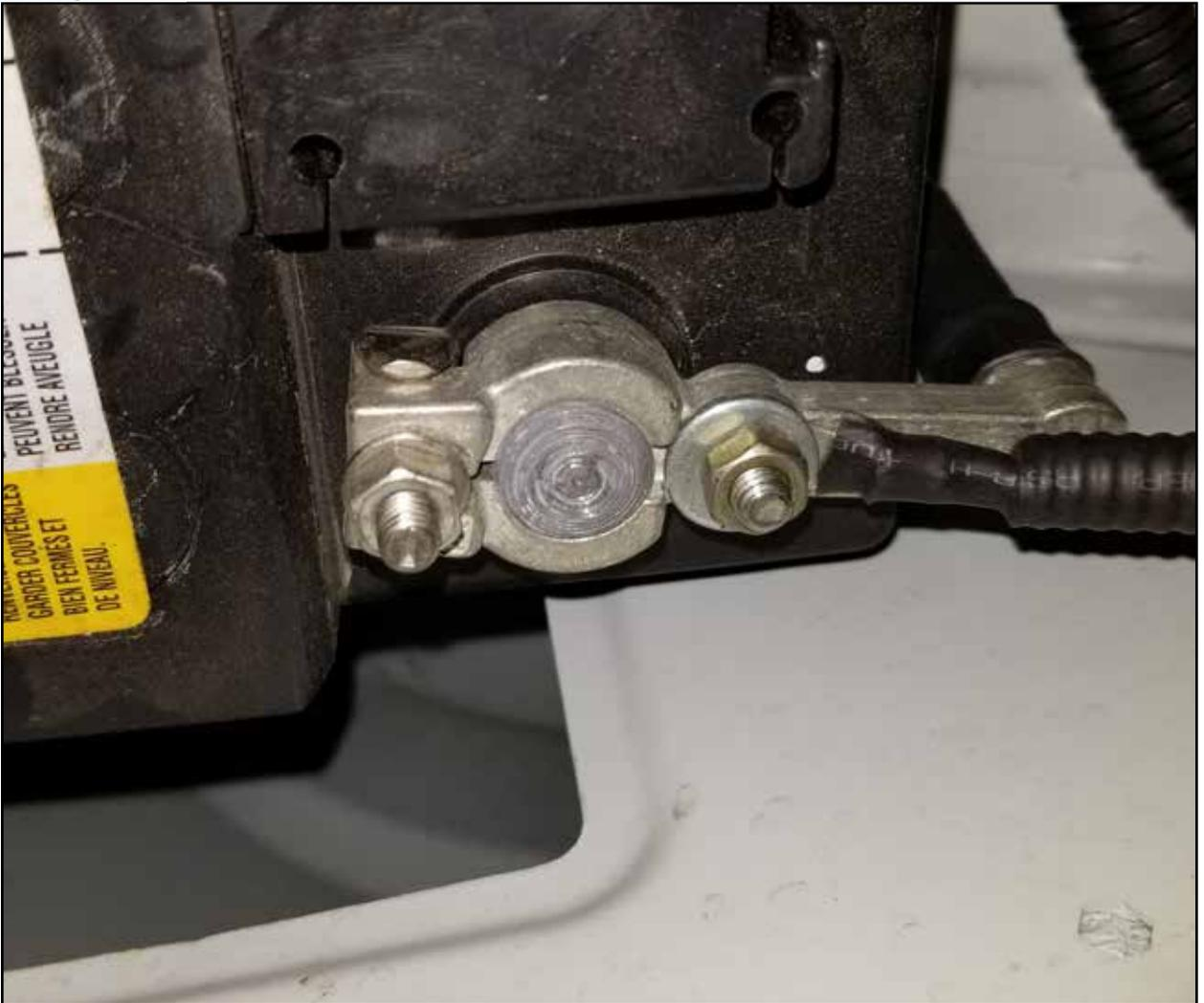
**Step 33:** Connect the black wire ring terminal on the power harness to the negative side of the battery.
