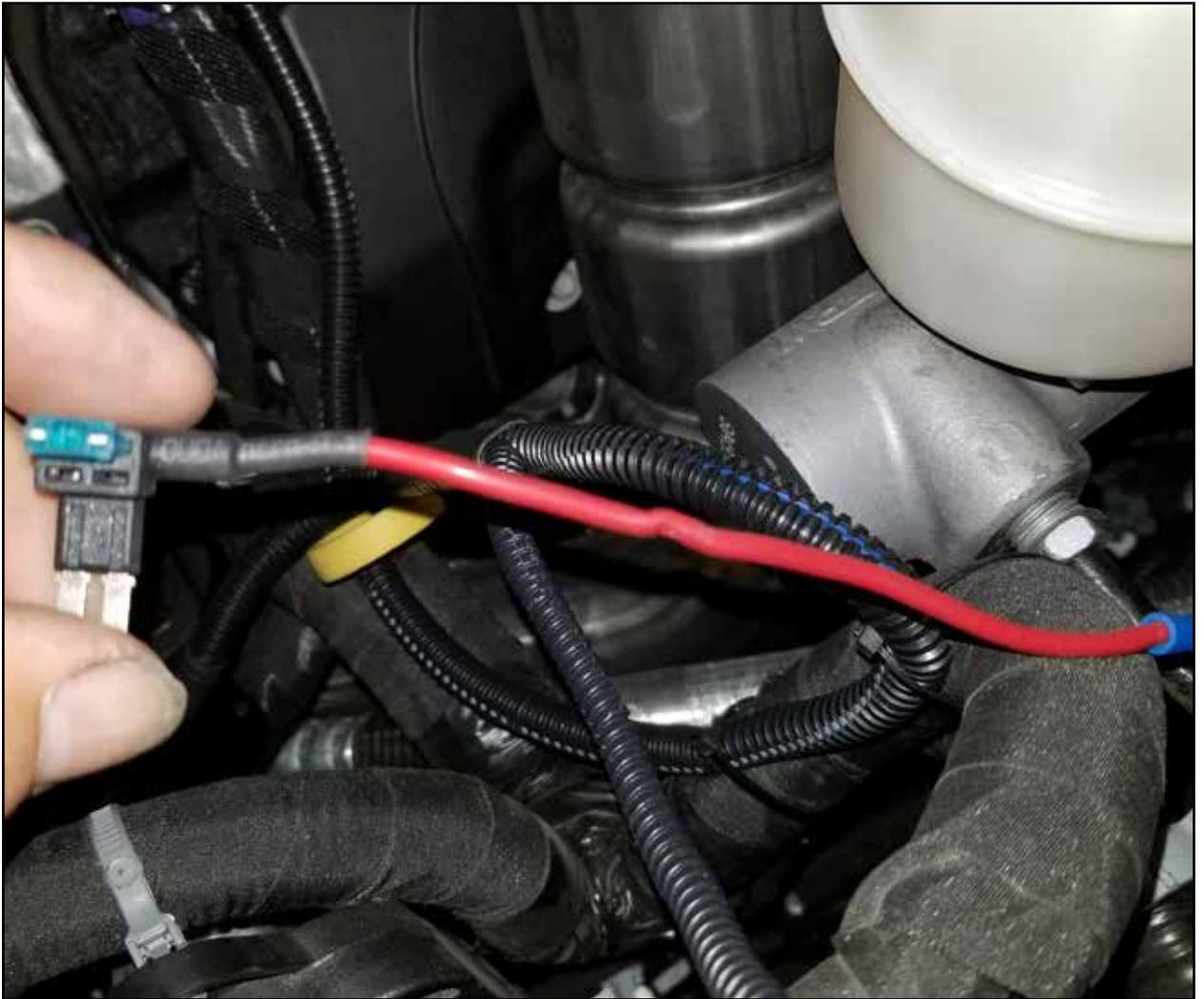
**Step 36:** Attach the power wire from the relay harness to the add a harness fuse adapter.
