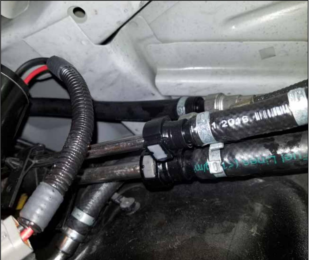
**Step 19:** Install the straight male quick disconnect fitting on the supplied fuel return hose (shown below) into the female side of the stock fuel return line.
