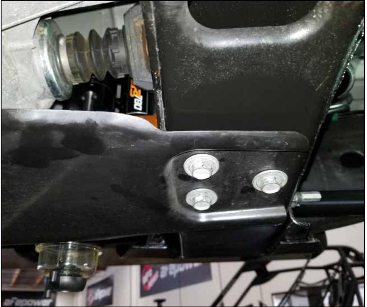
**Step 27:** Reinstall the factory transfer case skid plate using factory hardware.
