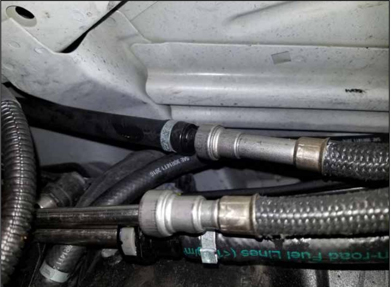
**Step 16:** Install the male quick disconnect fitting on the supplied fuel outlet hose (black 90° -8 AN fitting shown below) into the female side of the stock fuel feed line.
