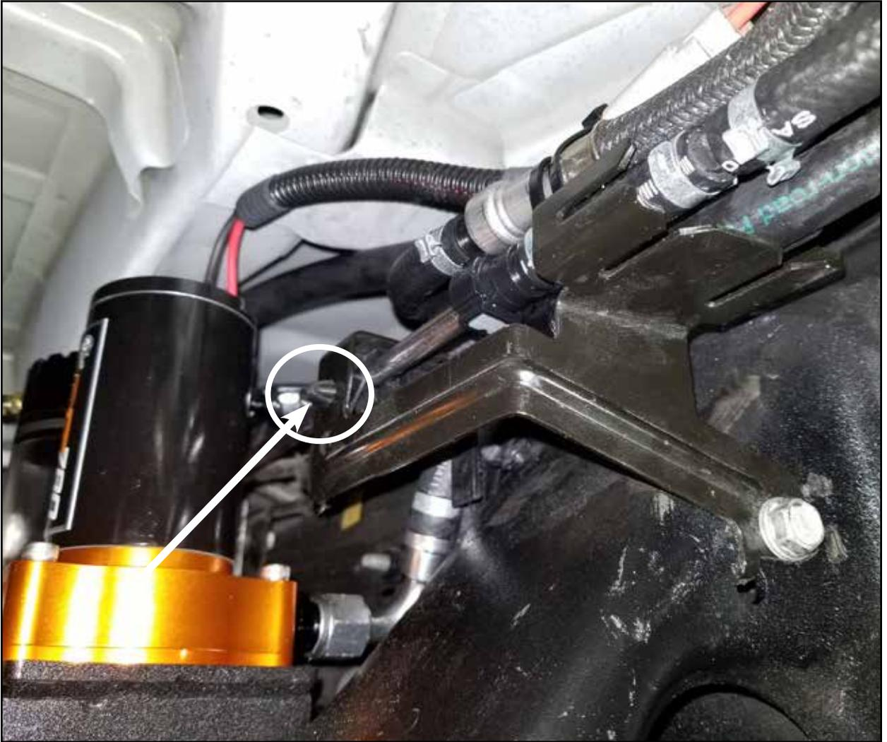
**Step 22:** Reinstall the factory fuel line retainer bracket.
