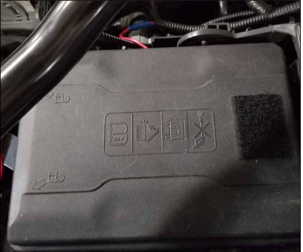
**Step 41:** Carefully route the power wire outside the fuse box and reinstall the cover (making sure not to pinch the wire).
