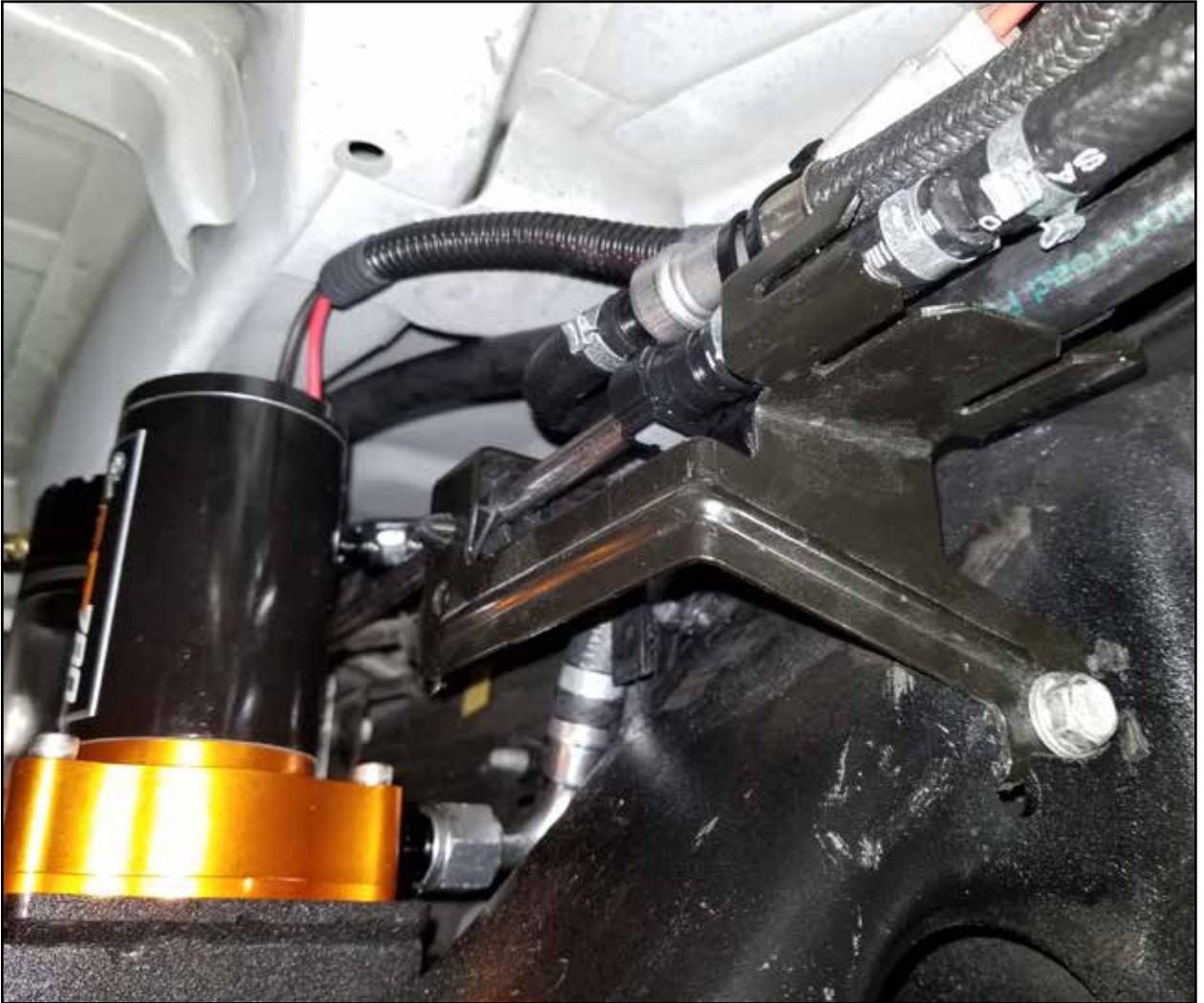
**Step 28:** From the inside of the frame, plug the Deutsch connector on the supplied power harness into the mating connector on the fuel pump motor.
