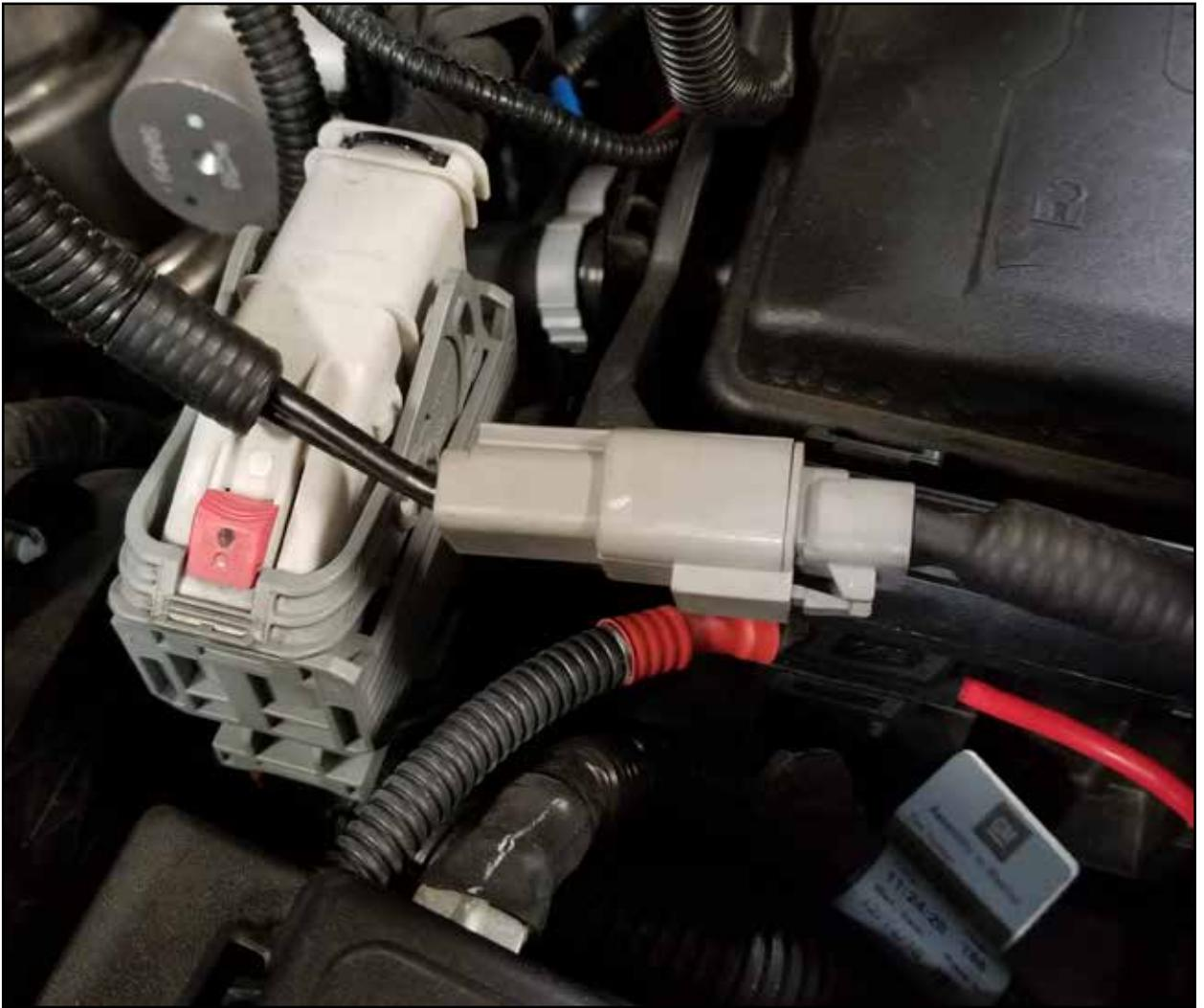
**Step 34:** Plug the supplied relay harness into the Deutsch connector on the power harness.
