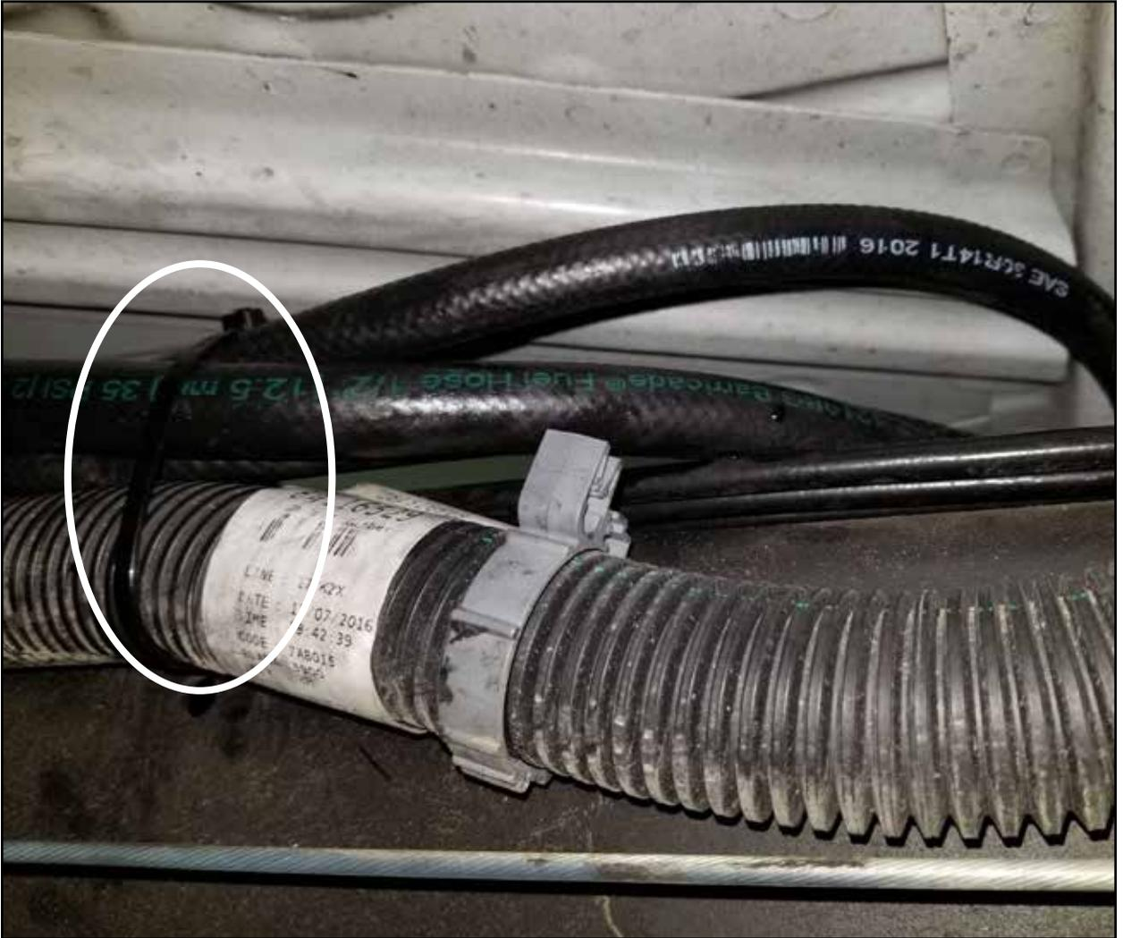
**Step 25:** Using the supplied nylon cable ties, secure the new hoses (as shown above).
