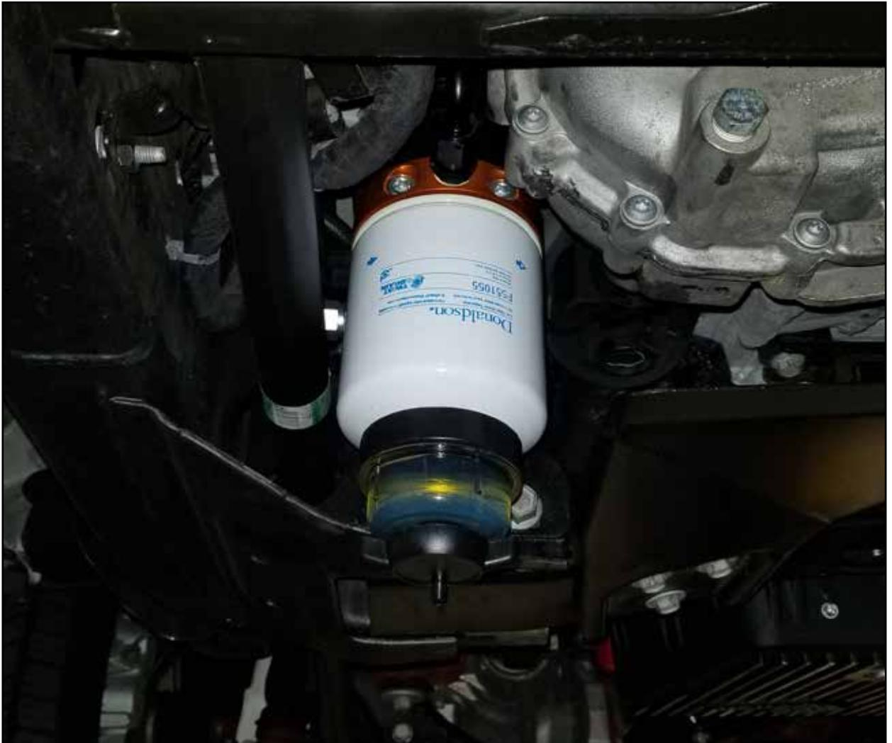
**Step 43:** Turn the key to the “Run” position and watch to see if the sight glass fills with fuel. If the sight glass does not fill with fuel, use the tank valve (on the top of the sight glass cover) to release any trapped air. If the sight glass still does not fill, try starting the engine.
