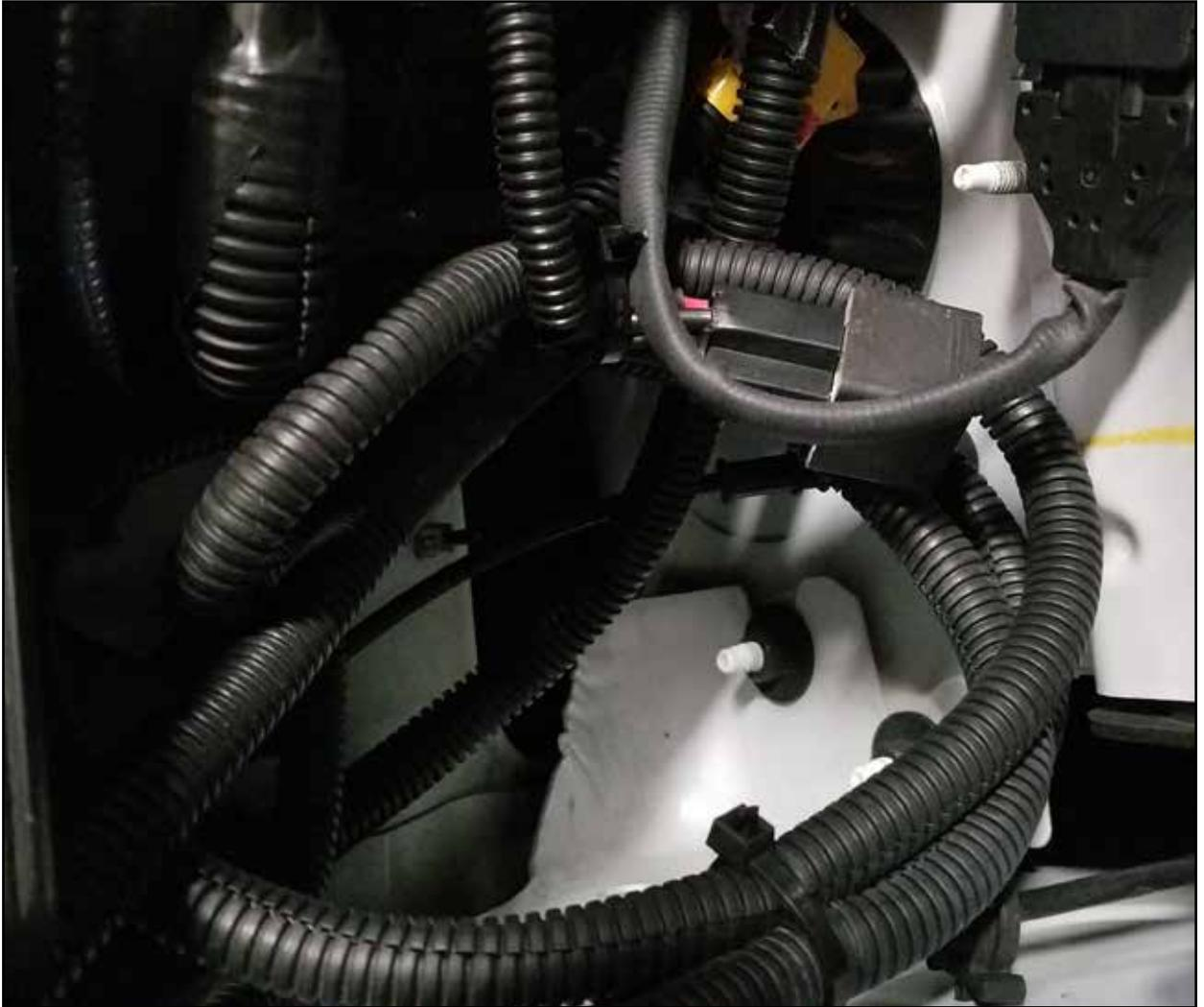
**Step 35:** Secure the relay harness using a supplied cable tie.
