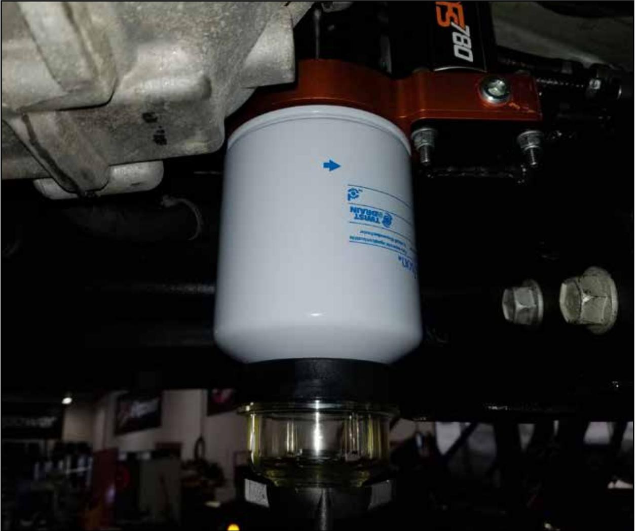
**Step 26:** Using a light oil, lube the gasket on the supplied fuel filter and install on the fuel manifold assembly. Thread the supplied water separator bowl into the fuel filter.
