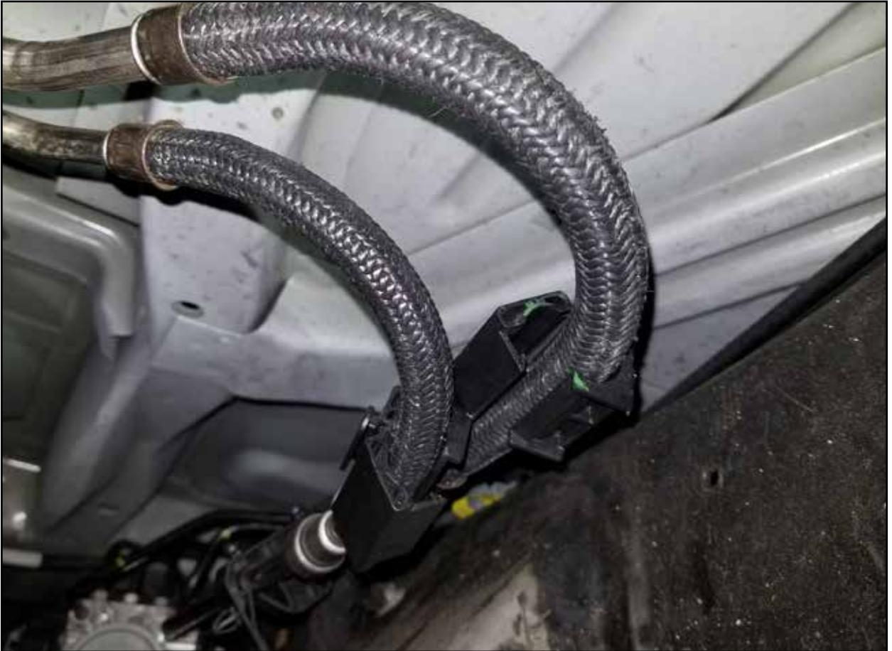
**Step 5:** Remove the fuel lines from the factory bracket and remove the black line holders from the factory fuel lines (shown above).
