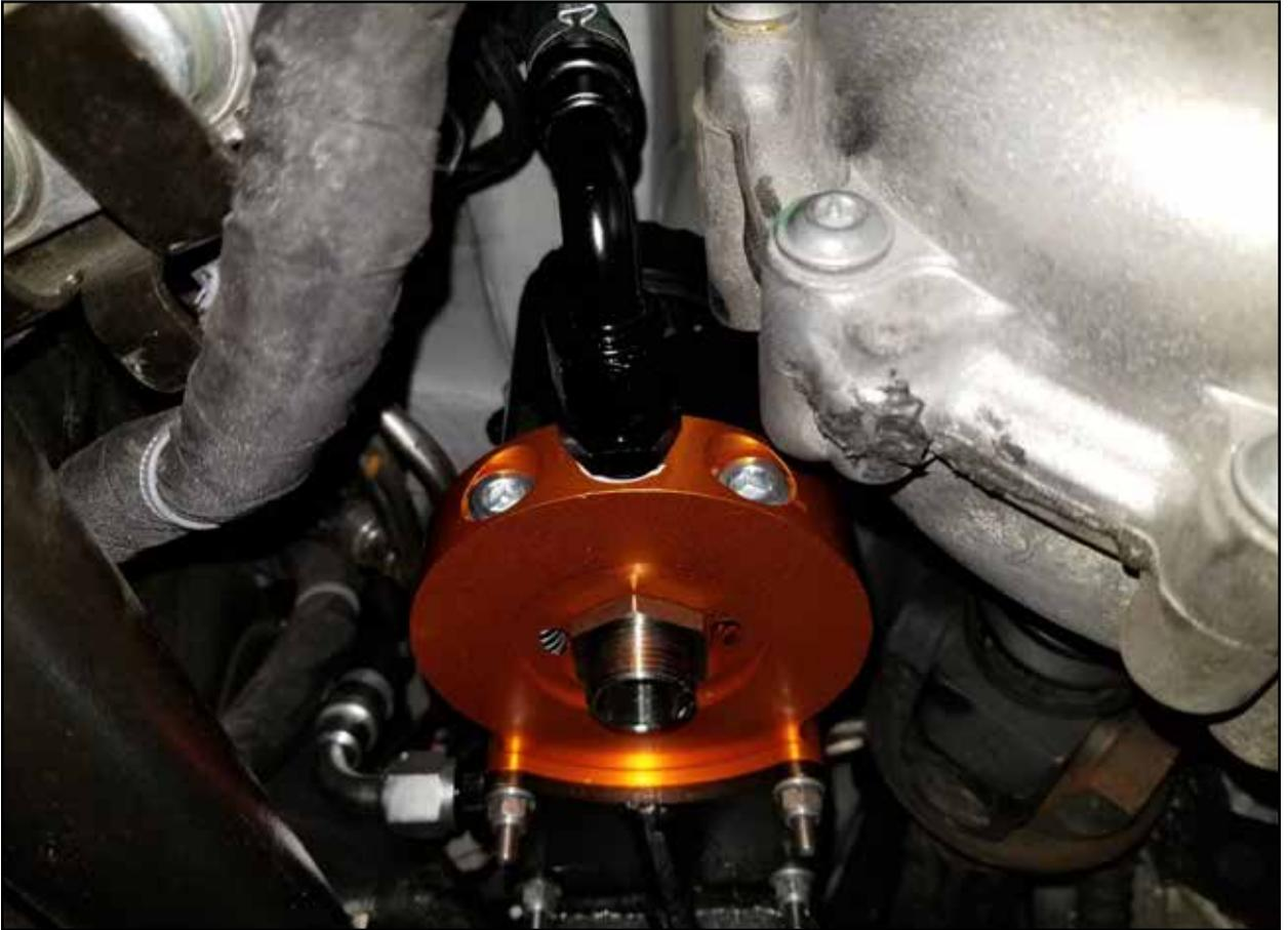
**Step 13:** Install the fuel outlet hose (black 90° -8 AN fitting) onto the male -8 AN fitting on the fuel outlet port of the fuel manifold assembly.
