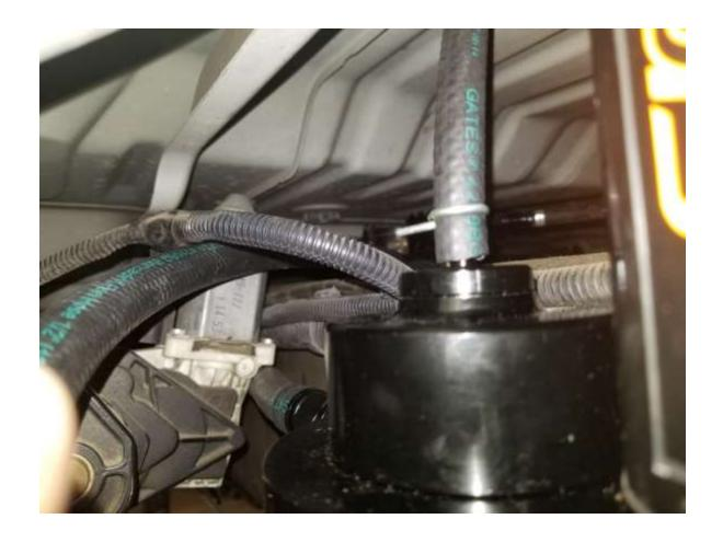
23. Carefully route the ½" hose to the top of the air chamber on the fuel manifold assembly, making sure not to kink the hose or allow it near moving parts. Carefully mark and then cut the hose to the correct length. Using the supplied spring clamp, attach the hose to the nipple on the top of the air chamber on the fuel manifold assembly.
