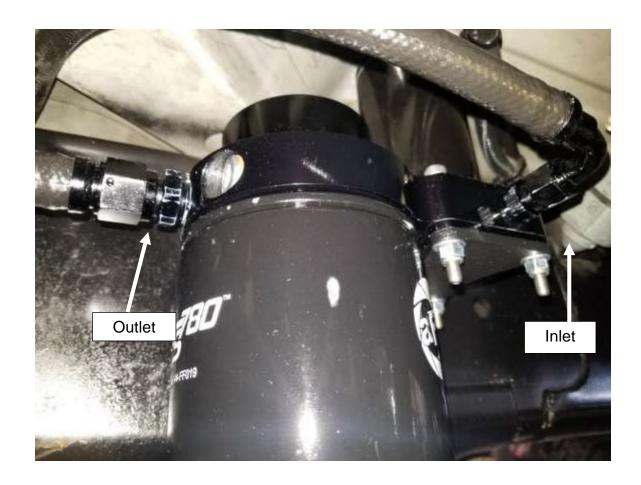
21. Attach the fittings to the inlet & outlet ports of the fuel manifold assembly. Make sure all connections are tight.
