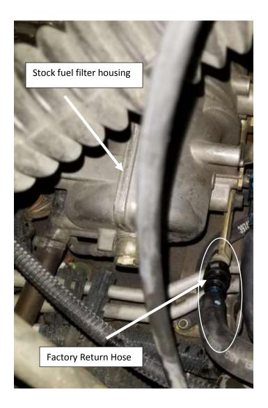
22. Disconnect the factory fuel return line. Attach the supplied fuel return hose between the male and female factory fuel fittings. Push all connections togethers.
