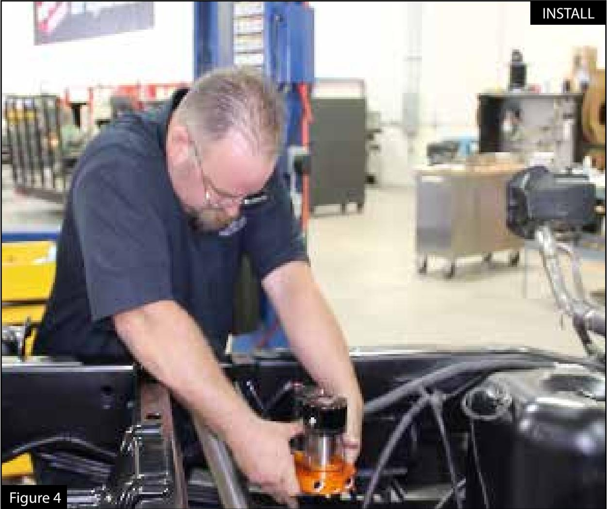
Step 4: Install the bracket onto the frame.
