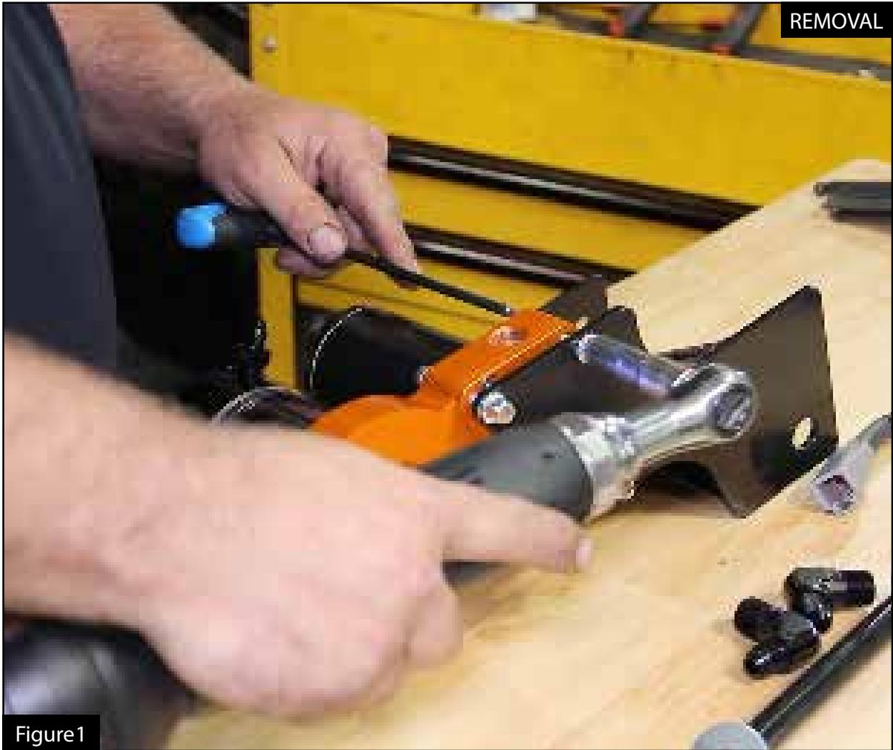
Step 1: Connect the bracket to the manifold using the four (4) supplied M6x1.0 x 50mm bolts, M6 washers and M6 flange nuts.
