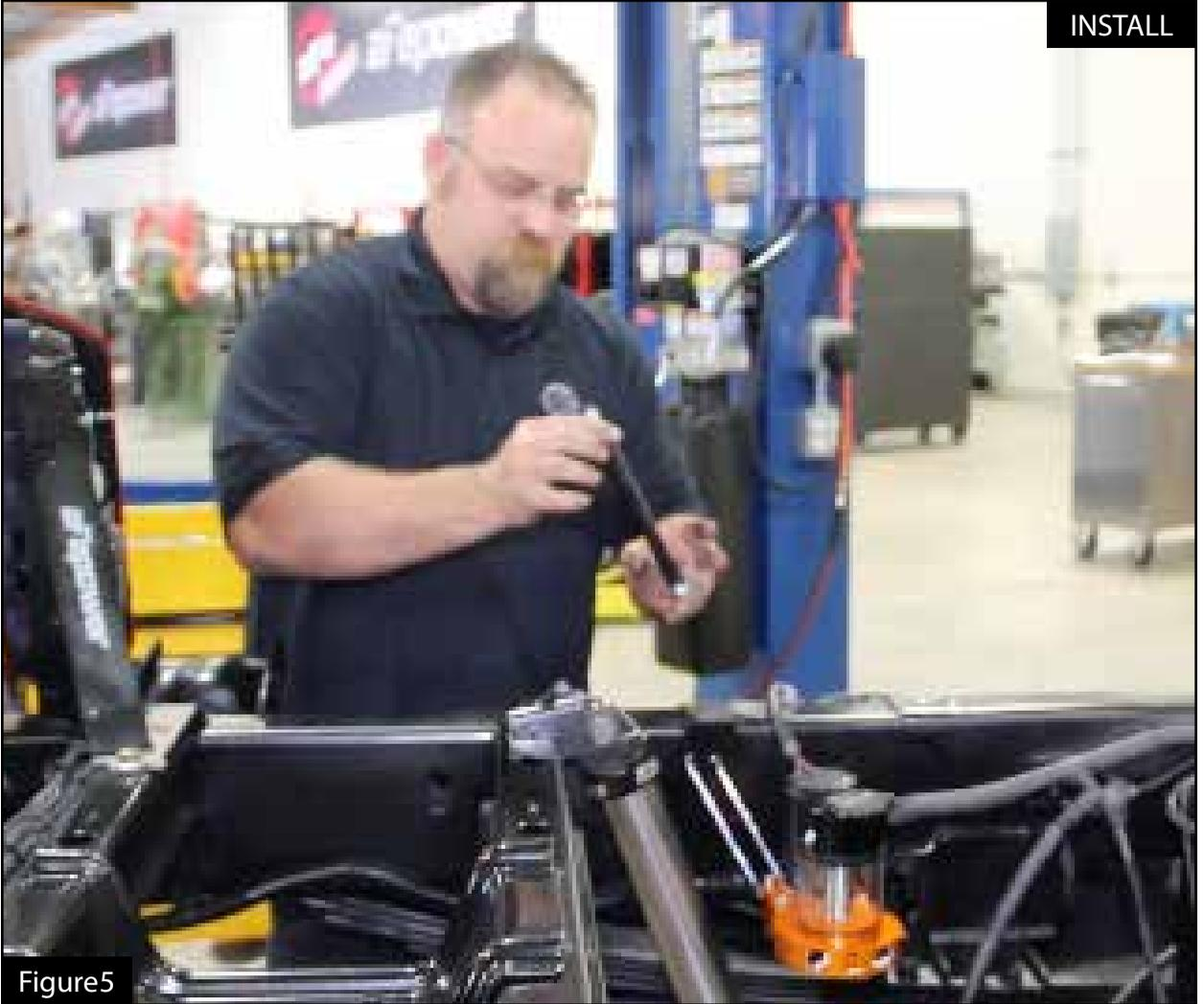
Step 5: Install the supplied 5/8"-11 x 8" bolt, and 5/8" washer through the bottom of the bracket into the factory hole in the frame.
