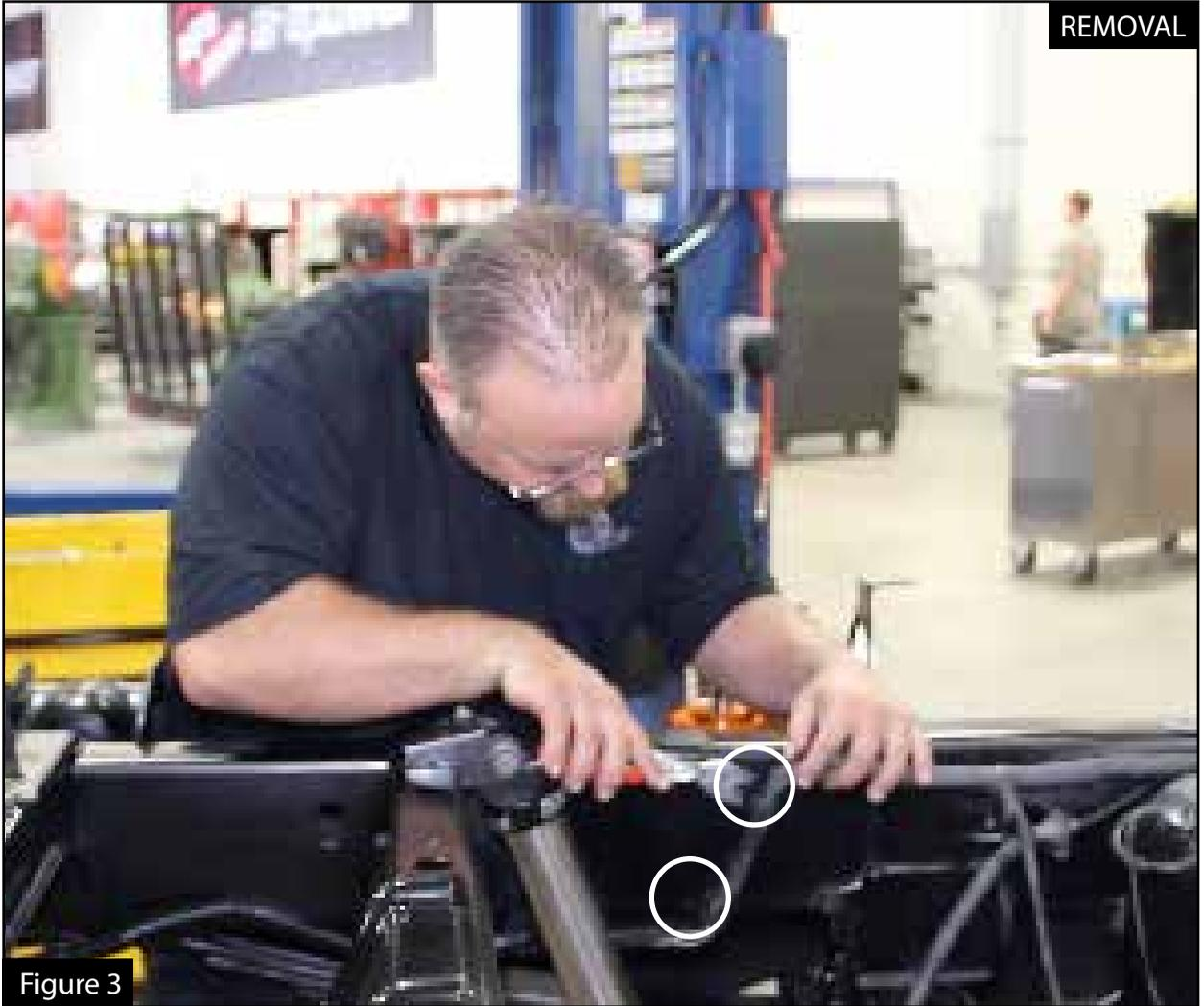
Step 3: Remove the factory wire harness from the two mounting holes. (As circled above)
