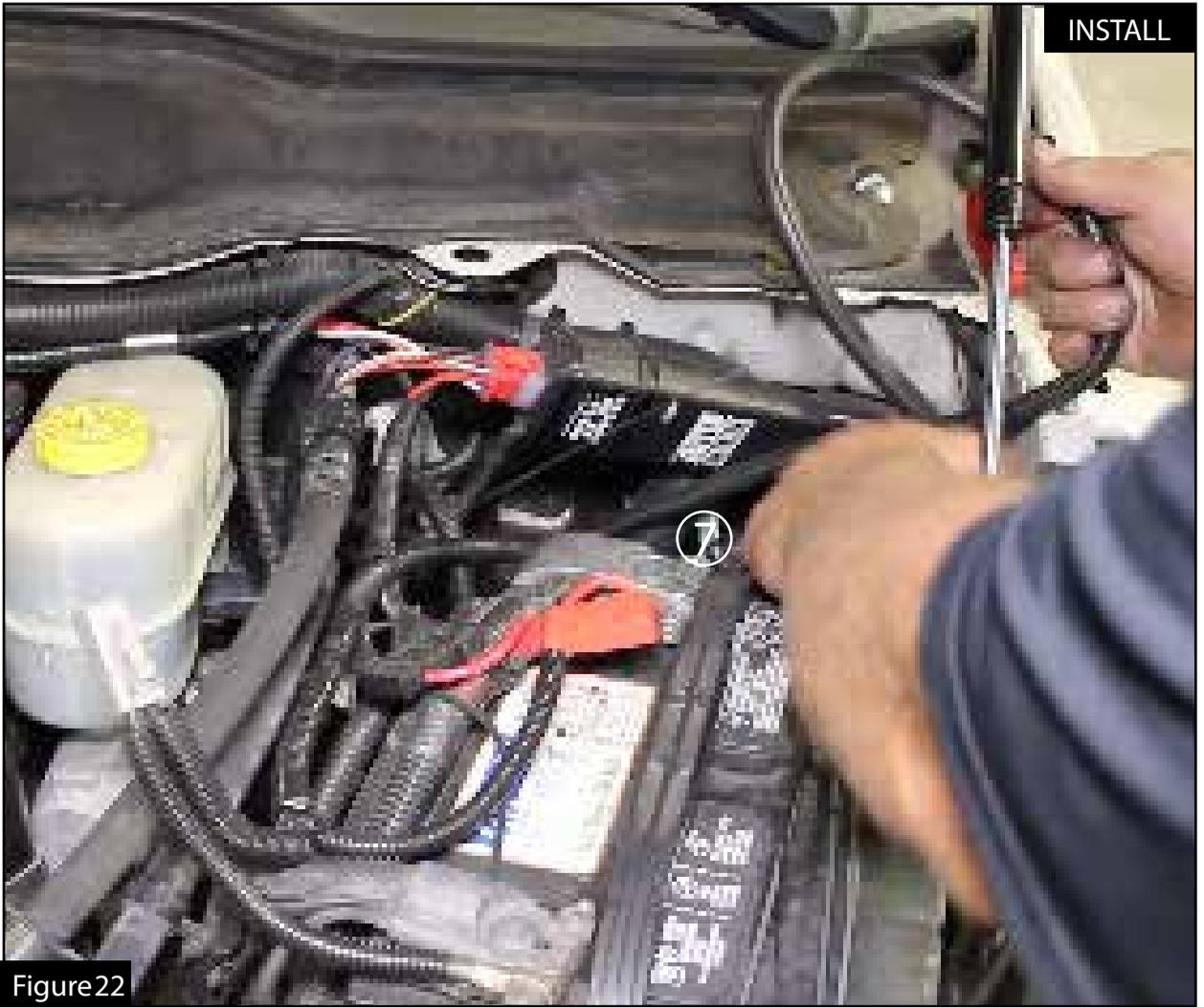
Step 27: Organize any of the loose wire harness and secure with the remaining zip ties.
