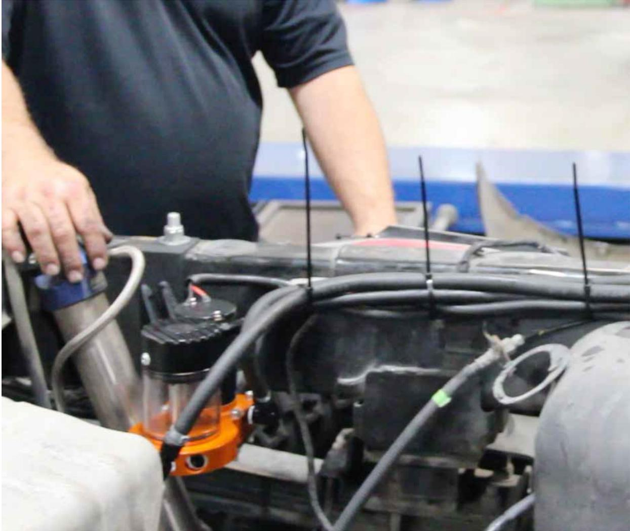
24. Organize the wire harness and fuel lines and secure with the supplied nylon cable ties.
