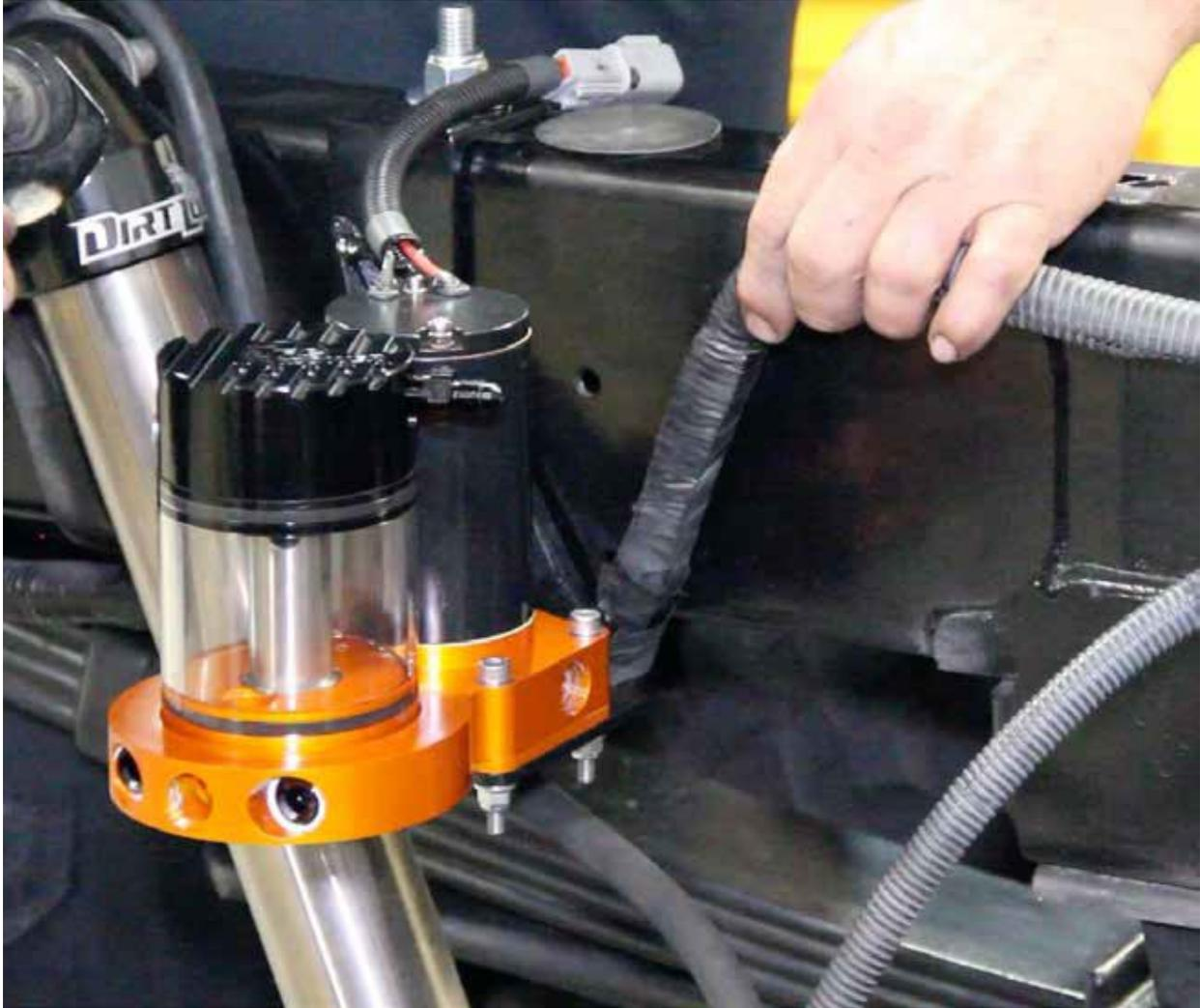
8. Reattach the differential vent tube back onto the shock tower.
