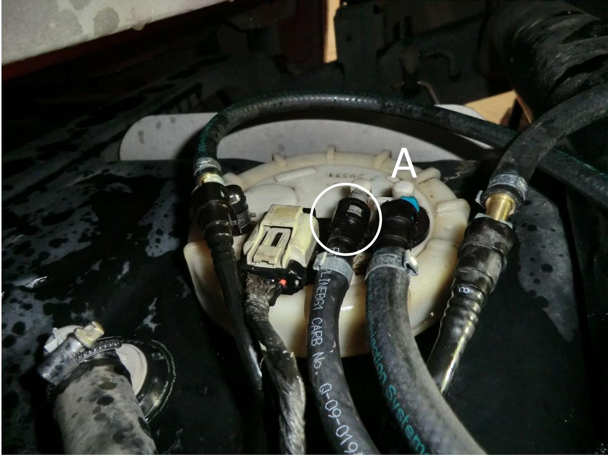
14. Install the female side of the supplied return line to the male connection on the stock fuel tank connection (as shown below).
