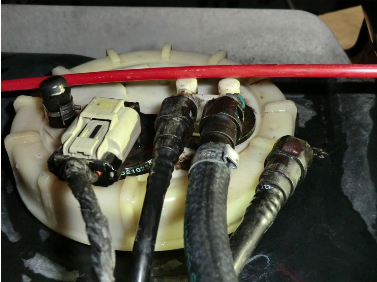
12. Install the supplied fuel inlet hose (with silver “AN” fitting) onto the male side of the stock fuel line (shown below).
