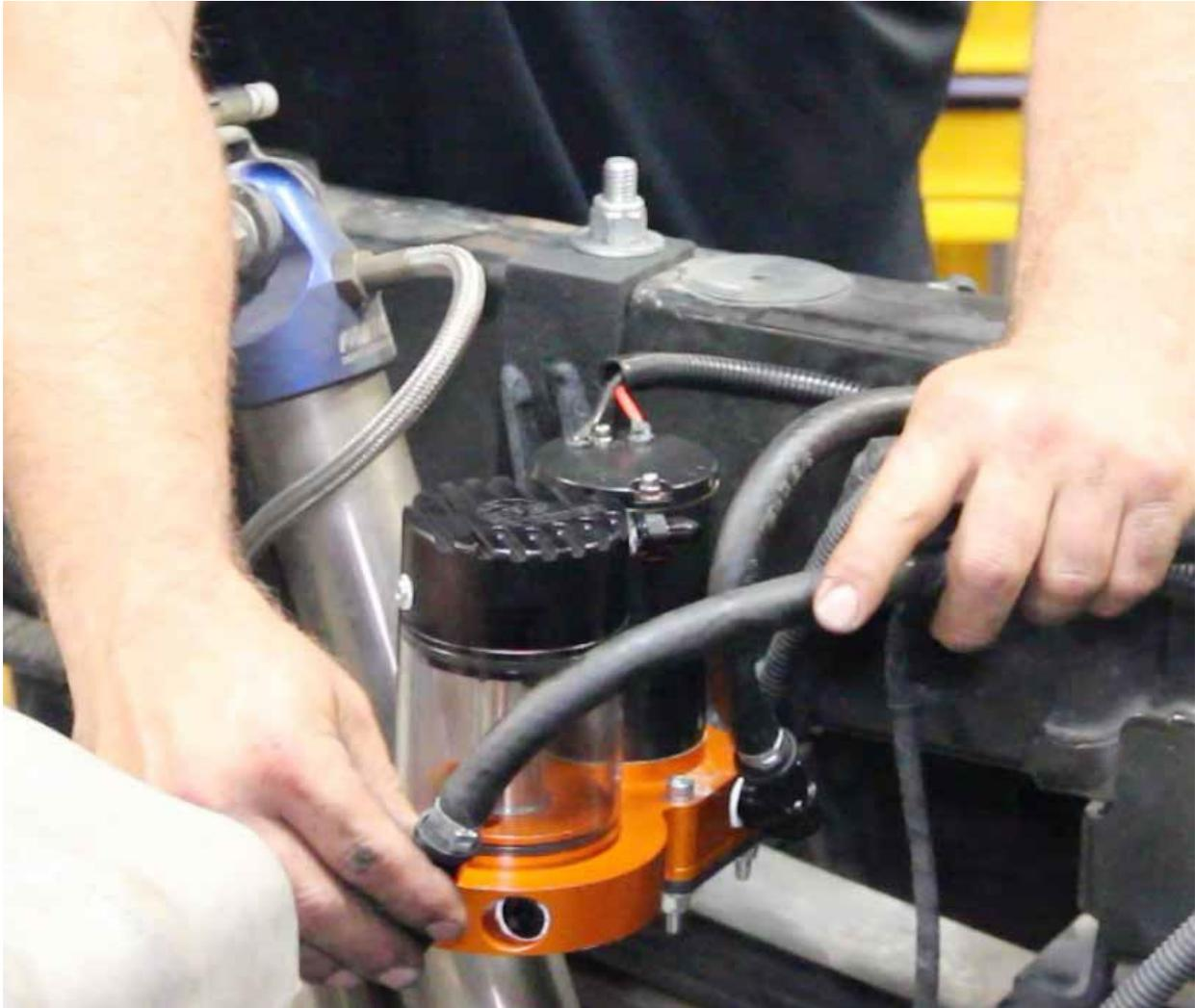
17. Install the fuel outlet hose (black "AN" fitting) onto the fuel outlet port of the DFS780.
