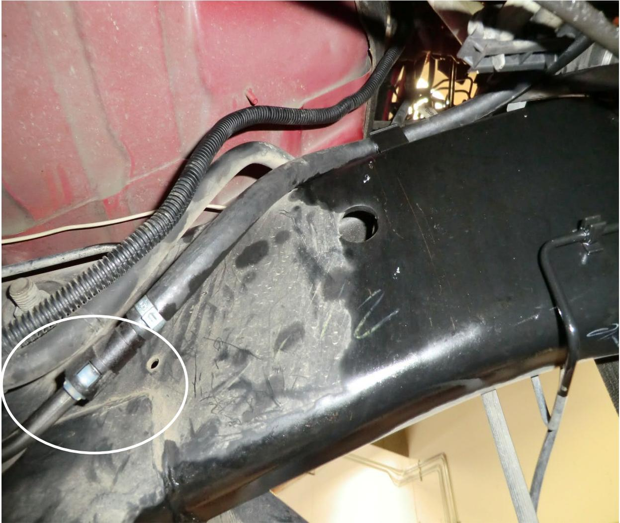
29. Attach the new aFe fuel supply hose to the factory fuel line (shown below).
