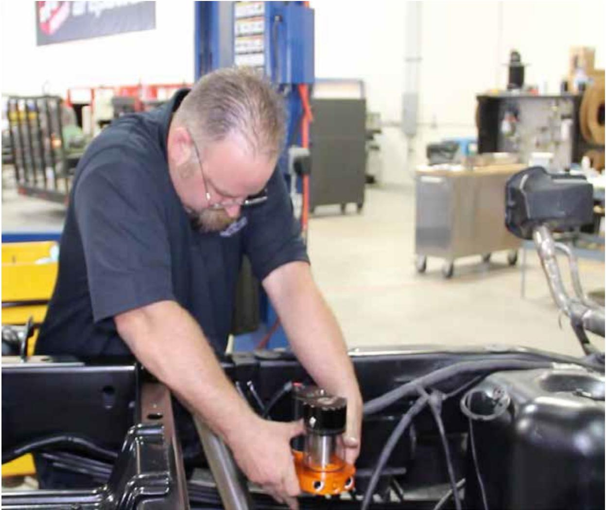
5. Install the carbon steel frame bracket onto the frame.
