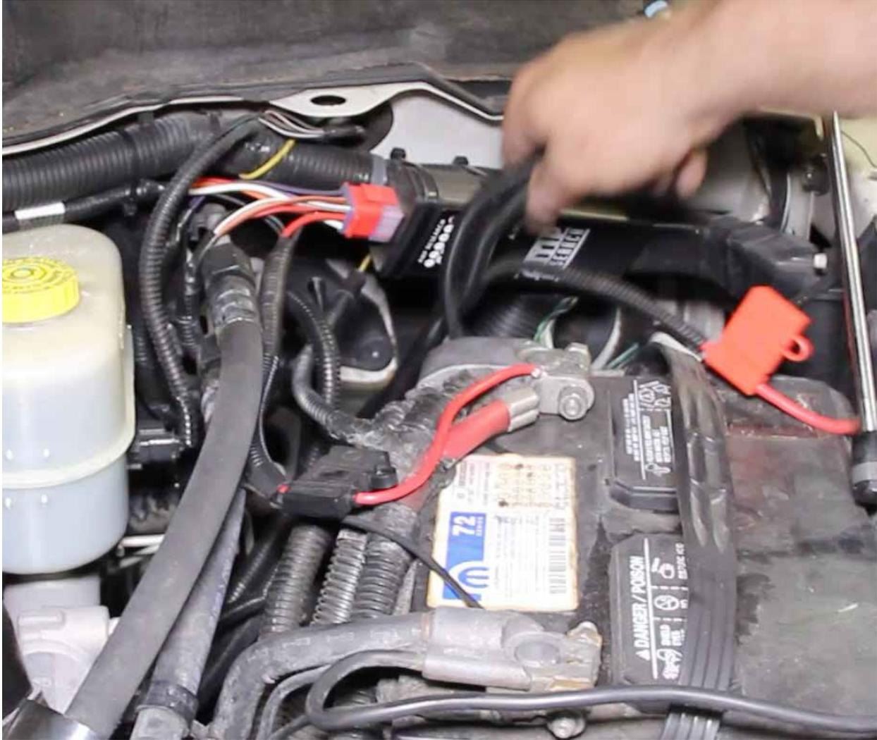
30. Run the remaining wire harness along the frame to the engine compartment.
