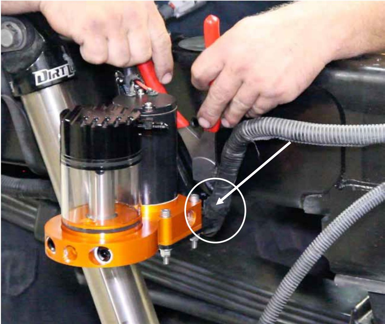
7. Remove (cut off) the lower plastic mounting tab on the stock wire harness (shown above).
