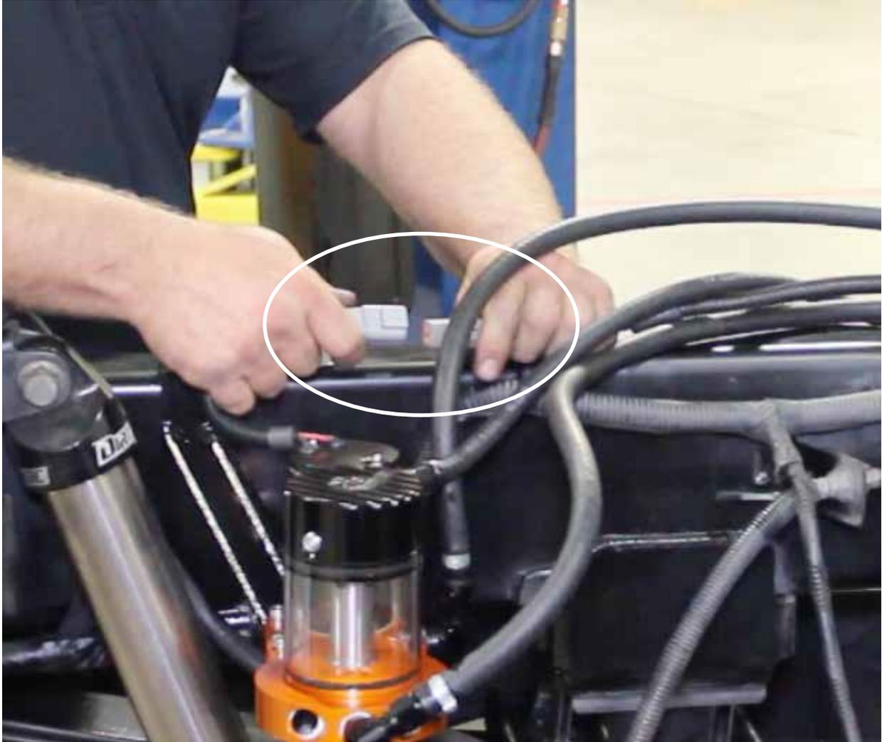
22. Plug the Deutsch connector into the mating connector on the DFS780.
