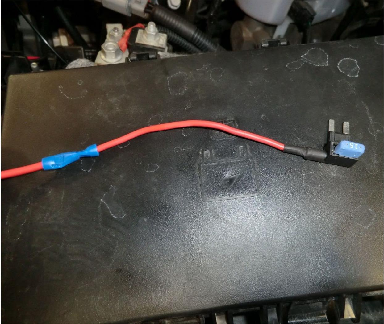
33. Attach the power wire from the relay to the inline fuse adapter.
