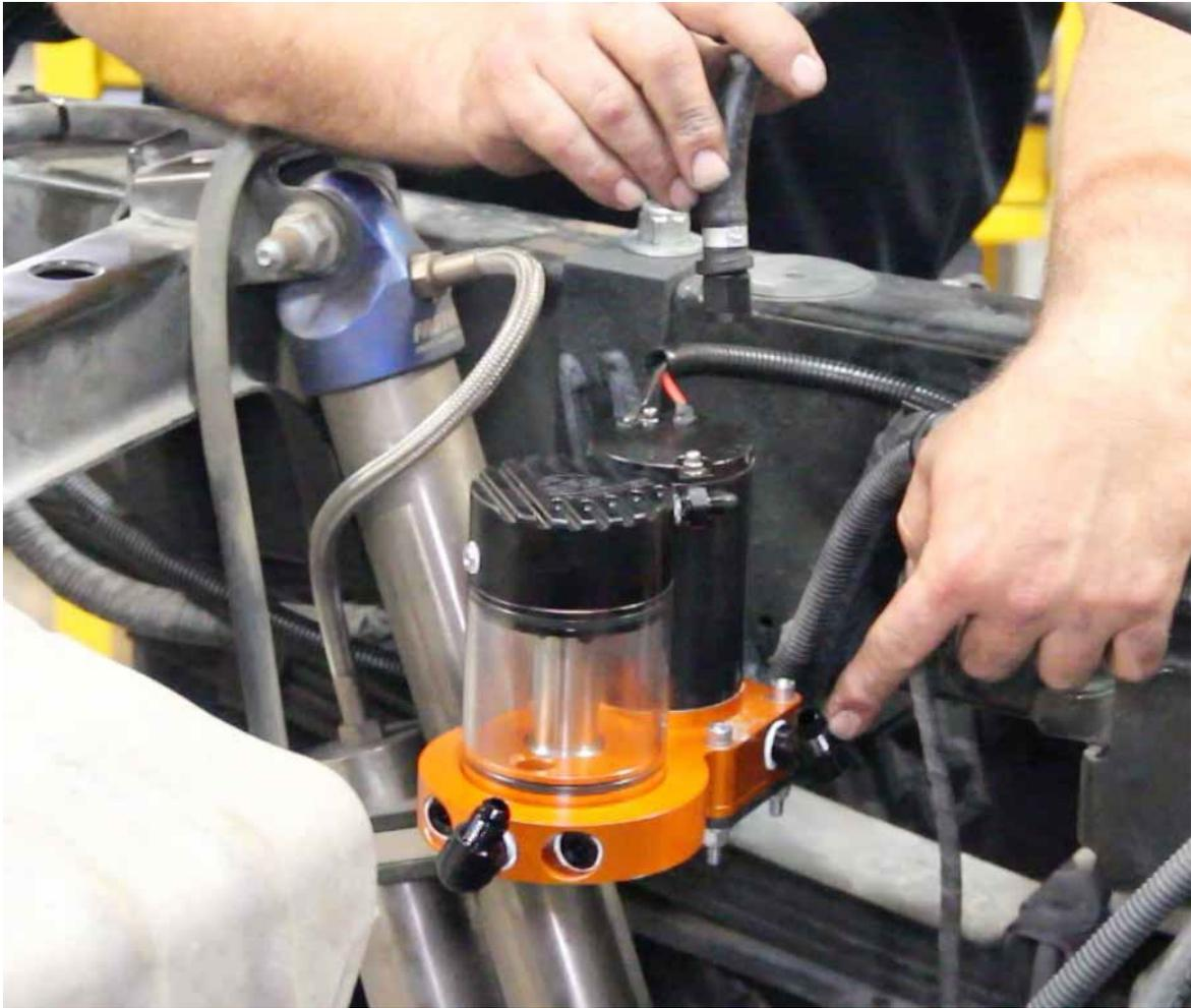
16. Install the fuel inlet hose (silver "AN" fitting) onto the fuel inlet port of the DFS780.
