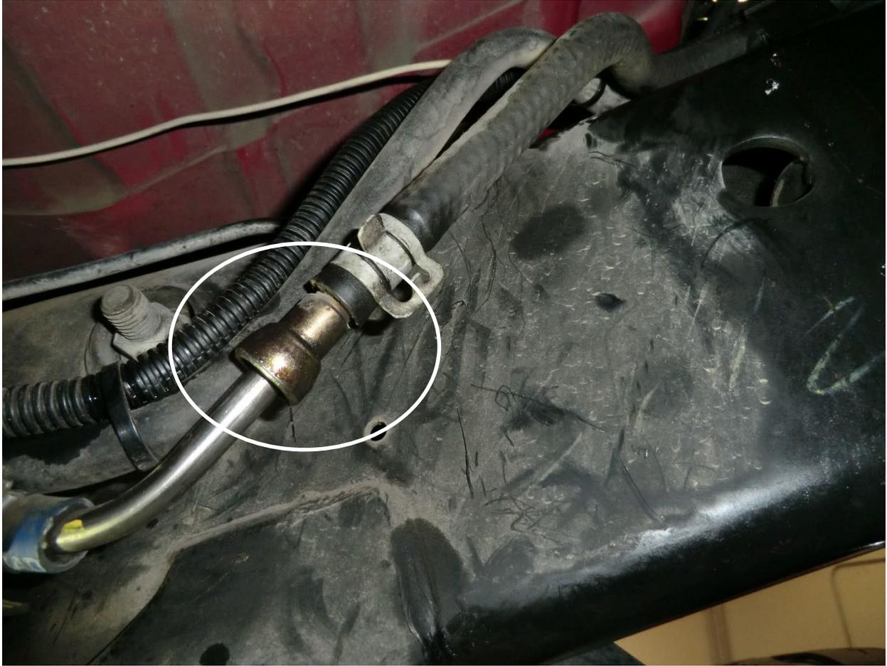
25. Disconnect the stock fuel pump feed hose located on the inside of driver's side frame rail under the driver's door.
