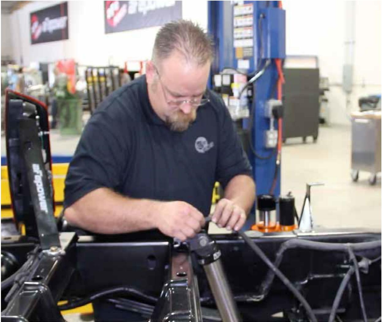
3. Remove the rear differential vent hose from the shock tower.
