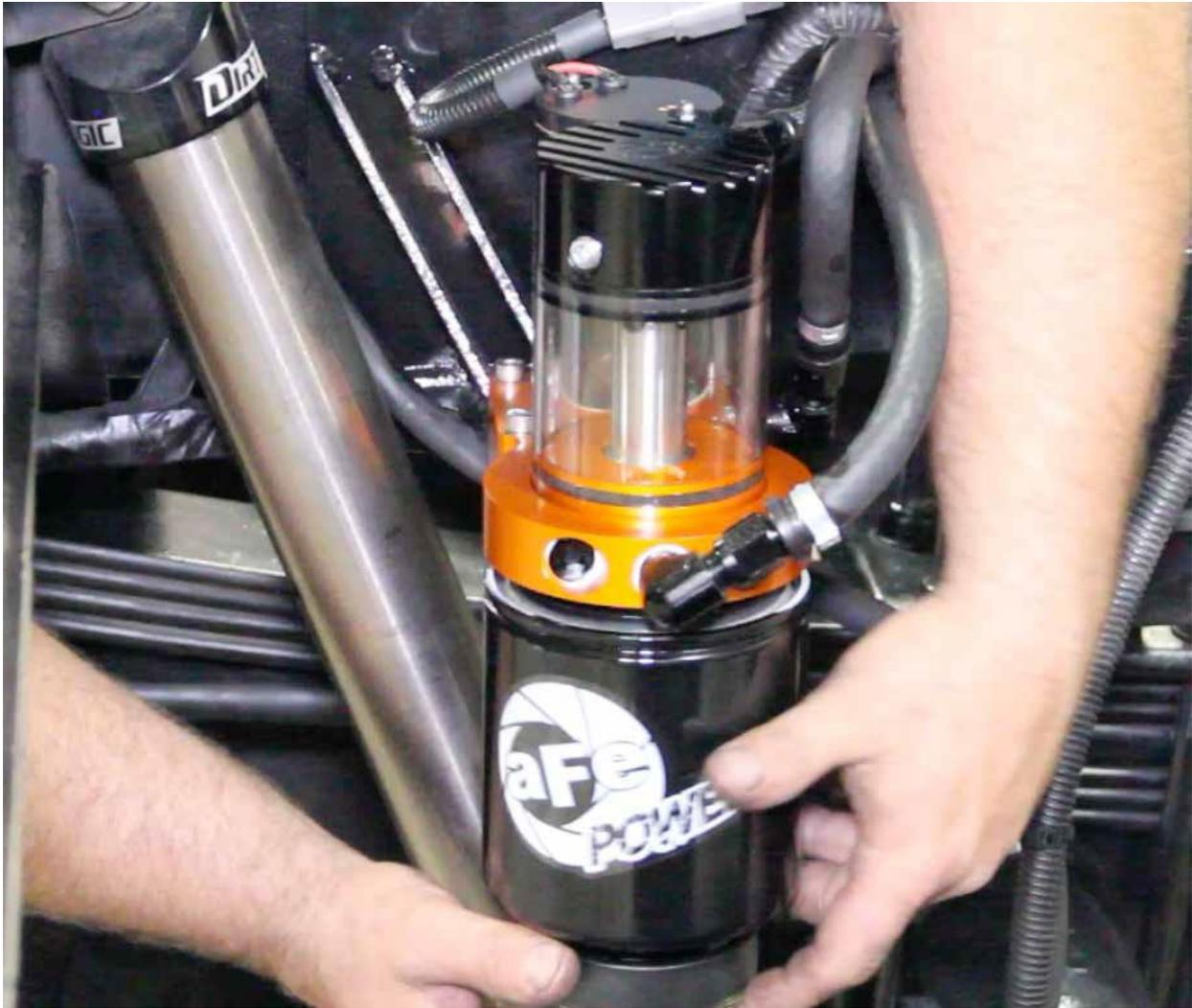
21. Using a light oil, lube the gasket on the fuel filter and install on the manifold. Thread the supplied water separator bowl onto the supplied fuel filter.
