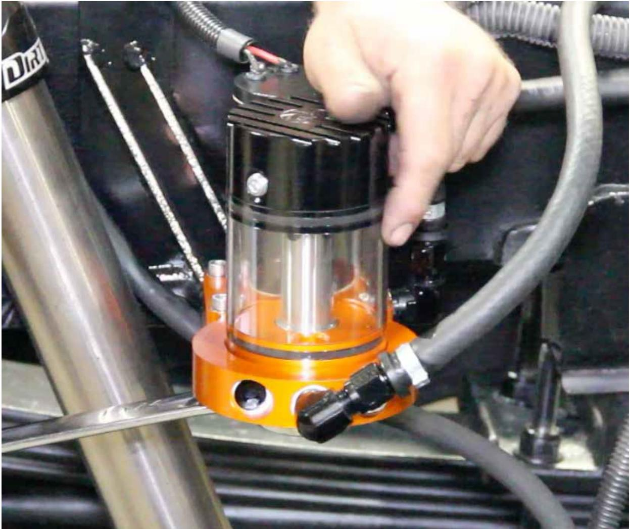
20. Turn sight glass to the desired angle and using a 1-1/4" wrench, tighten the center nut under the DFS780 manifold.
