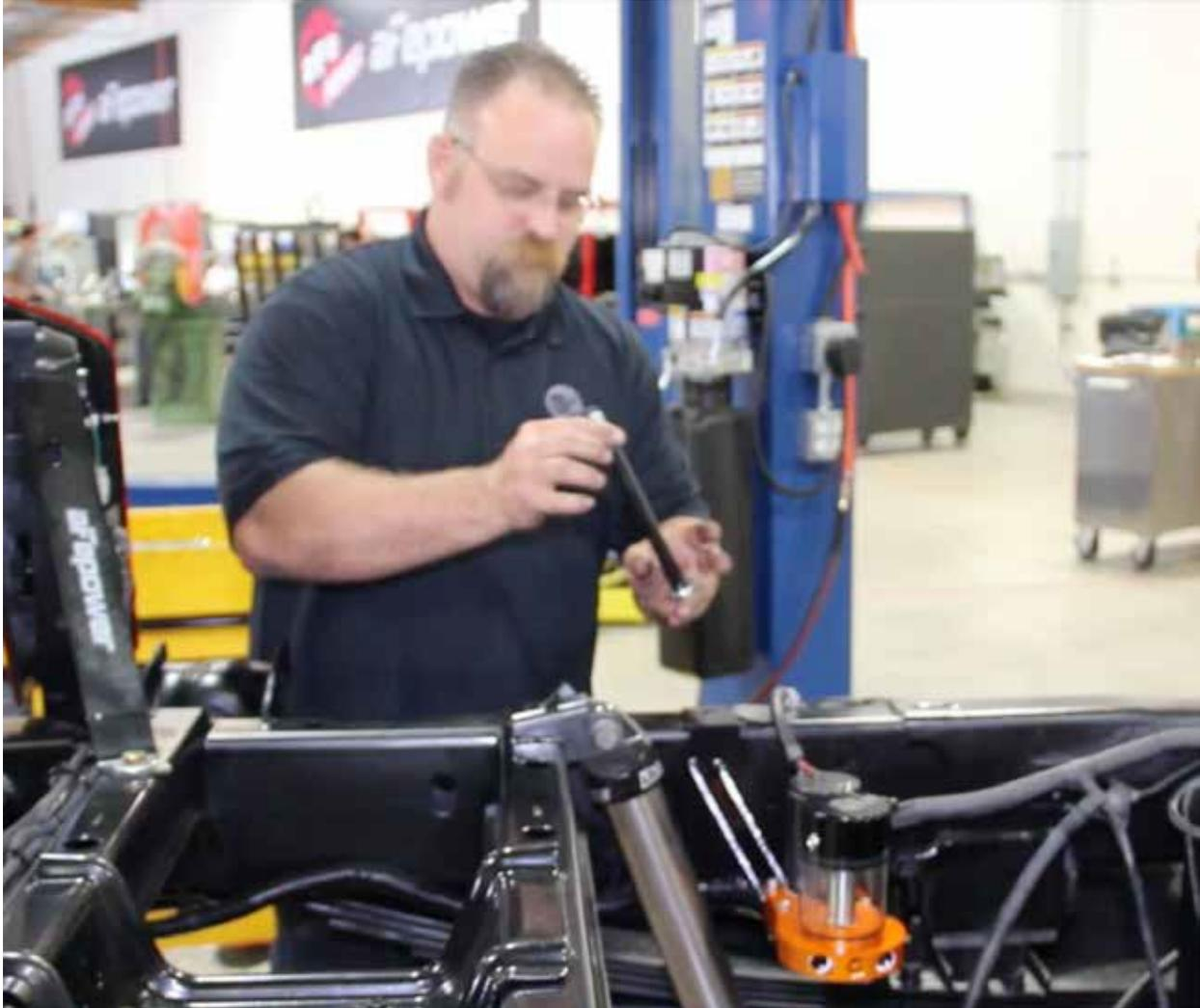
6. Secure the carbon steel frame bracket to the frame using the supplied hardware and tighten.
