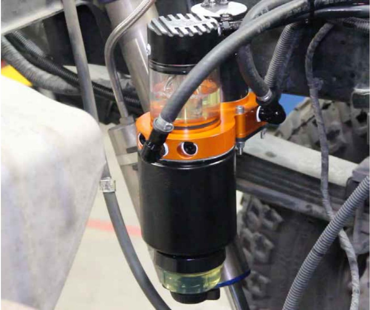
39. Turn the key to the “Run” position and watch to see if the DFS780 sight glass fills with fuel. If the DFS780 sight glass does not fill with fuel, use the Schrader valve (on the top of the DFS780) to release trapped air which will allow DFS780 to fill. If DFS780 still does not fill, try starting the engine.
