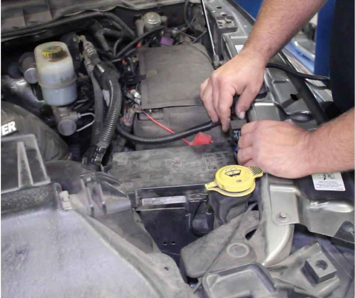
32. Secure the supplied relay using a supplied nylon cable tie.
