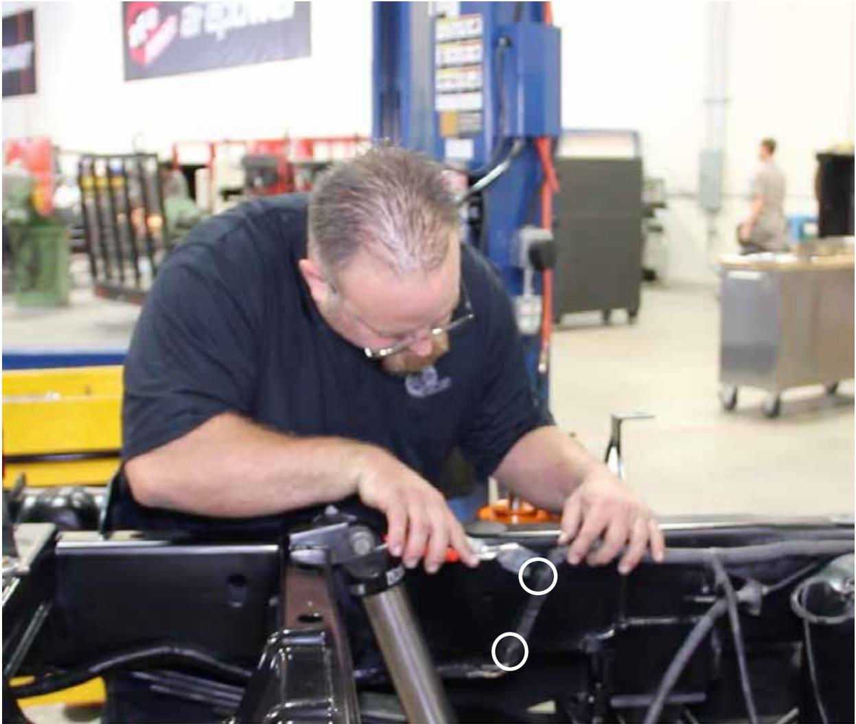
4. Remove the factory wire harness from the two mounting holes (as circled above).
