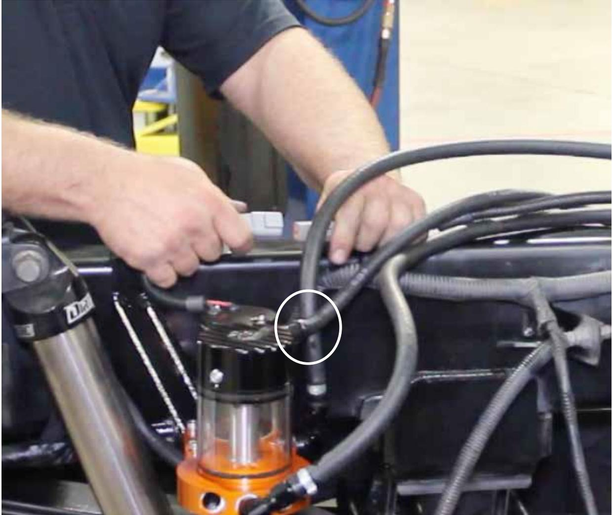
18. Run the supplied fuel return line (-4 AN fitting) down the frame toward the DFS780.
