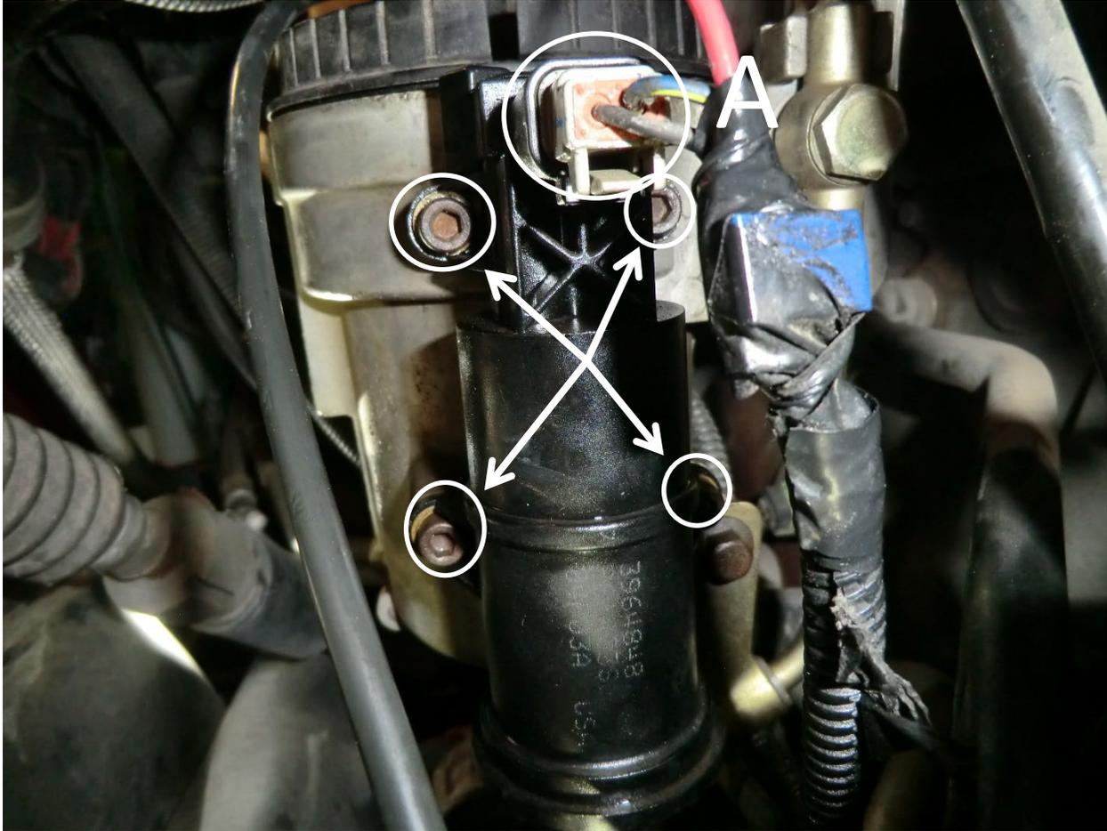
26. Disconnect the electrical connector (A) from the stock fuel pump.
