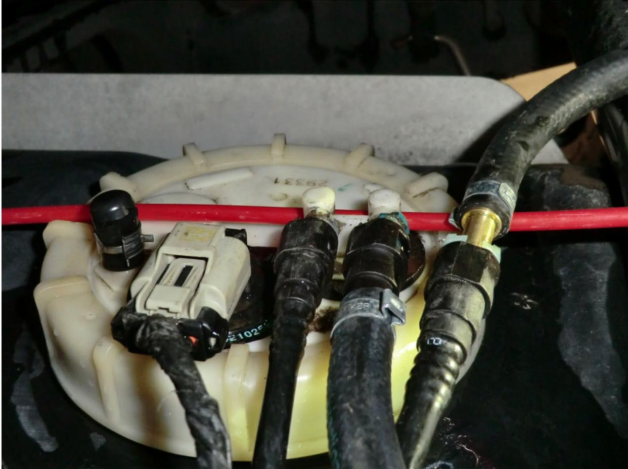
13. Install the supplied fuel outlet hose (with black “AN” fitting) onto the female side of the stock fuel line (shown below).
