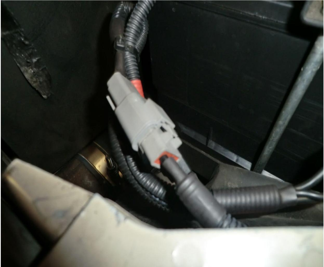
31. Plug the supplied relay harness into the Deutsch connector on the power harness.
