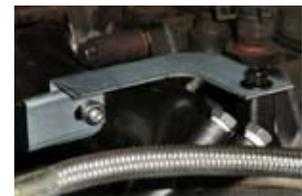
11. Re-install and tighten turbo with new (2) M10x1.5x50mm studs and (6) M10x1.5 flange nuts.
