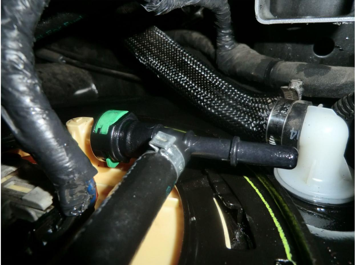
29. Install the female side of the "T" quick disconnect fitting on the supplied fuel return hose (shown below) onto the male fuel return connection on the top of the fuel sender assembly.
