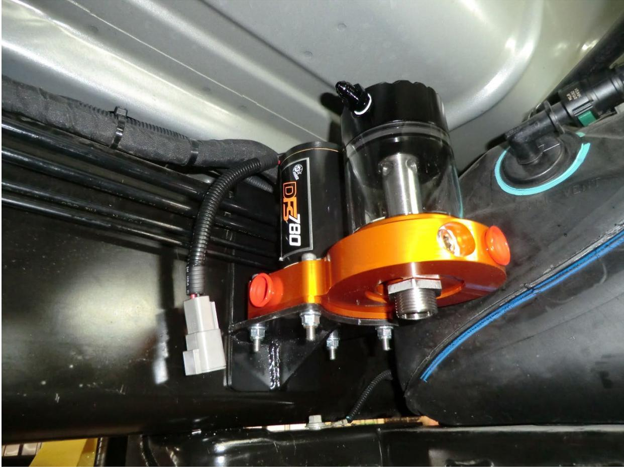
9. Mount the supplied fuel manifold assembly to the carbon steel frame bracket using the supplied hardware and tighten.
