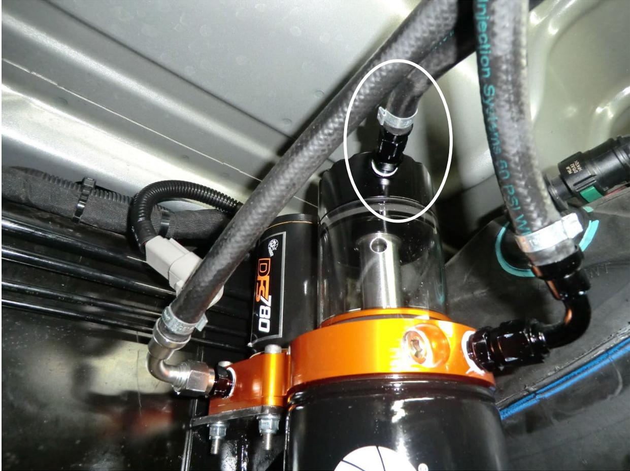
37. Install the fuel return hose (-4 AN fitting) onto the male -4 AN fitting on the top of the sight glass cover.
