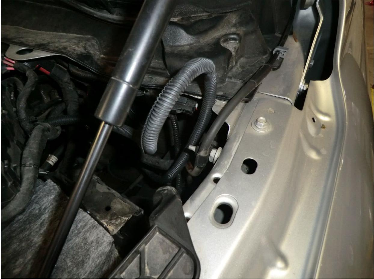
42. Run the other end of the power harness along the inside of the frame into the engine compartment.
