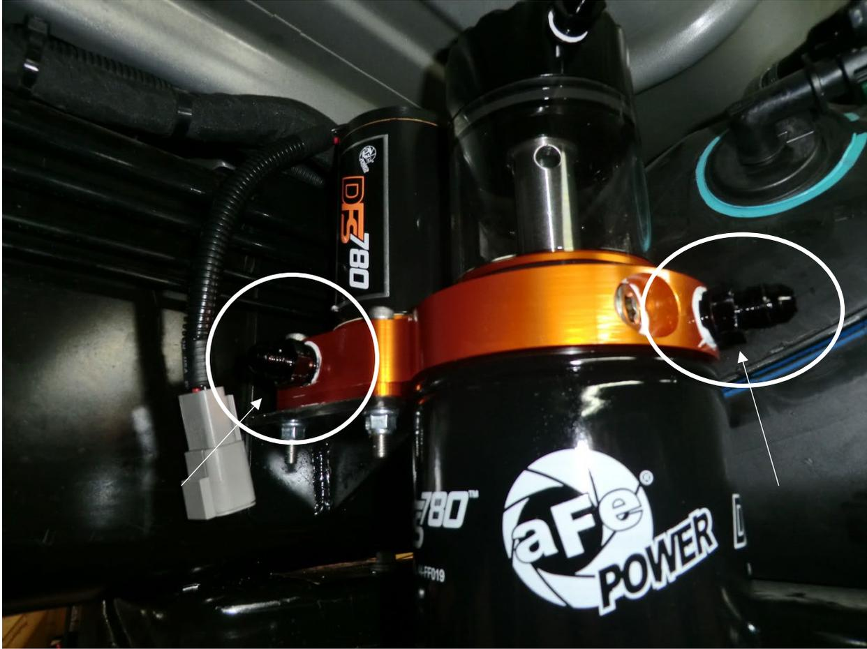
13. Install the 3/8" NPT to -6 AN fittings into the fuel manifold assembly (as shown above).
