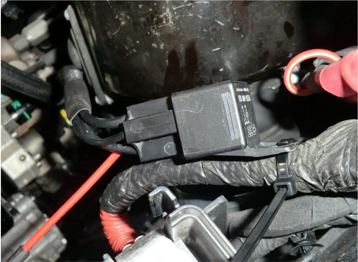
47. Secure the relay harness using a nylon cable tie.
