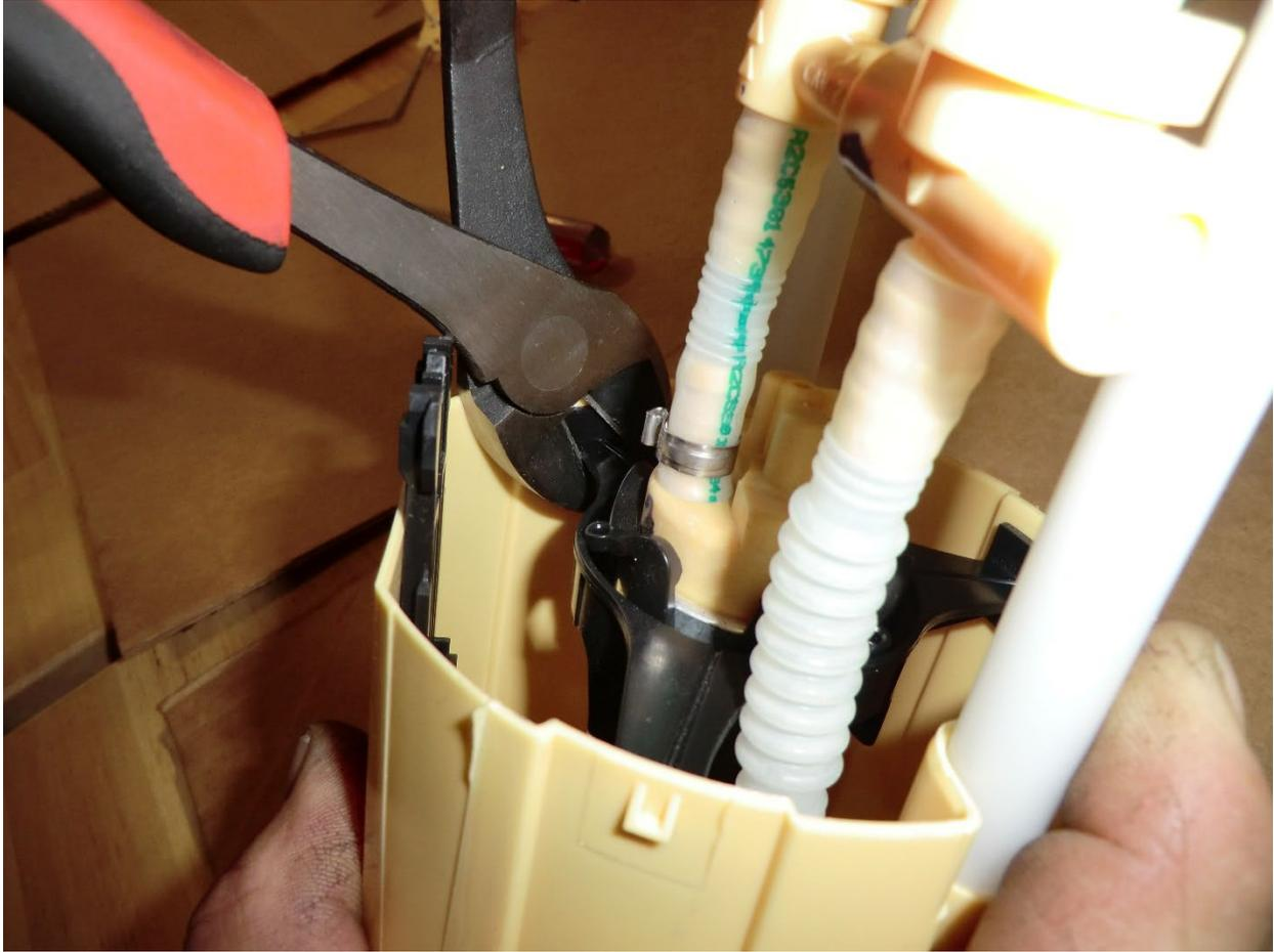
20. Carefully cut the three supports holding the factory fuel pump.
