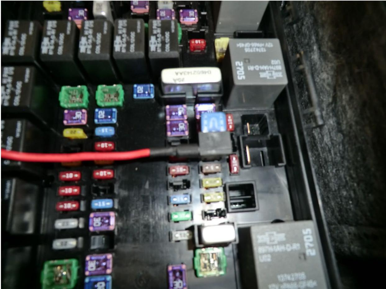
51. Install the add a harness fuse adapter (with installed fuses) into the 12-volt source inside the fuse box.
