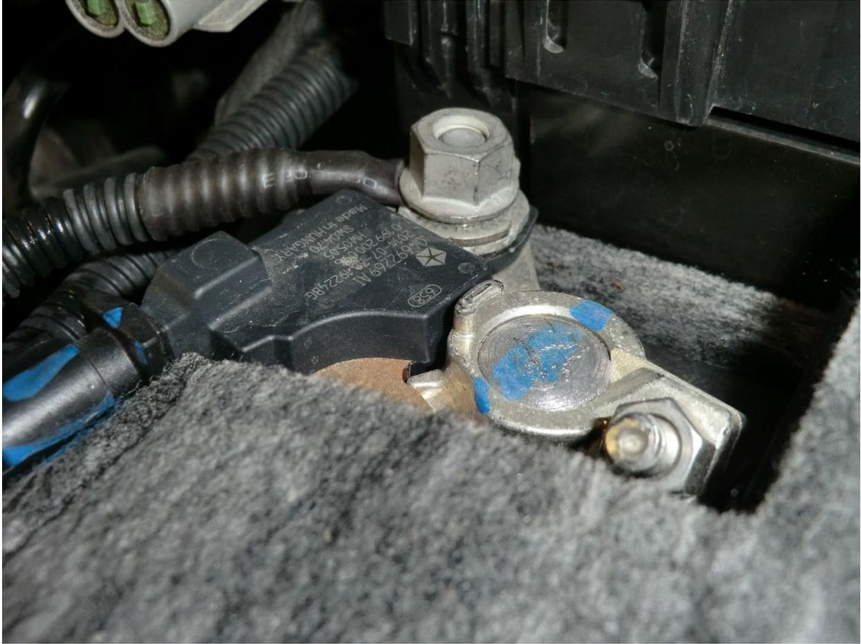
44. Connect the black wire ring terminal on the power harness to the negative side of the battery.
