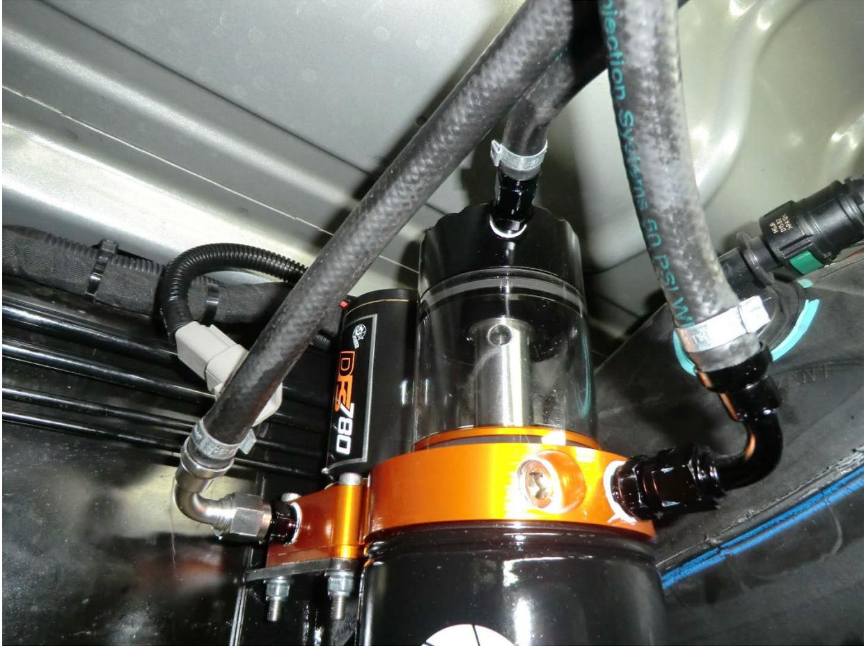
54. Turn the key to the “Run” position and watch to see if the sight glass fills with fuel. If the sight glass does not fill with fuel, use the tank valve (on the top of the sight glass cover) to release any trapped air. If the sight glass still does not fill, try starting the engine.
