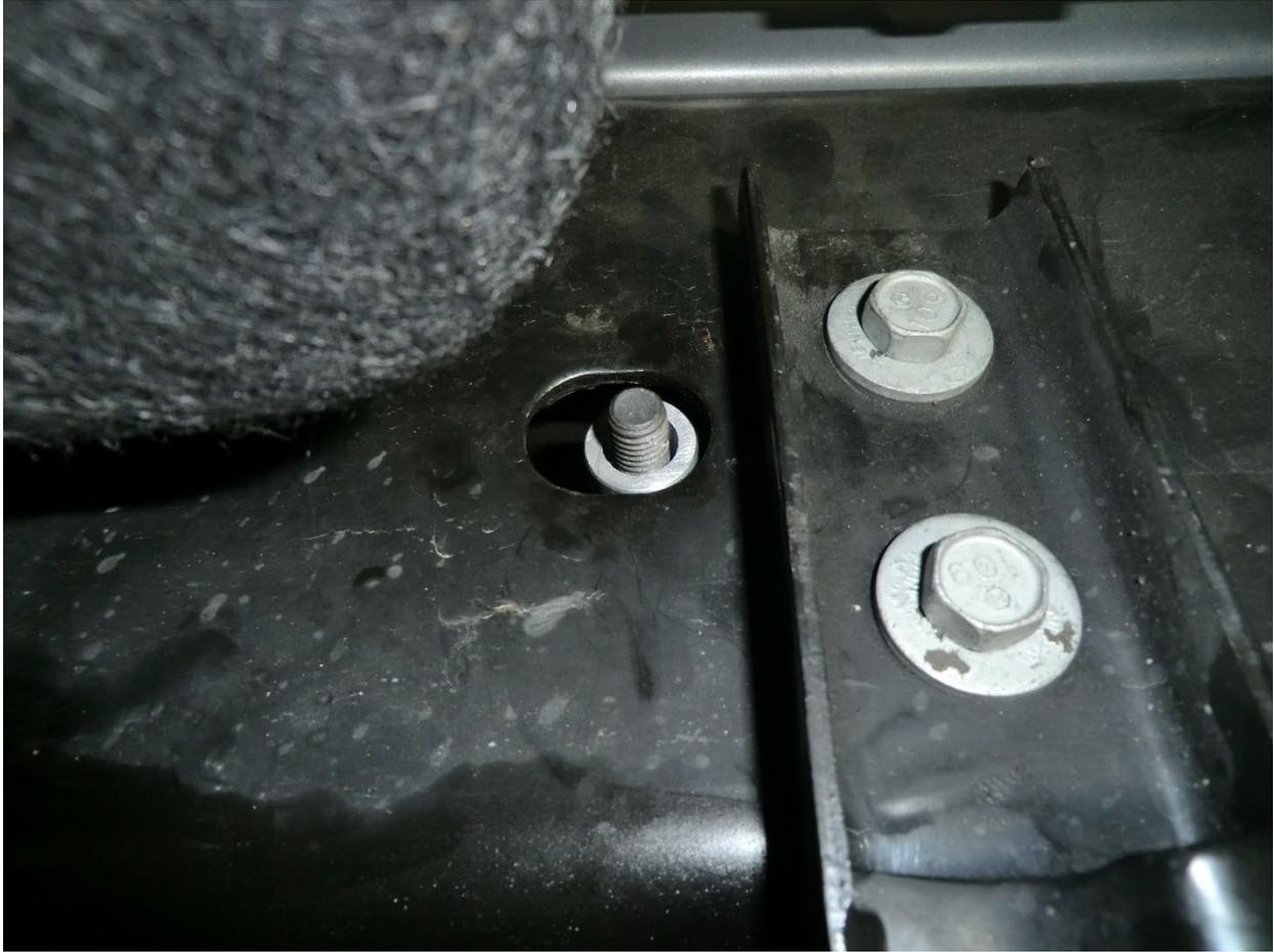
6. Install the supplied aluminum spacer onto the 3/8"-16 x 3.50" bolt.
