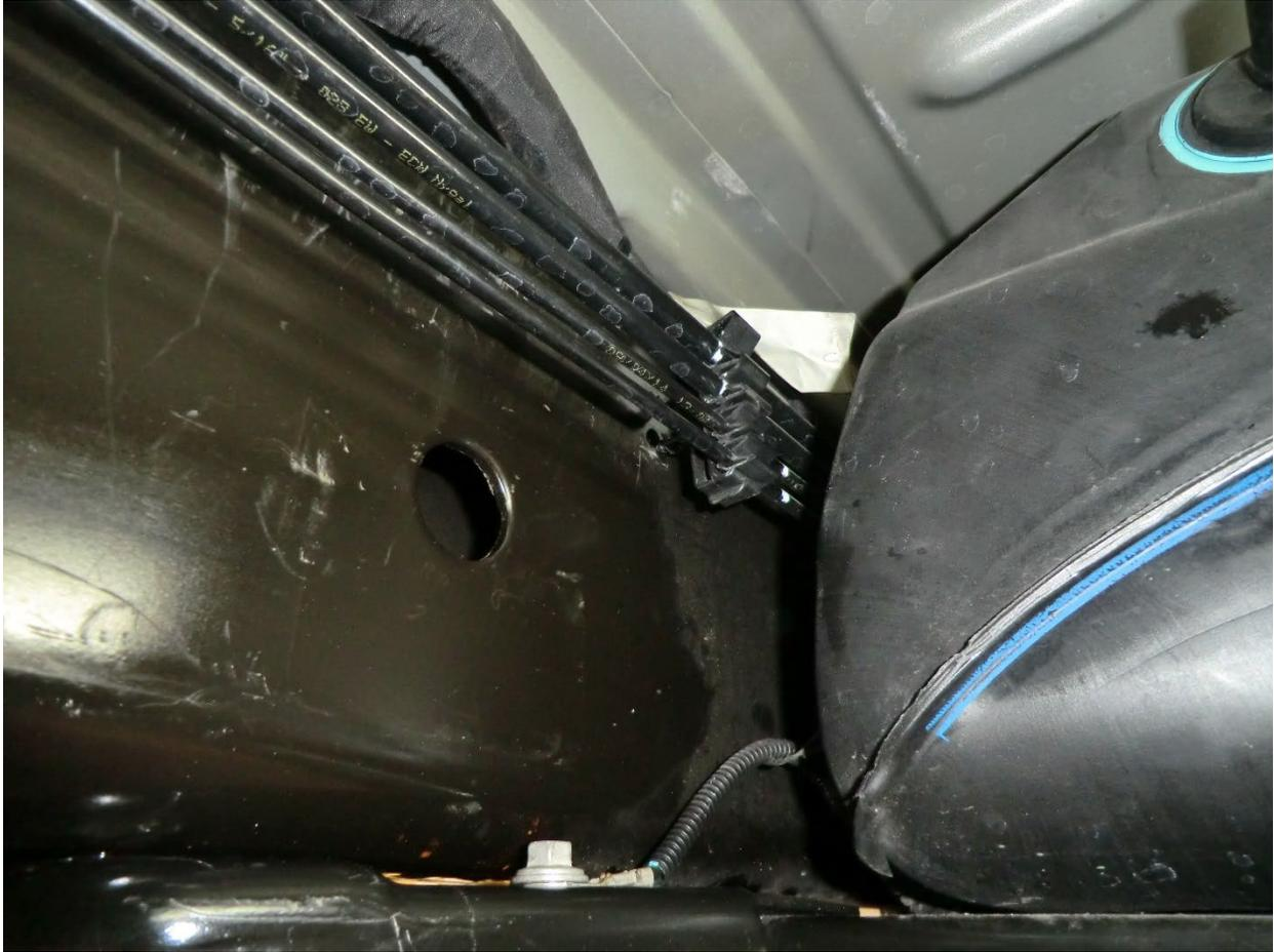
2. Gently pull the hard lines off the frame rail. Be careful not to bend or kink the hard lines.
