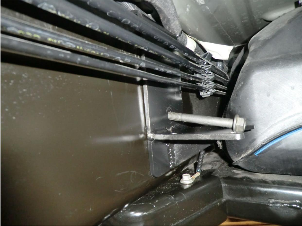
5. Install the supplied 3/8"-16 x 3.50" bolt through the carbon steel frame bracket and the frame rail.
