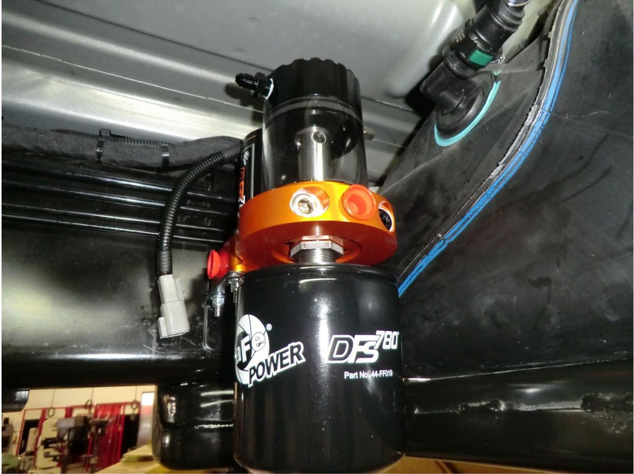
11. Using a light oil, lube the gasket on the supplied fuel filter and install on the fuel manifold assembly. Thread the supplied water separator bowl onto the fuel filter.
