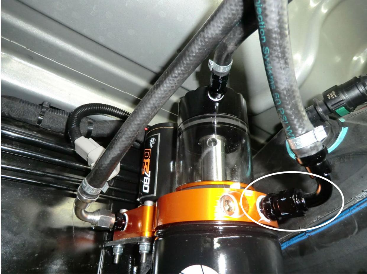
36. Install the fuel outlet hose (black 90° -6 AN fitting) onto the male -6 AN fitting on the fuel outlet port of the fuel manifold assembly.
