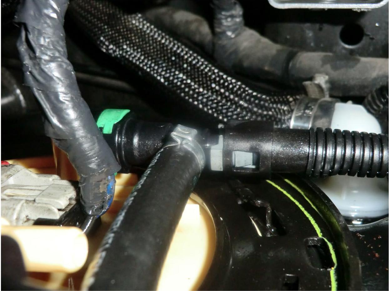
31. Install the factory female fuel return line onto the male side of the "T" quick disconnect fitting on the fuel return hose (shown below).
