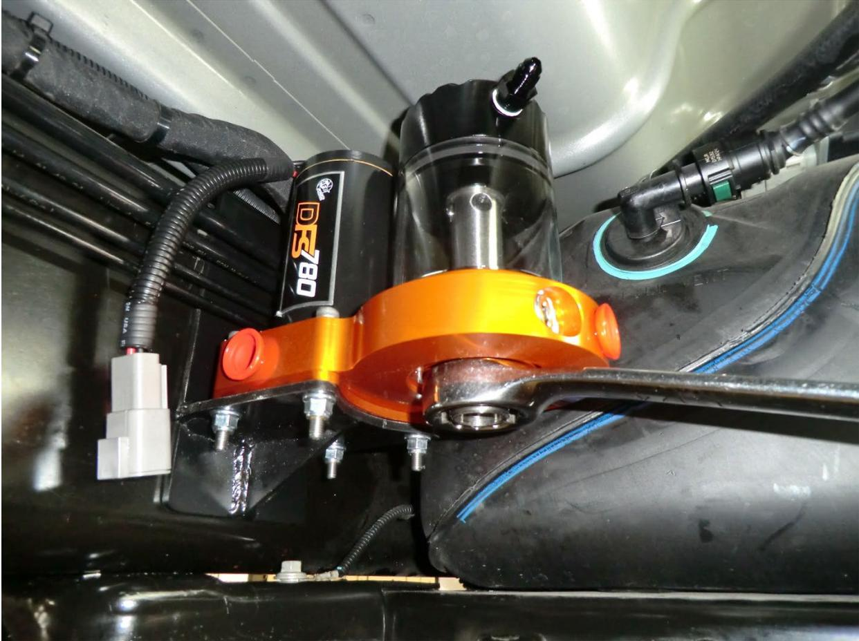
10. Turn the sight glass to the desired angle and using a 1-1/4" wrench, tighten the center nut under the fuel manifold assembly.
