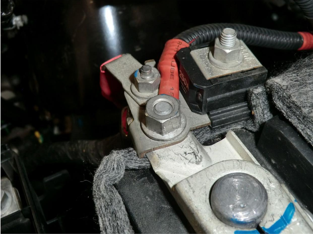
43. Connect the red wire ring terminal on the power harness to the positive side of the battery.
