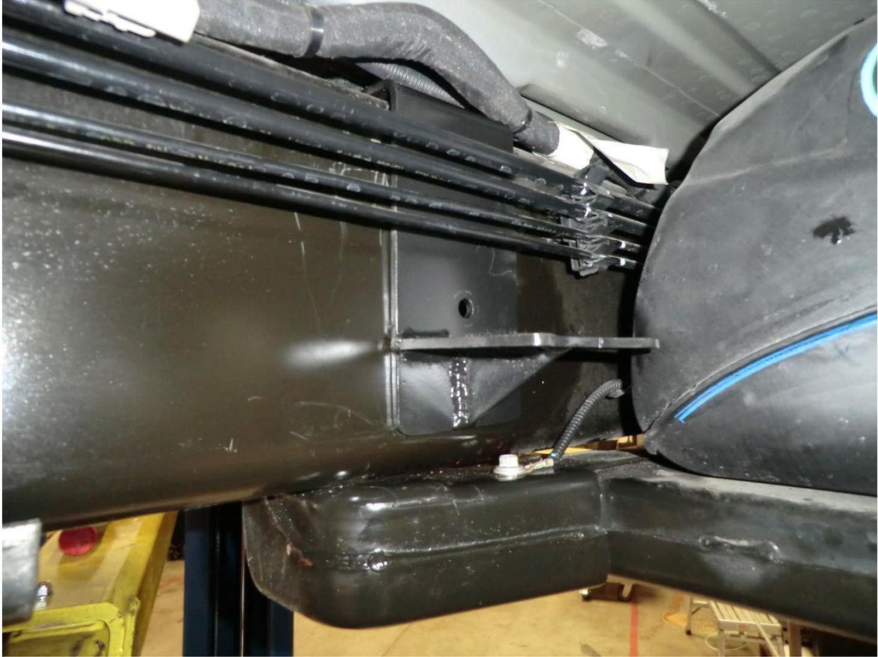
3. Place the supplied carbon steel frame bracket between the frame and the hard lines.
