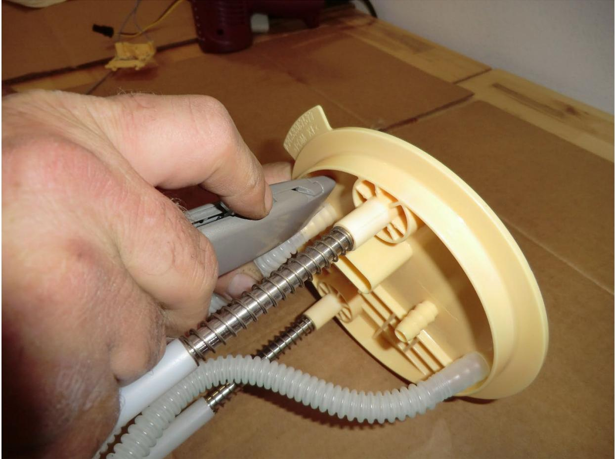
17. Unplug the electrical connector at the top of the fuel sender assembly.
