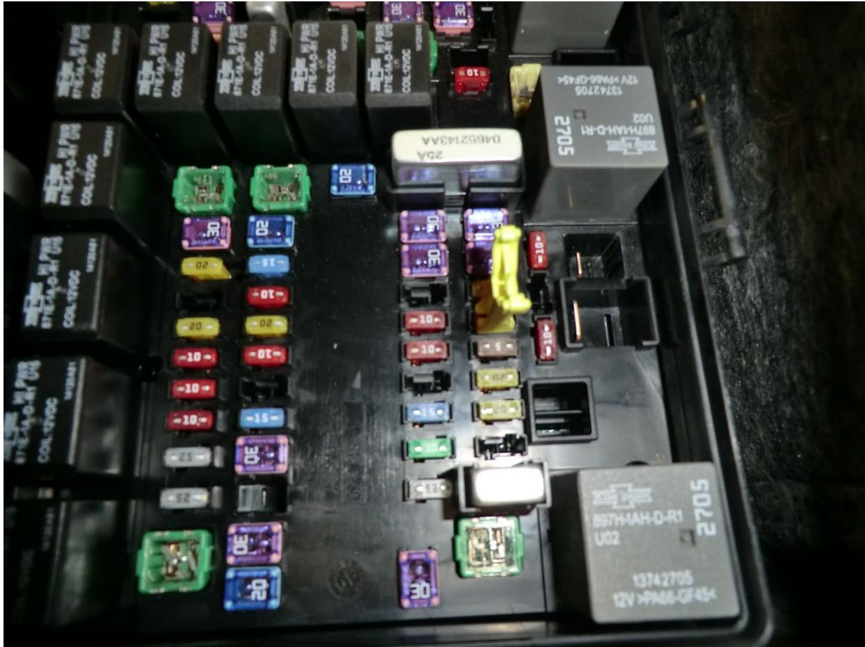
49. Find a 12-volt source inside the fuse box that only comes on with the key in the “run” position. Once a 12-volt source is located, pull the fuse from the fuse box.
