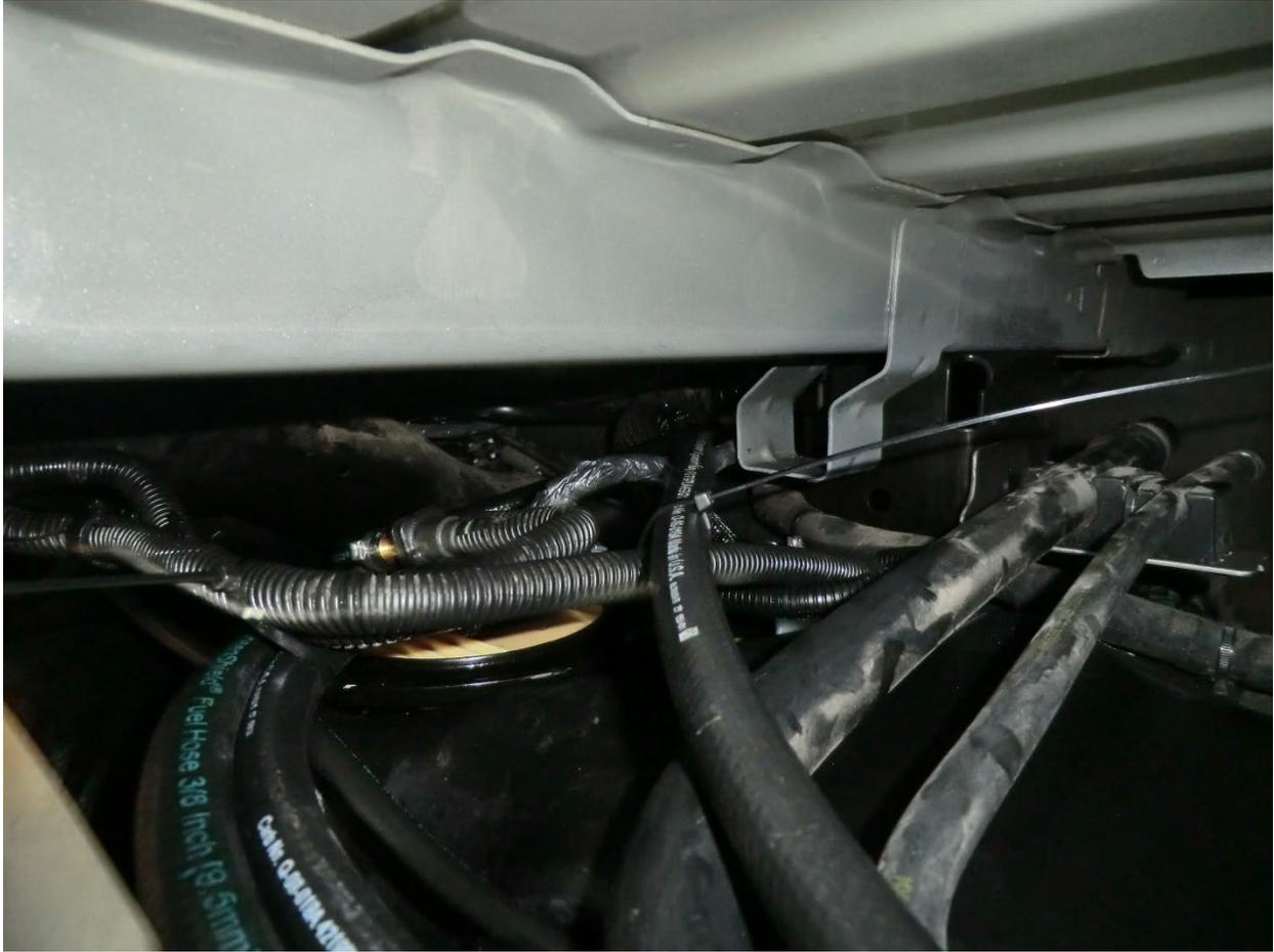
33. Route the new hoses as shown and secure with the supplied nylon cable ties.
