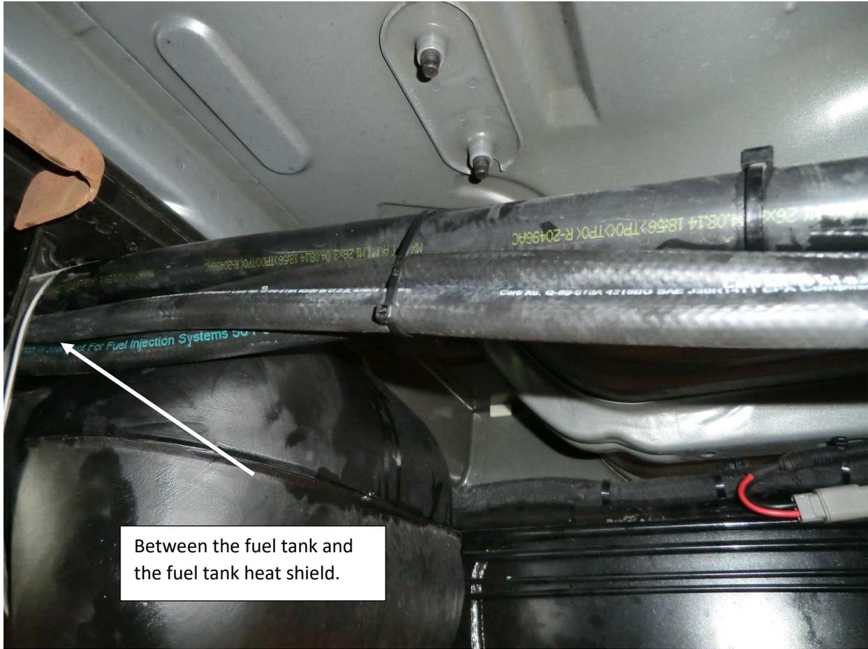
34. Route the new hoses along the DEF fill tube, between the fuel tank and the fuel tank heat shield. Secure with the supplied nylon cable ties (as shown above).
