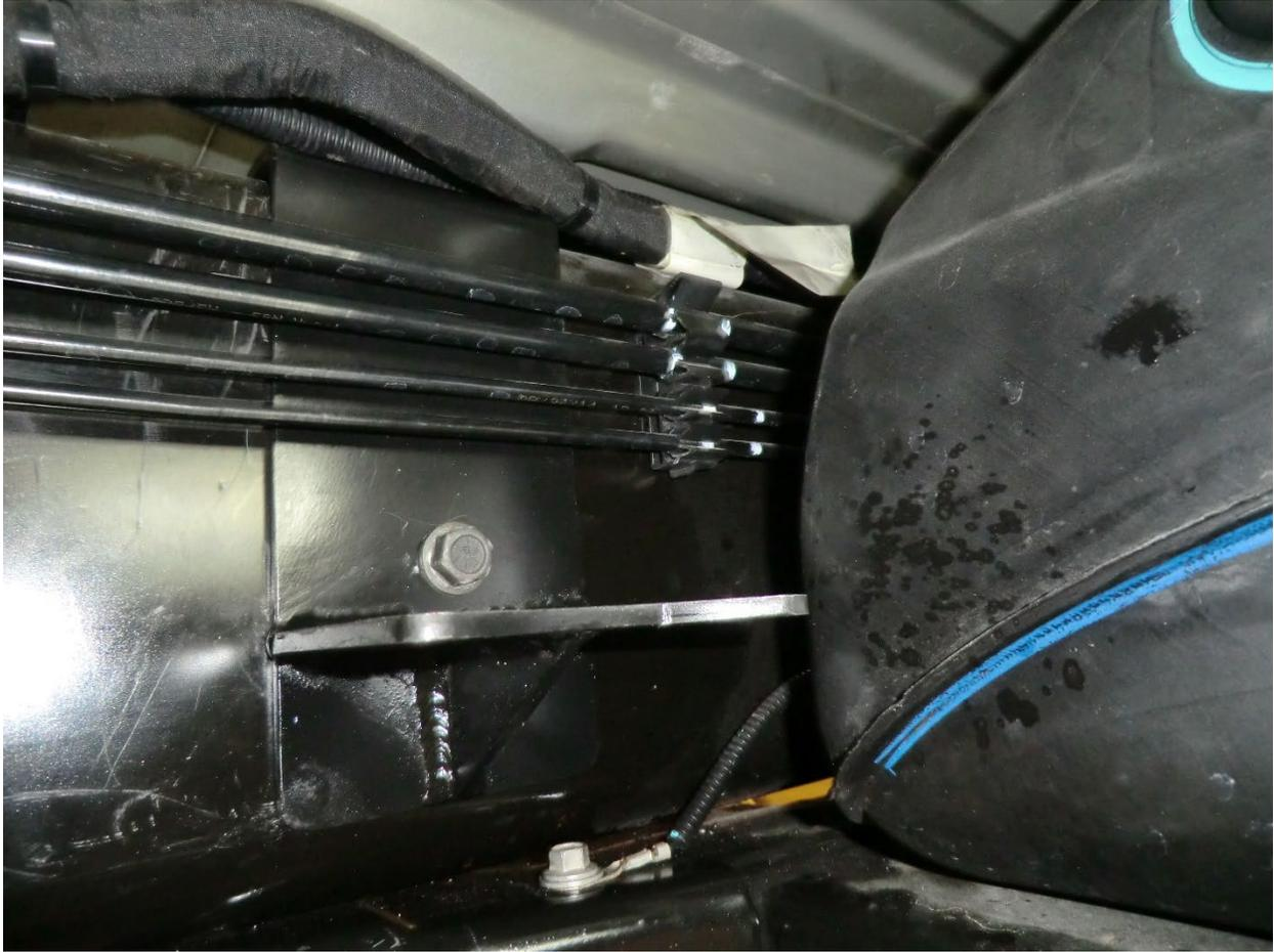
8. Re-install the hard lines onto the frame rail.
