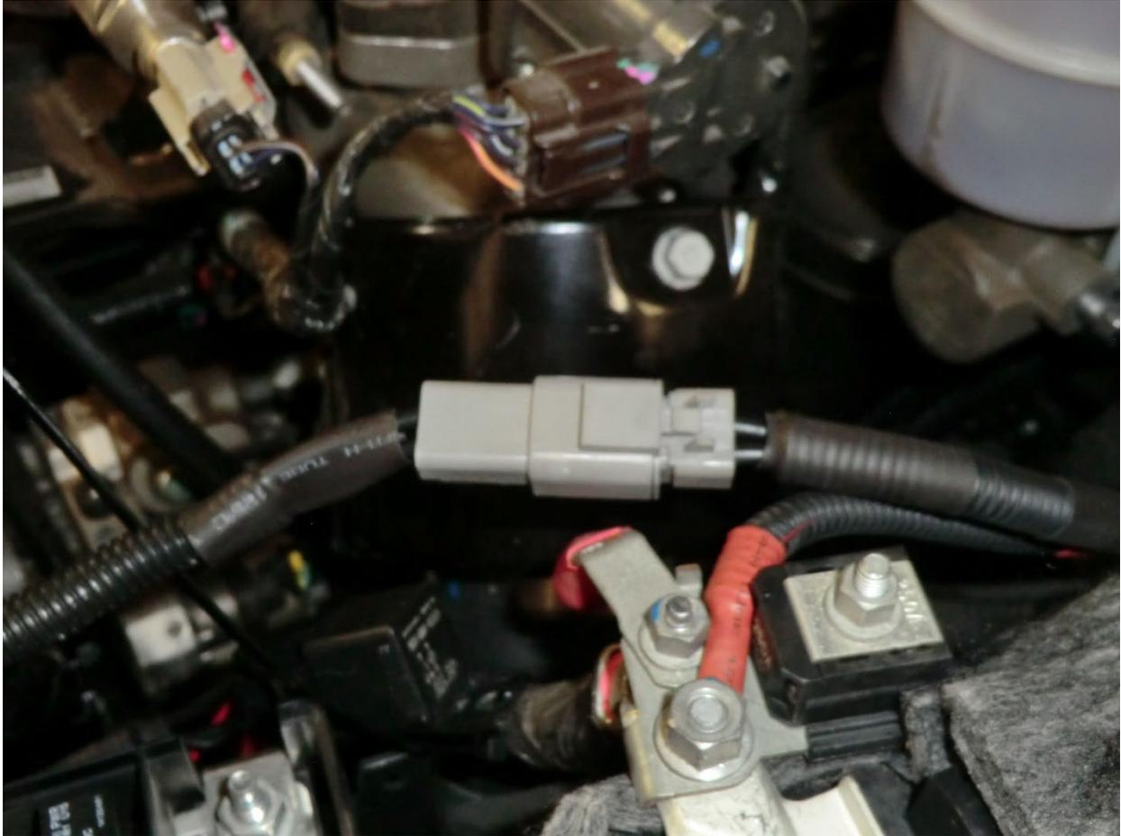
45. Plug the supplied relay harness into the weatherproof connector on the power harness.
