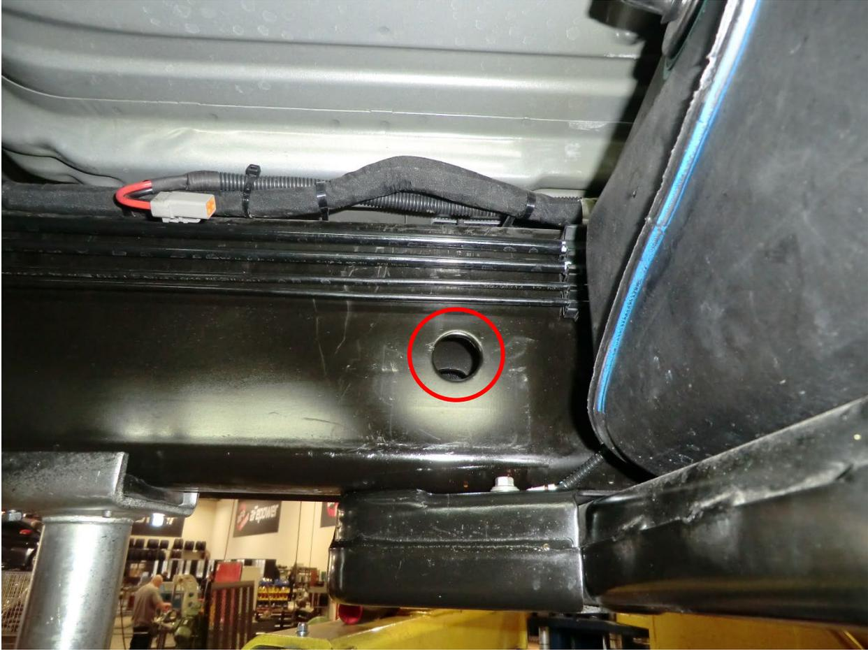
1. Locate the hole in the driver's side frame rail behind the DEF tank and in front of the fuel tank.
