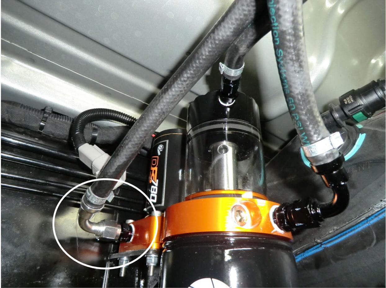
35. Install the fuel inlet hose (silver 90° -6 AN fitting) onto the male -6 AN fitting on the fuel inlet port of the fuel manifold assembly.
