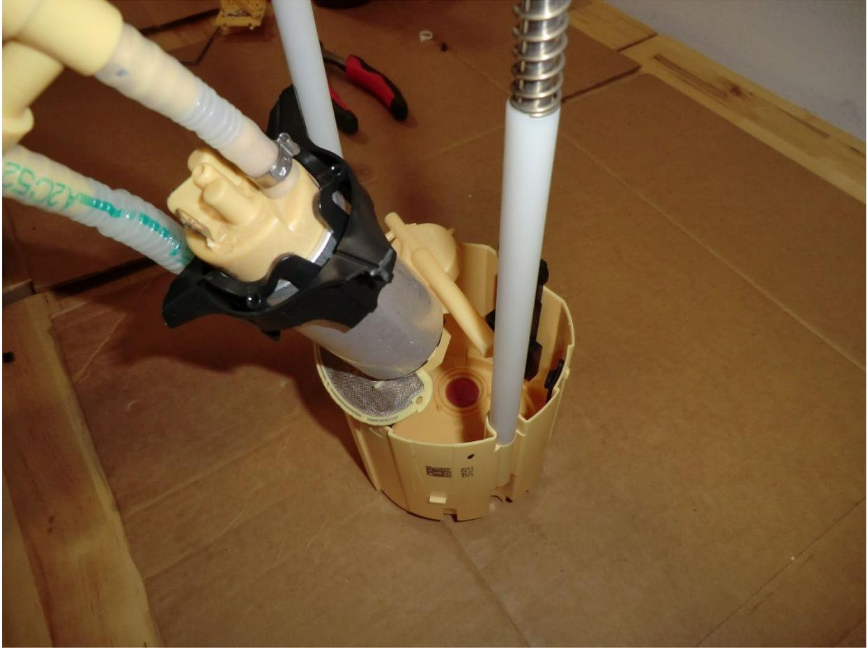
21. Remove the factory fuel pump, suction line and return line from the fuel sender assembly.
