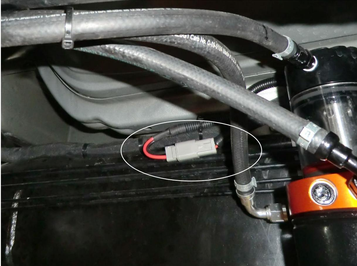
39. From the inside of the frame, plug the weatherproof connector on the supplied power harness into the mating connector on the fuel pump motor.
