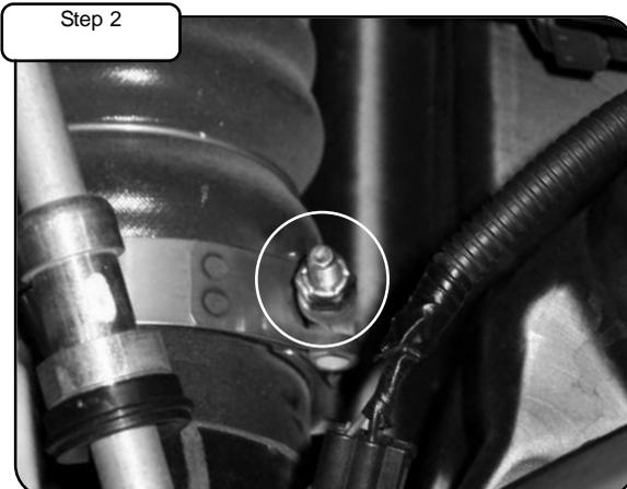
With 7/16" deep socket, loosen clamp on intercooler.
