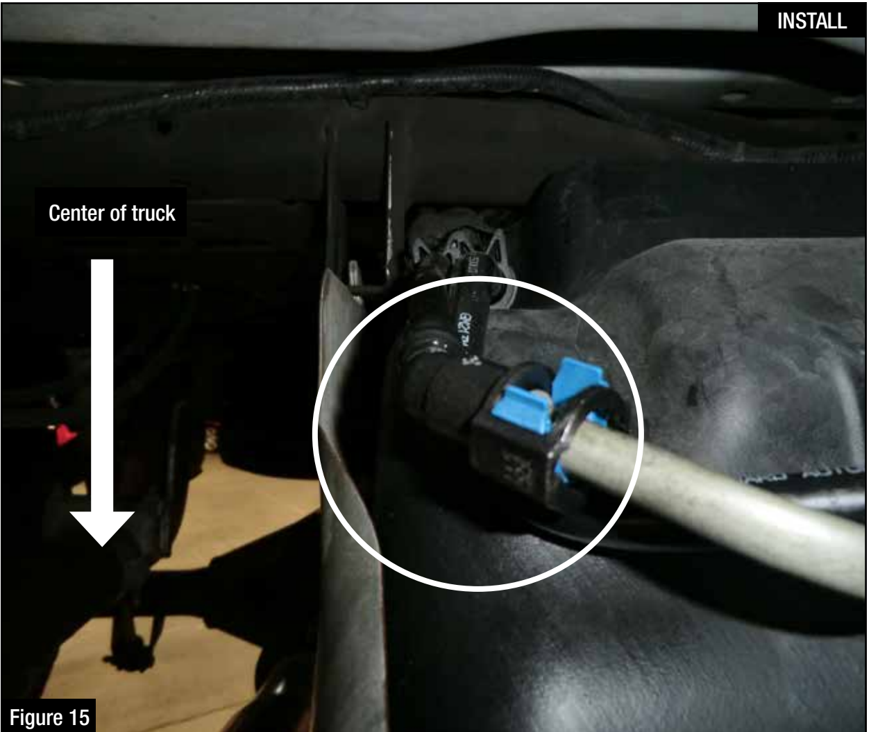
Figure 15 Step 16: Locate the factory fuel return line. It is located at the front of the fuel tank near the center of the truck.
