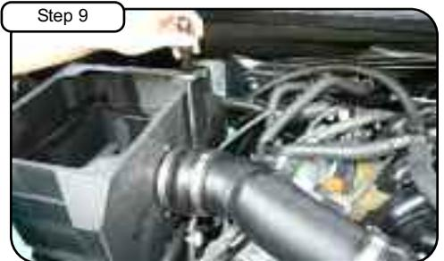
Tighten clamps with 5/16" nut driver. Take out OE crankcase line and replace with 1/2" hose and clamp provided.
