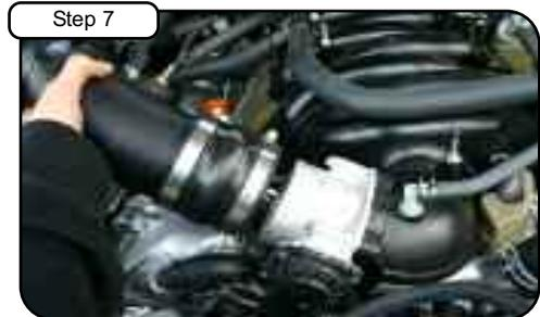
With couplers and clamps provided, place onto new intake tube and install. **Make sure 4-1/4" coupler is on filter side and 3-1/2" coupler is on throttle body side.**
