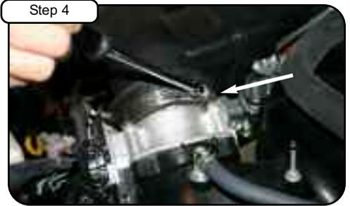
With 5/16" nut driver loosen both clamps on OE intake tube. Remove crankcase and vacuum line away from tube. Disconnect MAF sensor harness & remove.
