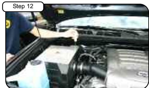
With button head screws provided tighten down housing cover with 5/32" allen key. Re-Install engine cover.
