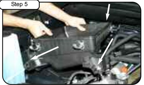
With 12mm socket with extension, loosen the 3 bolts and remove the OE air box out of vehicle. **Note: Save 3 bolts and grommets for later install.**
