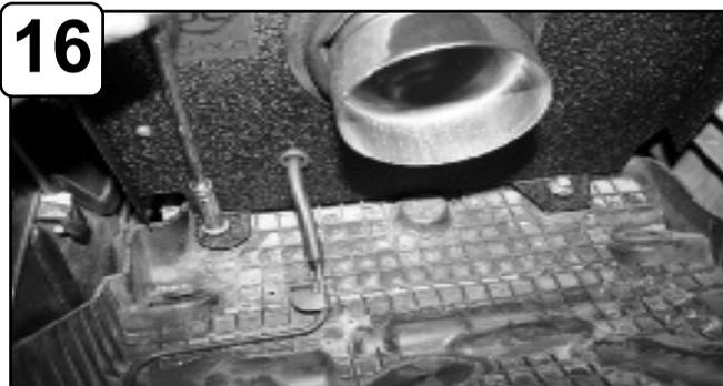
16 Tighten screws using 10mm socket or wrench.
