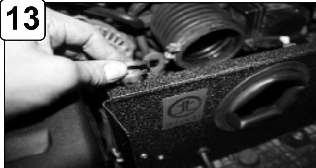
13 Remove OE grommets from air box and install to hole cut outs on top of housing.
