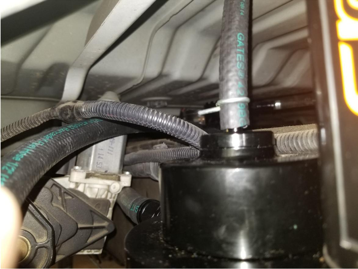
17. Carefully route the  $\frac{1}{4}$ " hose to the top of the air chamber on the fuel manifold assembly, making sure not to kink the hose or allow it near moving parts. Carefully mark and then cut the hose to the correct length. Using the supplied spring clamp, attach the hose to the nipple on the top of the air chamber on the fuel manifold assembly.
