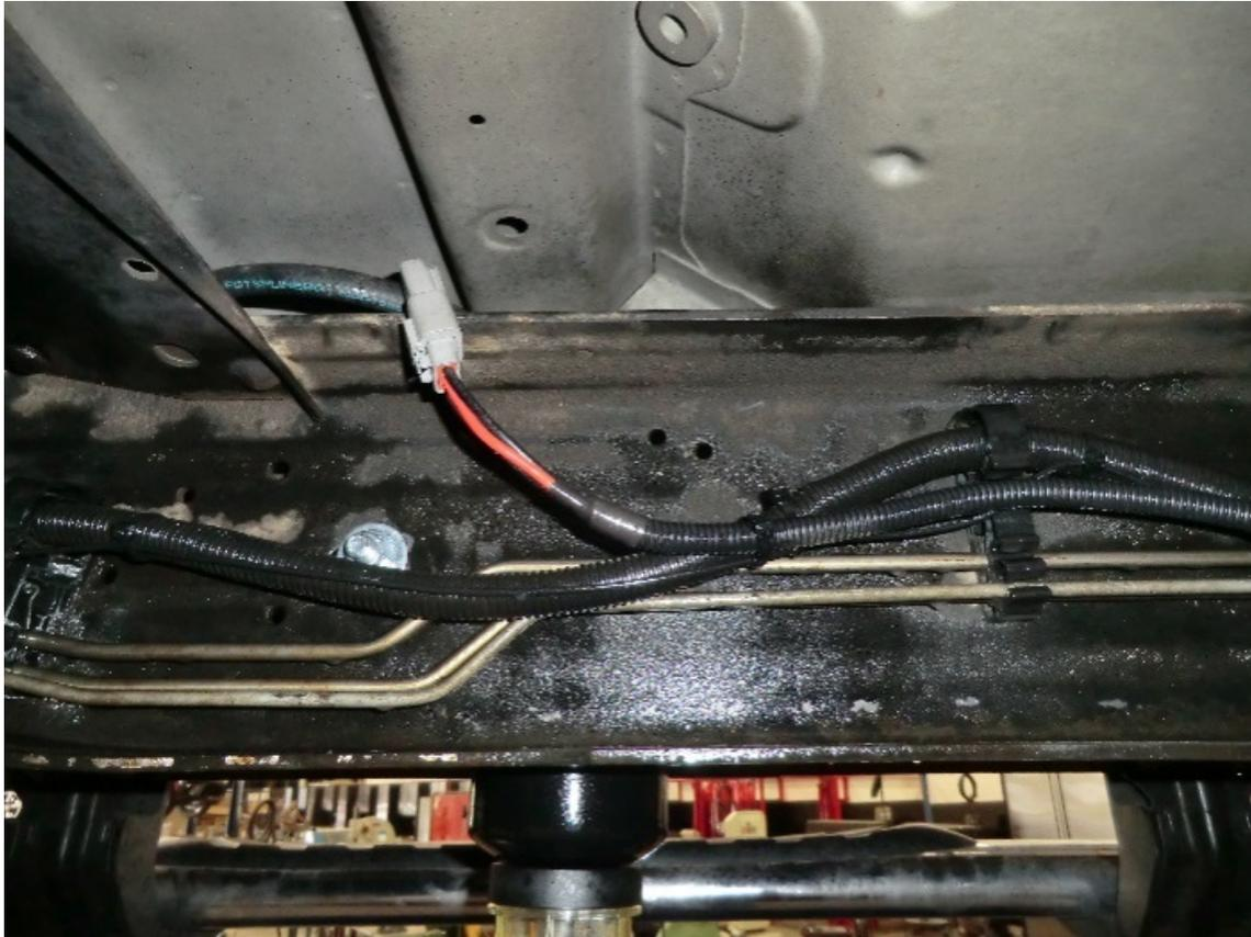
18. Plug the weatherproof connector on the end of the supplied power harness into the mating connector on the fuel manifold assembly motor. Route the power harness along the inside of the frame and into the engine compartment.
