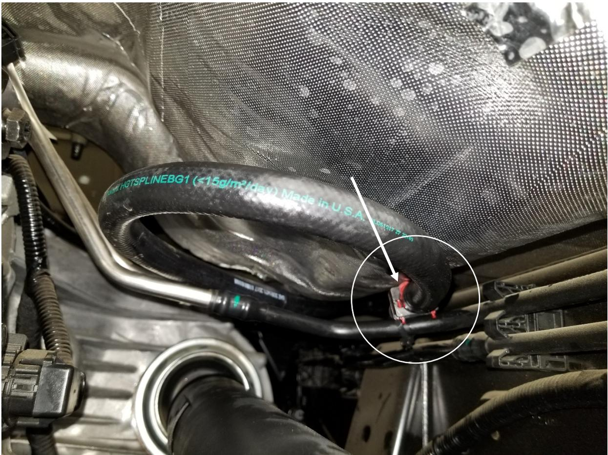
11. Disconnect the factory fuel supply line. Attach the male quick disconnect fitting on the supplied inlet/outlet hose to the factory female quick disconnect fitting on the factory fuel supply line. Route the hose to the inlet port on the fuel manifold assembly, making sure not to kink the hose or allow it near moving or hot parts. Carefully mark and then cut the hose to the correct length.
