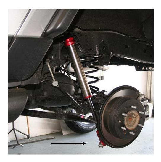
9. Next, install the top stud though the frame. Only one black urethane bushing should be on the stud when you insert the stud through the hole in the frame. Make sure the Racerunner logo is facing out and the Schrader valve axis is parallel to the vehicle axis.
