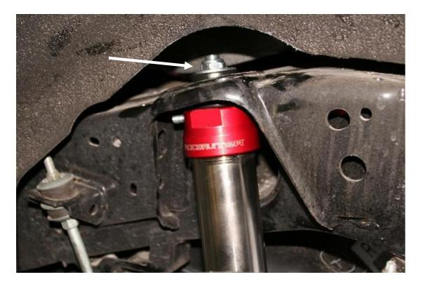
10. Place the second bushing on the stud, on the top side of the frame, followed by the washer and the locknut. Hand-tighten the locknut, until the nylon engages and the nut starts to tighten.
