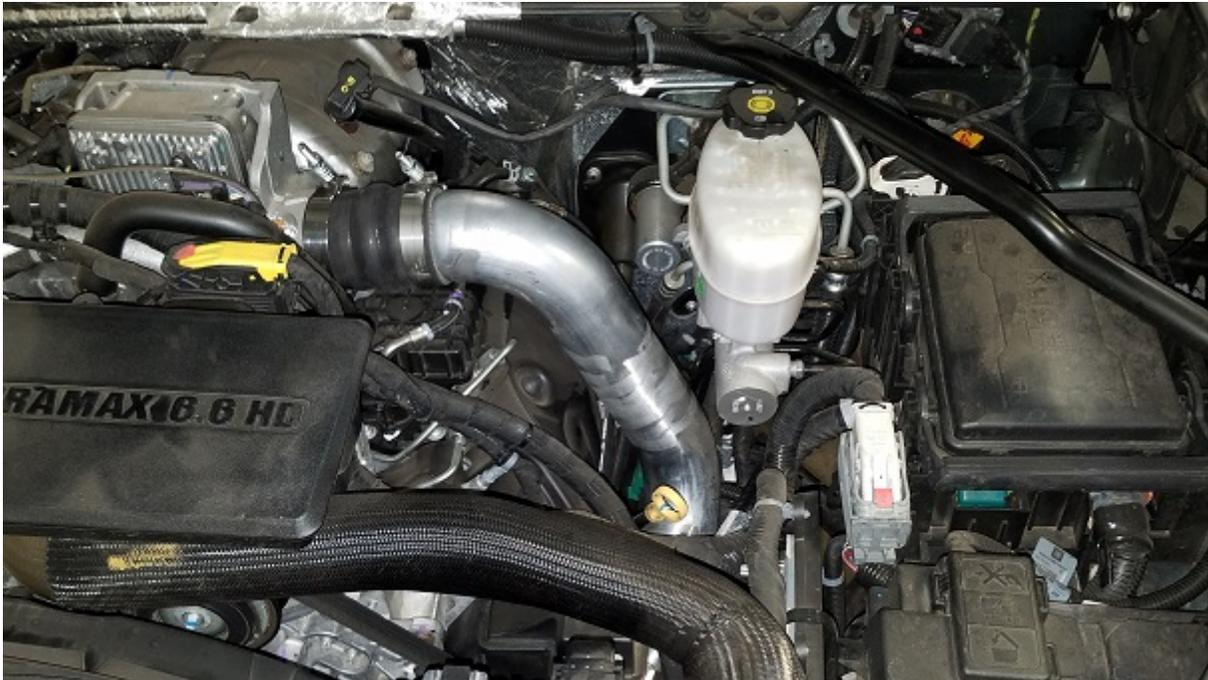
15. Ensure tubes are not touching anything then tighten all the clamps using an 11mm socket.
