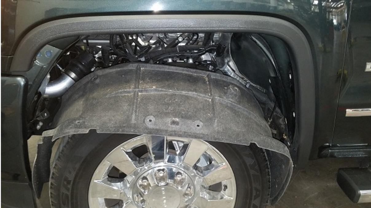
11. Install one of the 3" clamps and the small hump coupling onto the turbo then install the longer tube into the vehicle from the top.
