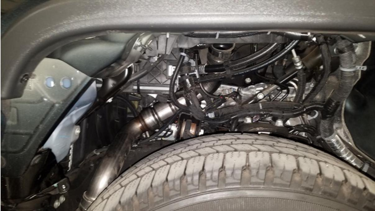
5. Loosen the clamp securing the coupling onto the intercooler using a 11mm socket, it will be accessible from the top behind the radiator with a long extension.
