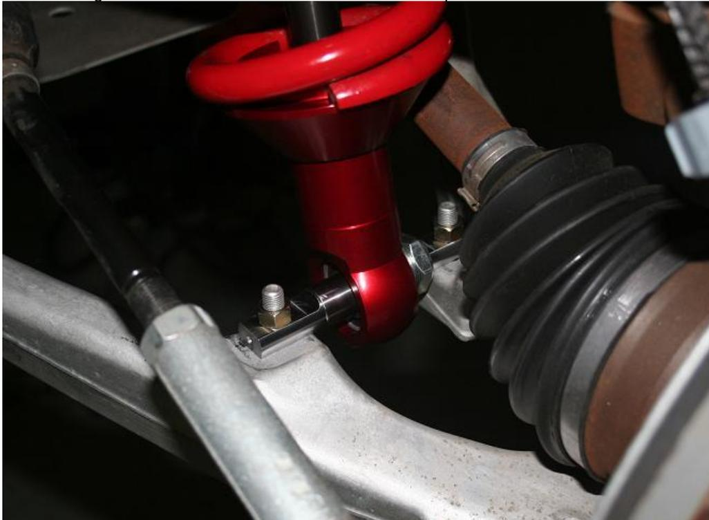
13. Using a **9/16"** wrench or socket torque the new spring hat 3/8"bolts to 25ft lbs. Tighten the nut on the lower mounting pin (1-1/16") to 50ft lbs using a **1-1/16"** wrench or crescent wrench.
