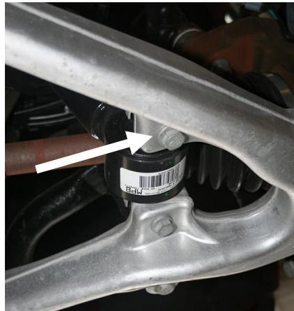
8. Using a **15mm** socket remove the 2 bolts from the lower shock mount.
