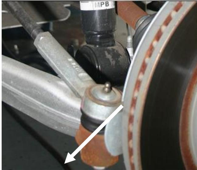
9. Using the **21mm** socket or wrench, remove the nut on the end of the tie-rod and then move the steering are out of the way. This will make the removal of the stock strut and installation of the new Racerunner shock easier.
