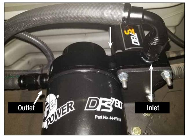
**Step 13:** Attach the fittings to the inlet & outlet ports of the fuel manifold assembly. Make sure all connections are tight.
