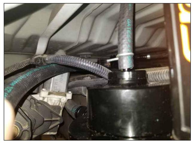
**Step 15:** Carefully route the ¼" hose to the fitting on the top of the fuel manifold assembly, making sure not to kink the hose or allow it near moving parts. Carefully mark and then cut the hose to the correct length. Using the supplied spring clamp, attach the hose to the nipple on the top of the air chamber on the fuel manifold assembly.
