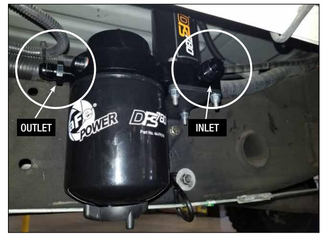
Step 1: Mount the supplied fuel manifold assembly to the supplied carbon steel frame bracket using the supplied hardware and tighten:
