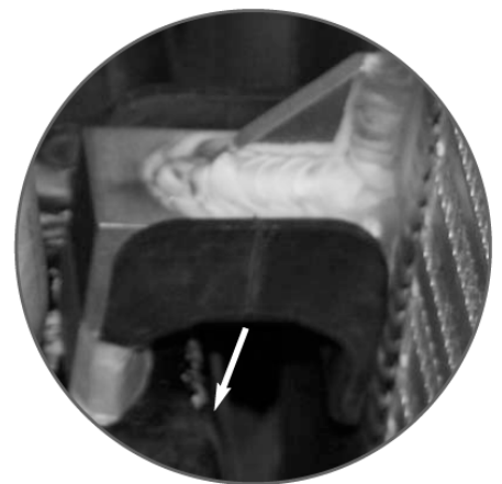
Position and make sure intercooler rubber U-shaped isolators sit square on cross beam and have not folded during installation.
