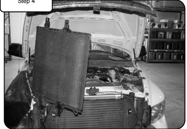
With A/C condenser turned 90 degrees, secure to the vehicles lifted hood using steel wire.
