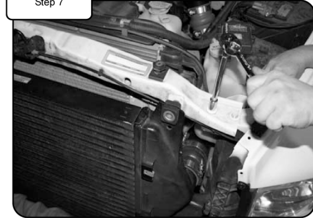
Loosen and remove the 4 bolts holding in upper radiator support using 13mm socket or wrench.
