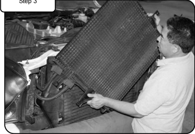
Rotate the A/C condenser up and out away from vehicle. Take care to prevent damage to A/C lines.
