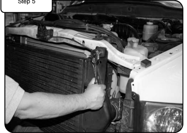
With 10mm socket or wrench remove the 2 top intercooler attachment bolts connected to upper radiator support.
