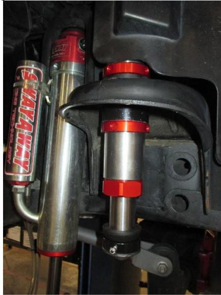
*\*\*Check to see that both rings are fully engaged to the frame, if they do not sit correctly, remove the bumpstop and use the grinder to remove any sections that are causing the lock rings to sit flush in the hole.*
