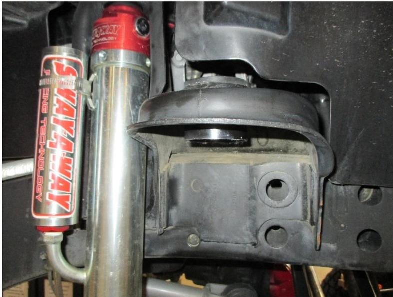
13. Remove upper lock ring from the bumpstop, slide it up from the bottom and re-install lock ring with the included spanner so that it is tight in the existing hole.
