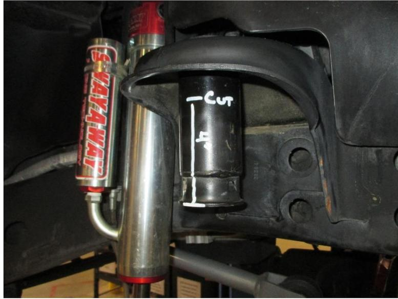
12. Carefully cut off the tube, be sure to cut as level as possible, as the bumpstop will need a straight surface to mount correctly.
