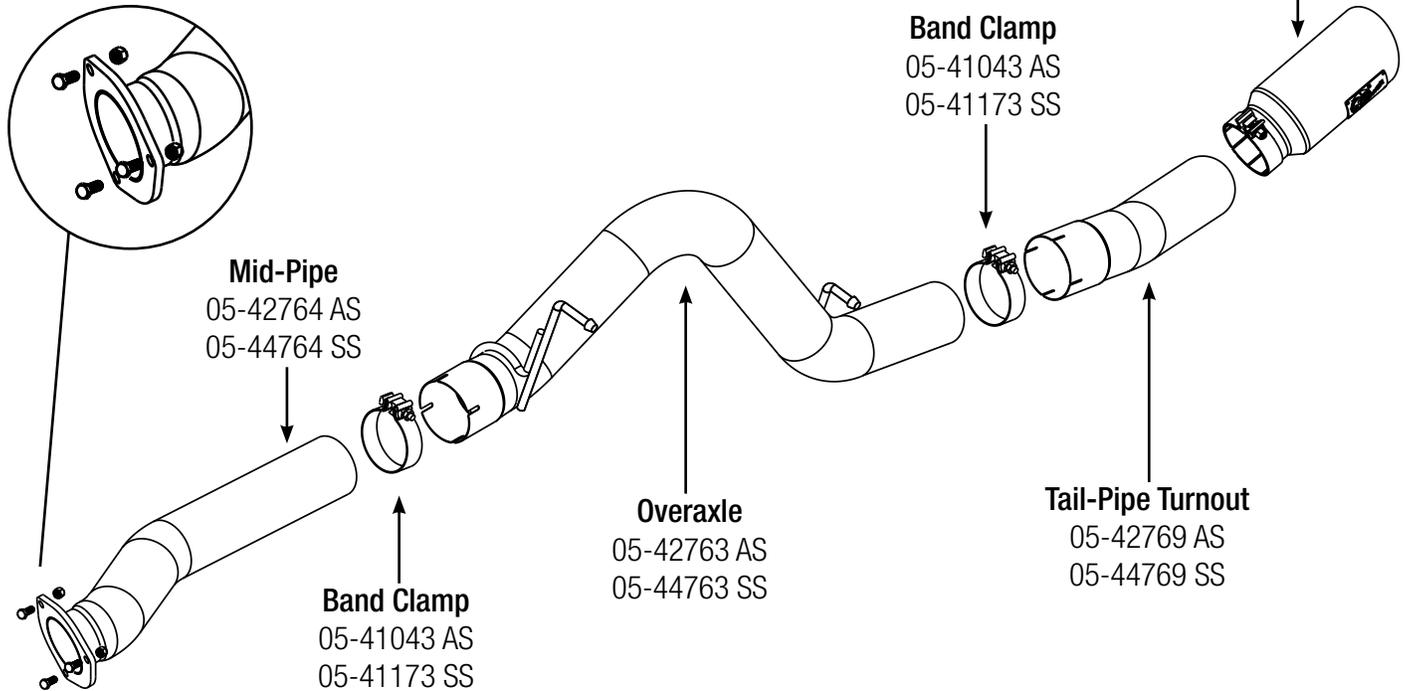
**Step 1: (Read Instructions prior to installation)** Loosen mounting flange at rear of particulate filter before muffler. Remove the stock exhaust from the rear of the truck working your way forward. Take caution not to damage the factory isolation mounts and gasket as they will be reused. **It is recommended to not fully tighten the clamps until the entire system has been installed.**
