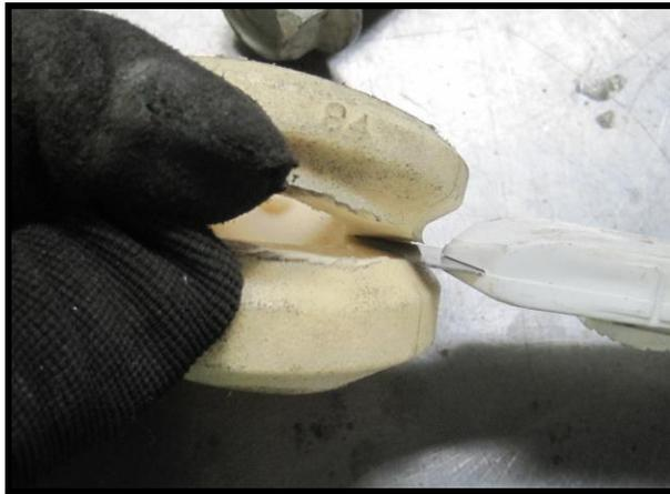
**Figure 7- Trimming Front Bump Stop**
