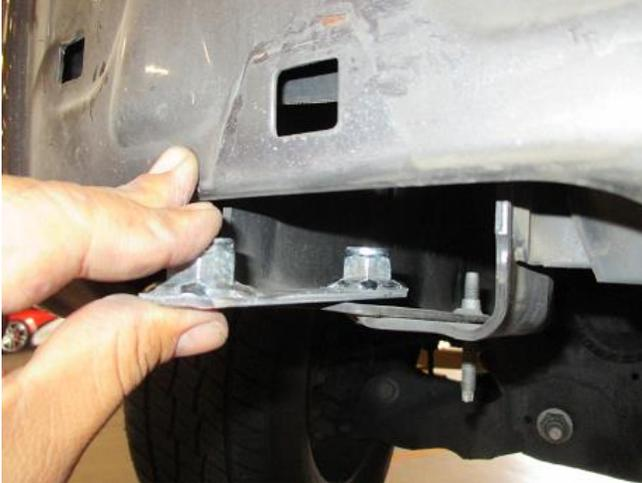
21. Install the reservoir mount with the supplied bolts to the frame with the bracket facing downwards. Use the stock stud for the rear mounting hole on the bracket and the backing plate for the front mounting hole.
