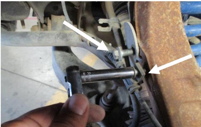
10. Follow the ABS sensor wire to the back of the wheel well, disconnect the plug, remove the wire from the clip on the upper arm, and let the wire hang free.
