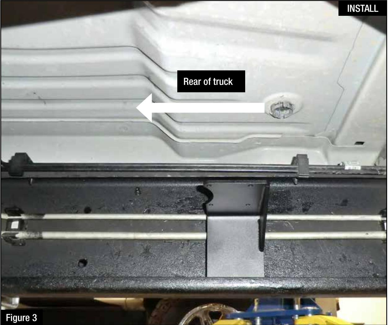
**NOTE: This is what the bracket looks like when installed correctly.**
