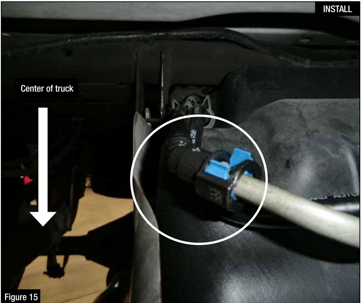
Step 16: Locate the factory fuel return line. It is located at the front of the fuel tank near the center of the truck.
