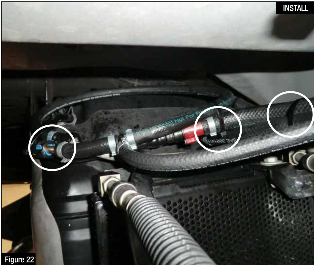
Step 23: Using the supplied nylon cable ties, secure the new hoses (as shown above).
