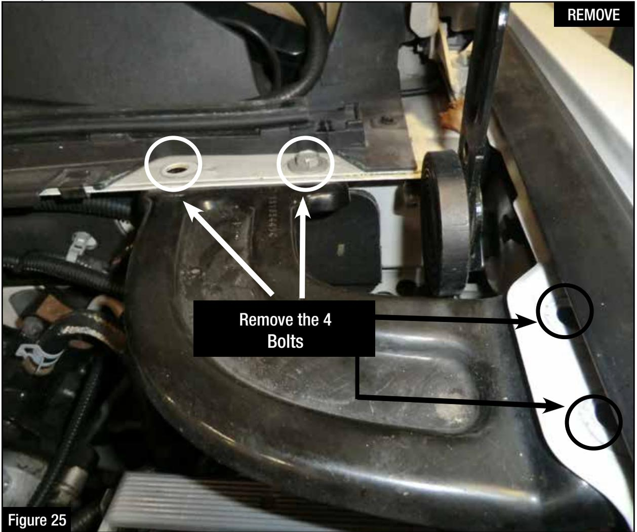
Step 28: Remove the four (4) bolts holding the corner brace in the engine compartment. Remove the brace and hardware and retain for re-installation.
