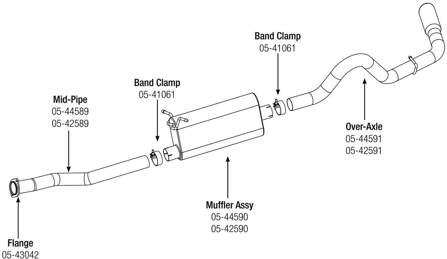
**Step 1: (Read Instructions prior to installation)** Remove your stock exhaust from the rear of your truck working your way forward. Take caution not to damage the factory isolation mounts as they will be reused. It may be helpful to lubricate the isolation mounts prior to disassembly. **It is recommended to not fully tighten the clamps until the entire system has been installed.**
