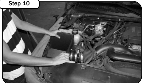
Step 10 Place the rubber trim seal along edges of the housing. Bolt the housing to the engine bay using the factor bolts removed in Step 6. If installing stage 1 kit re-connect factory tube to MAF sensor.
