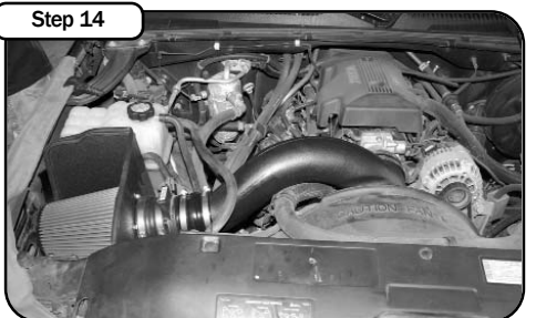
Step 14 Place enclosed CARB EO sticker on a clean/smooth surface on or near the intake system. EO identification label is required in passing the Smog Check inspection. Make sure all hoses and clamps are tight and that all electrical components are secure. Reconnect the battery at this time.
